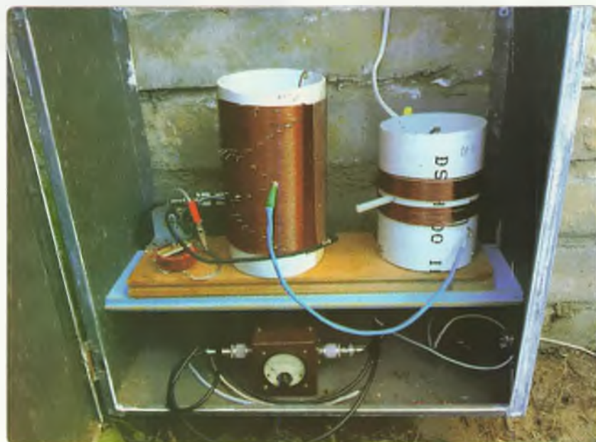
Photo 3: VK7TW's 630 metre antenna tuning unit. Photo courtesy of Justin VK7TW.
