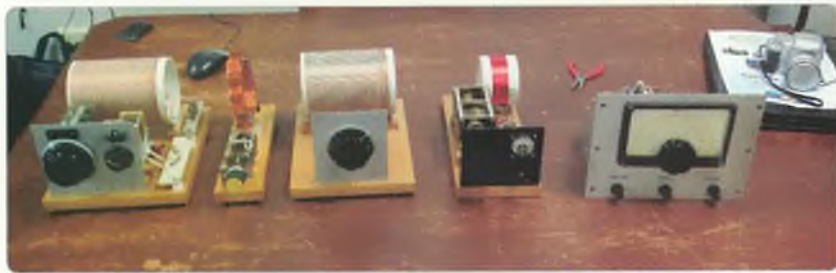
Photo 2: Examples of the homebrew crystal sets constructed by GARC members.
