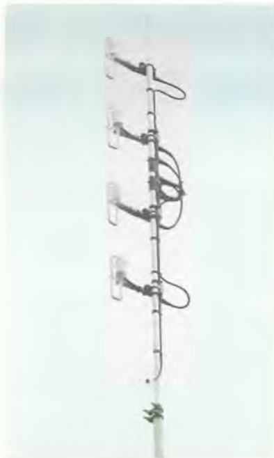
Photo 6: The completed vertical array.
