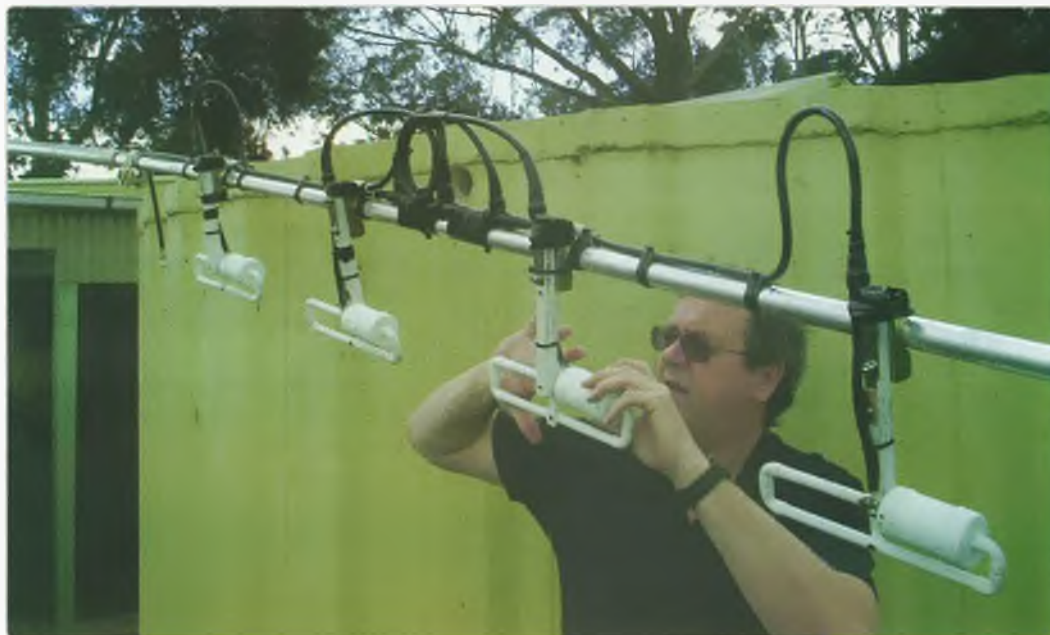
Photo 5: Rob VK3BRS waterproofing the tuned antennas.
