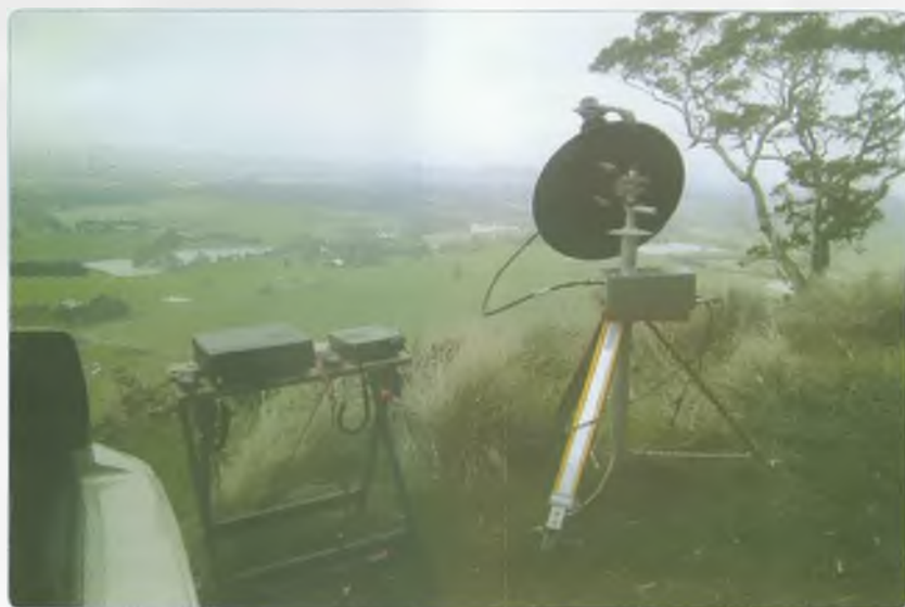
Photo 2: Ian VK3AXH's 3.4 GHz system on location at Mt Buninyong.
