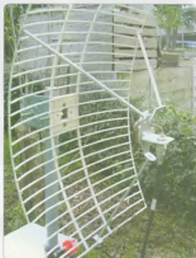
Photo 1: Rob VM3MQ's gridpack with homebrew 3.4 GHz feed.
