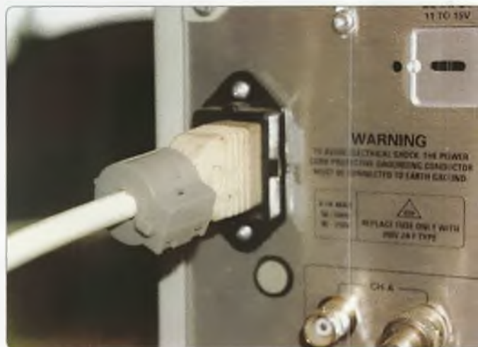
Photo 5: Mount ferrite as close to equipment as possible.
