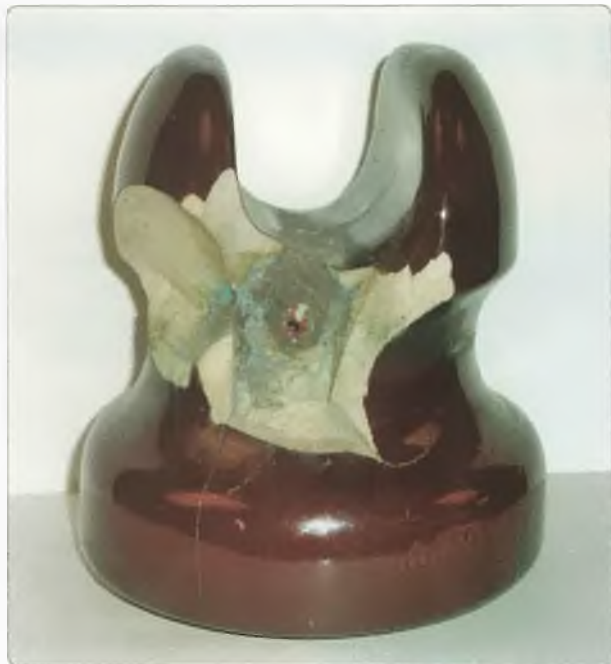
Photo 3: Lightning damaged insulator.
