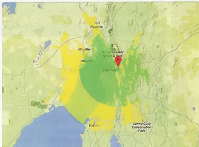
Figure 2: Predicted ATV repeater radiation pattern.
