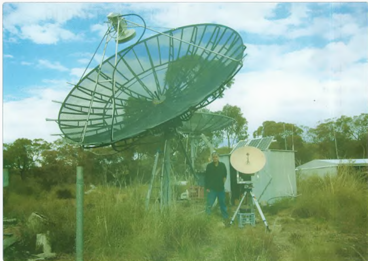
Photo 1: Rex VK7MO with his 10 GHz 77 cm dish alongside Dave VK2JDS's five metre 1296 MHz system.
