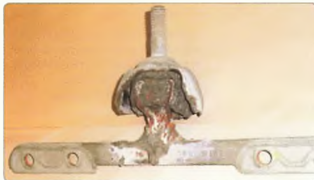
Photo 7: Pole hardware damaged by lightning.
