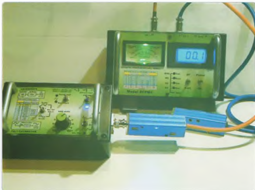
Photo 3: The RFPM1 power meter together with the VK3AQZ homebrew calibrator.
