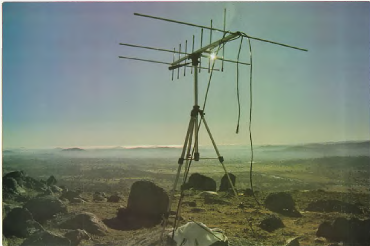
Photo 1: The dual band Yagi ready to be connected, looking out from Castle Hill, VK1/AC-032.
