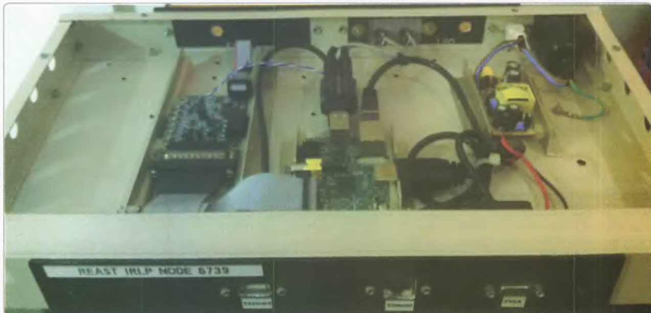
Photo 2: REAST IRLP node 6739 using RaspberryPi single board computer. Photo courtesy of Justin VK7TW.
