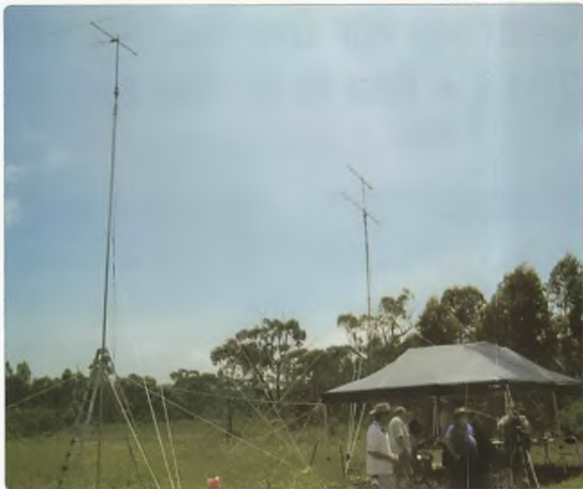
Photo 2: The Blue Mountains ARC seems to have field day antenna erection down to a fine art – 6 m on the left hand mast, 2 m and 70 cm on the right hand mast.
