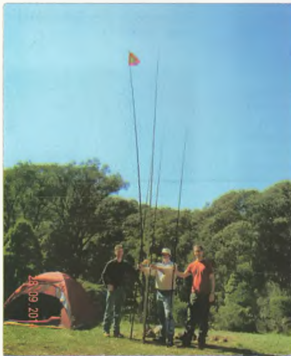
Photo 4: L to R: a 7 m heavy duty squid pole, 10 m squid pole, 4.1m mini-pole and 2 x 5 m light duty squid poles.
