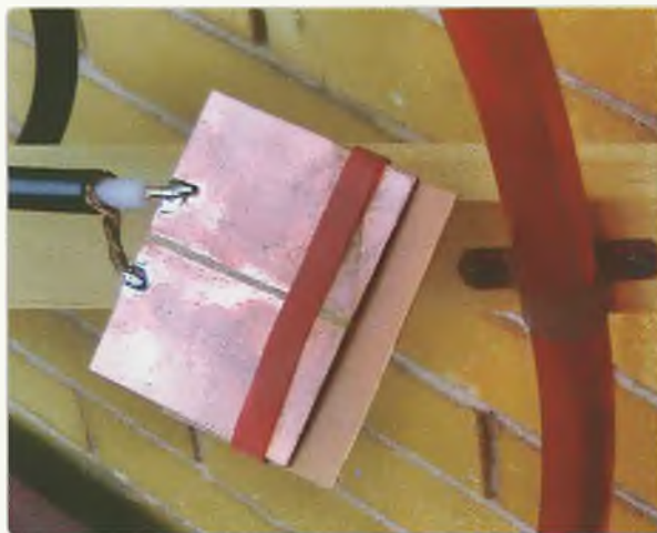
Photo 5: Printed circuit board capacitor for fine frequency adjustment.
