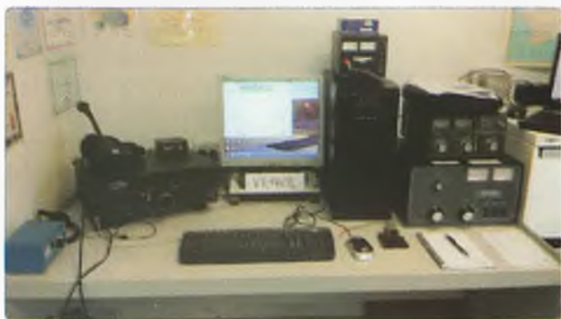
Photo 4: VK4WIL 14 and 3.5 MHz position. The big black box contains switchable coax stubs for 160 - 10 m.
