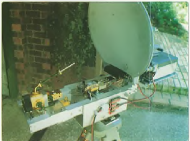
One of the 76 GHz transverter units used in the VK4 record contact.
