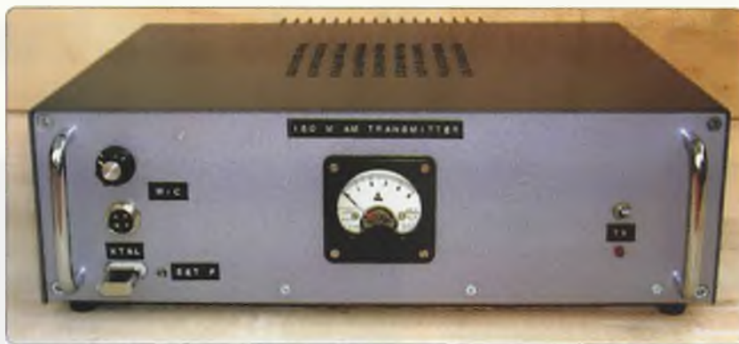
Photo 1: The 100 W class-D AM transmitter for 1.8 MHz.
