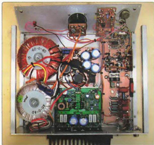
Photo 2: Inside the case of the 100 W 1.8 MHz AM transmitter.
