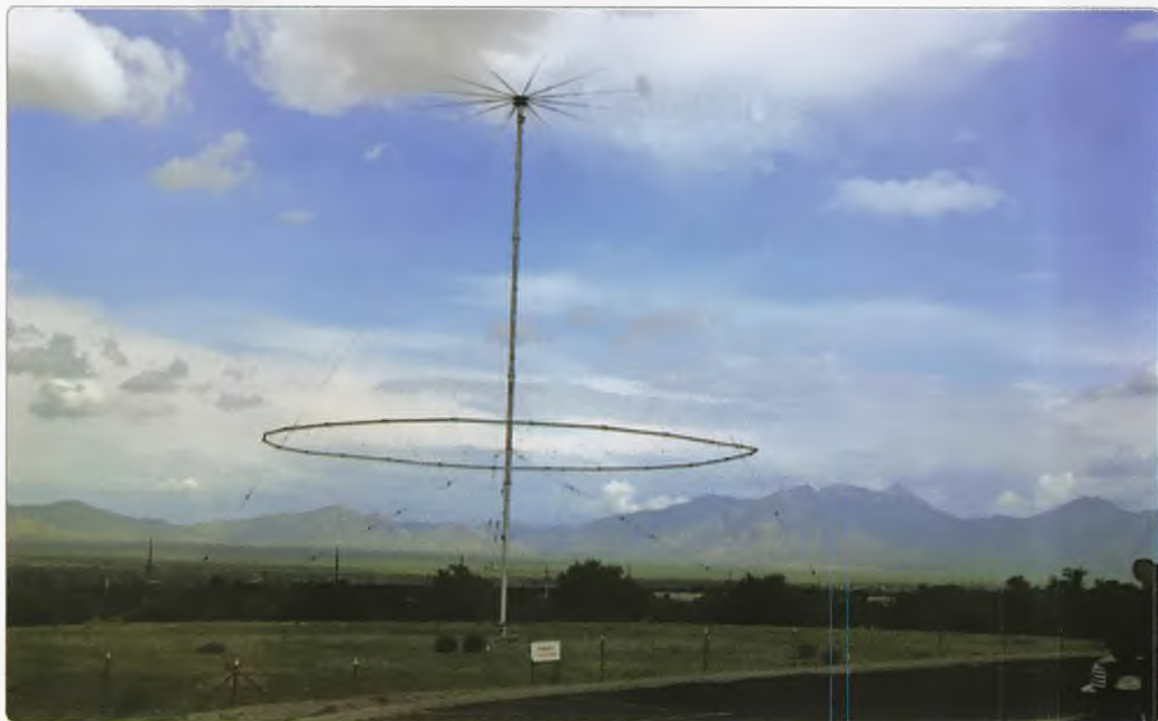
Photo 1: The Titan discone antenna itself – imposing, to say the least.
