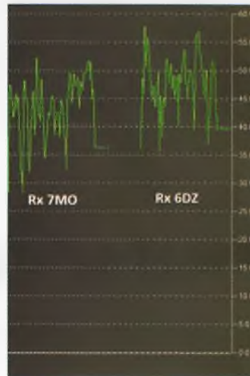
Figure 11: Comparison of S/N on best single tone signals (time for each section of signal around 20 seconds, vertical scale from 0 to 50 dB).
