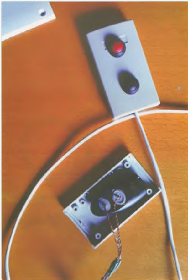
Photo 2: The remote affected by pulsing from the small weather station.
