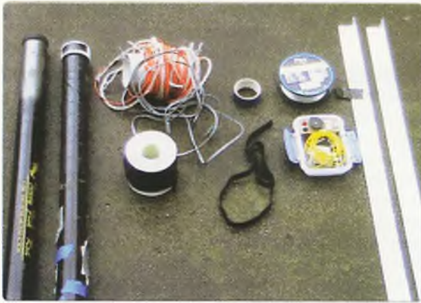
Photo 1: Typical items needed – 2 x squid poles, sand stakes, wire, Velcro straps, coupler, fishing line, insulation tape.
