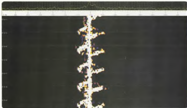
Figure 2: Spreading due to wind-generator some 3.5 km away over a 1040 km 10 GHz path from VK7MO to VK5KK. Note that the pattern repeats around every 1.3 seconds consistent with the speed of the wind-generator.
