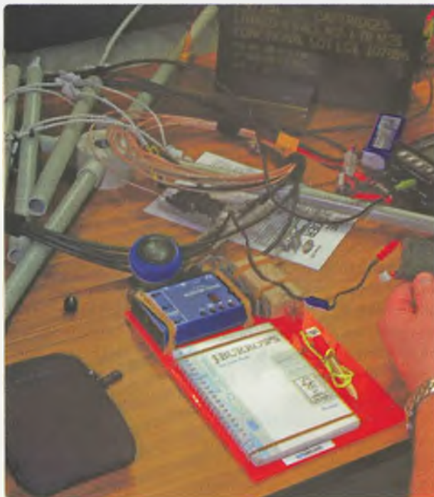
Photo 2: Shown is a SOTA Flight Deck. It holds a MTR CW three band transceiver, the paddle keyer, logbook and pencil. Operation is easier with everything held in place by rubber bands.
