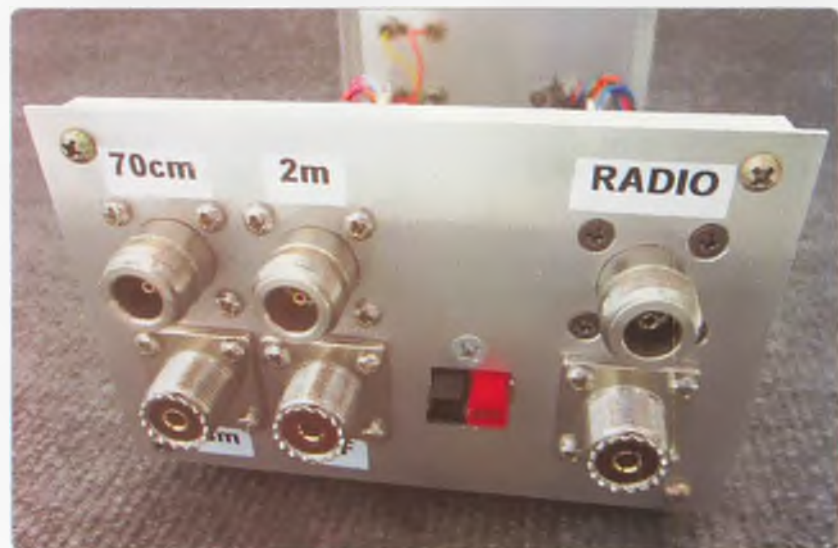
Photo 1: The RF end of the completed breakout adapter.
