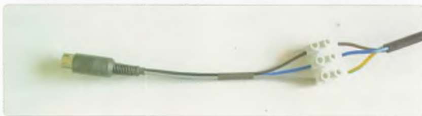
Photo 6: Terminal block to 5 pin DIN connector.
