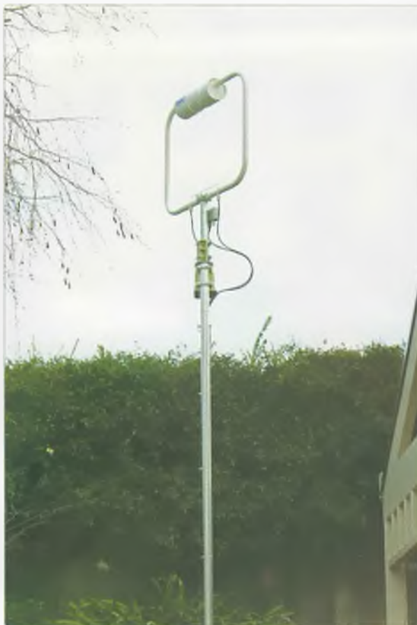
Photo 5: The loop mounted on a mast.
