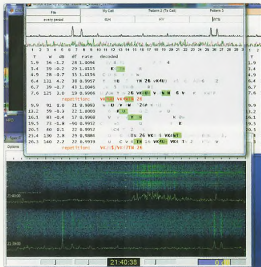
Figure 3: 50 MHz FSK441 signals received at VK4UH from VK4WTN 21.4.15. Lower period showing Meteor Backscatter pings and corresponding MSRX decodes. Upper period showing classical patterns of Aircraft Backscatter – all undecodable. Both periods superimposed on weak direct signals off the back of the beam.
