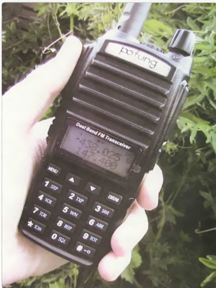
Photo 1: The real cost of amateur radio transceivers has fallen by 70 to 90% in recent decades. This is a 50 dollar dual band 2 m/70 cm FM handheld.
