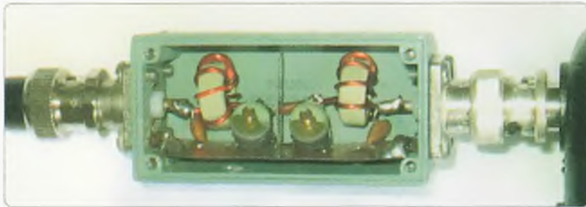
Figure 4: The low-pass filter which fits conveniently between the whip antenna and connector.
