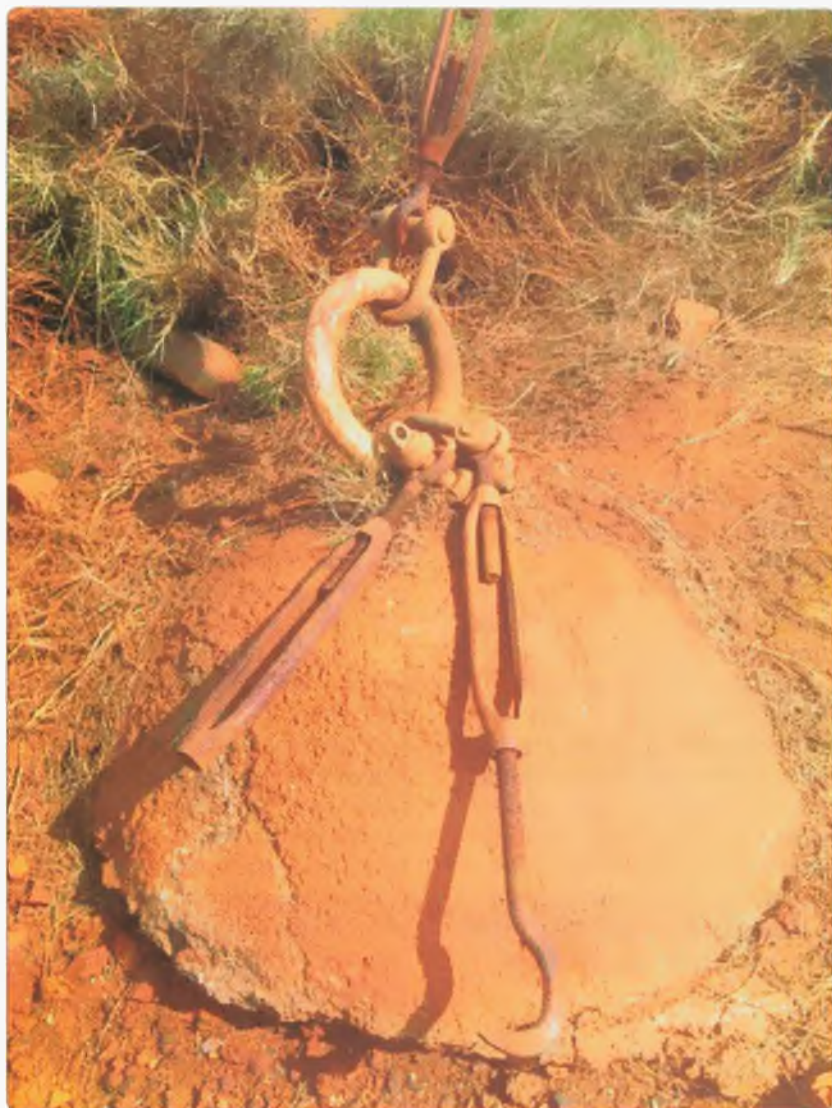
Photo 3: The damaged turnbuckles.
