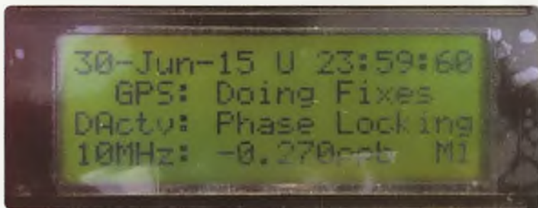
Photo 2: 2015 Leap Second captured by the author on his GPS Disciplined Oscillator. Photo courtesy of Justin VK7TW.
