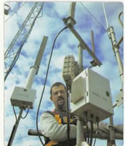
Photo 2: Damien VK5FDEC with the 3.4 and 5.7 GHz beacons. The 10 GHz unit is yet to be installed at the time of taking the photo.
