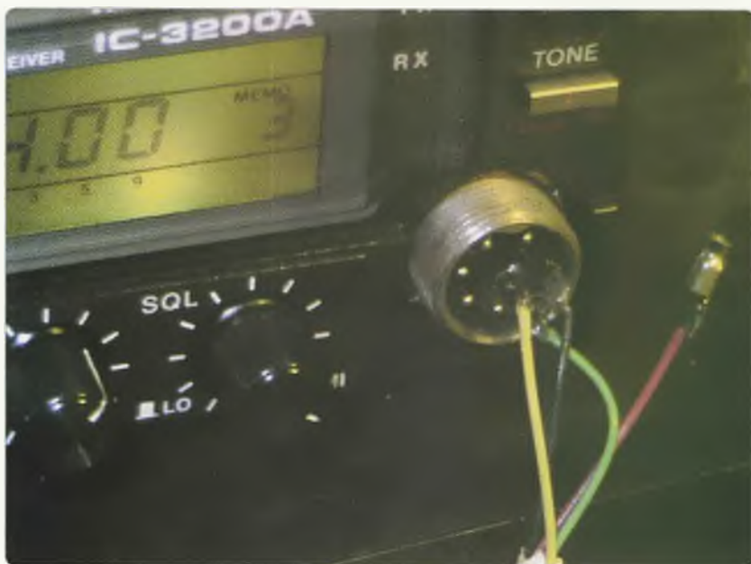
Photo 2: The base transceiver's microphone socket showing salvaged connectors from old crystal sockets.
