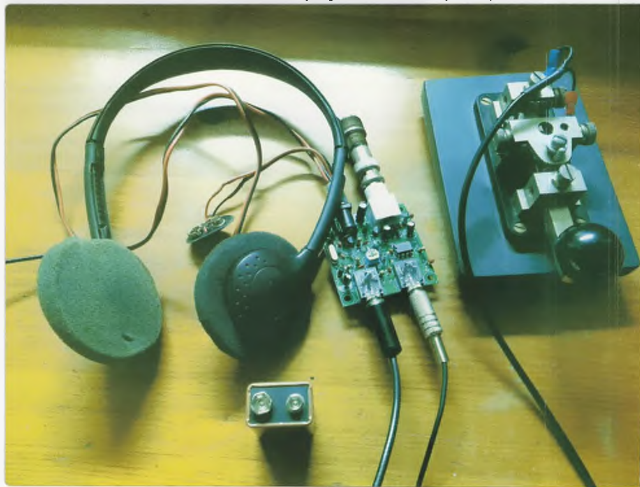
Photo 1: The Pixie transceiver and accessories almost ready to go into action. Photo by John Eyles VK2YW.
