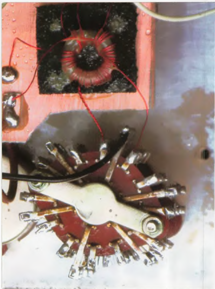
Photo 3: Close up of coil and band switch.
