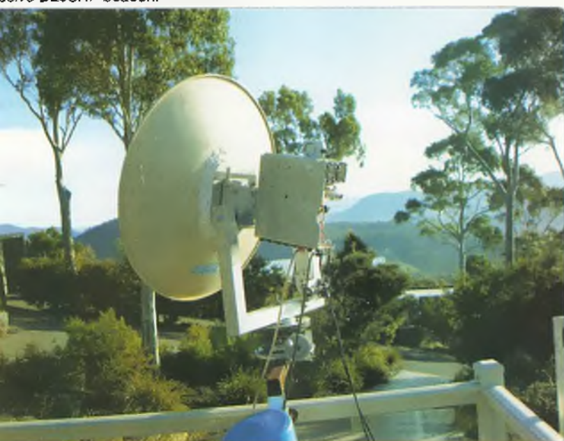
Photo 2: VK7MO's 77 cm dish and system rotated to Vertical Polarization to receive DL0SHF beacon.
