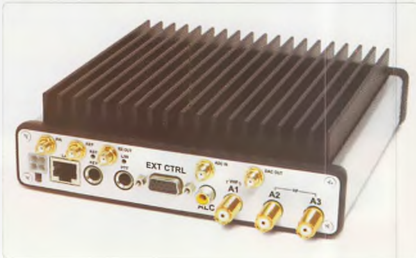
Photo 2: The transceiver rear panel layout.
