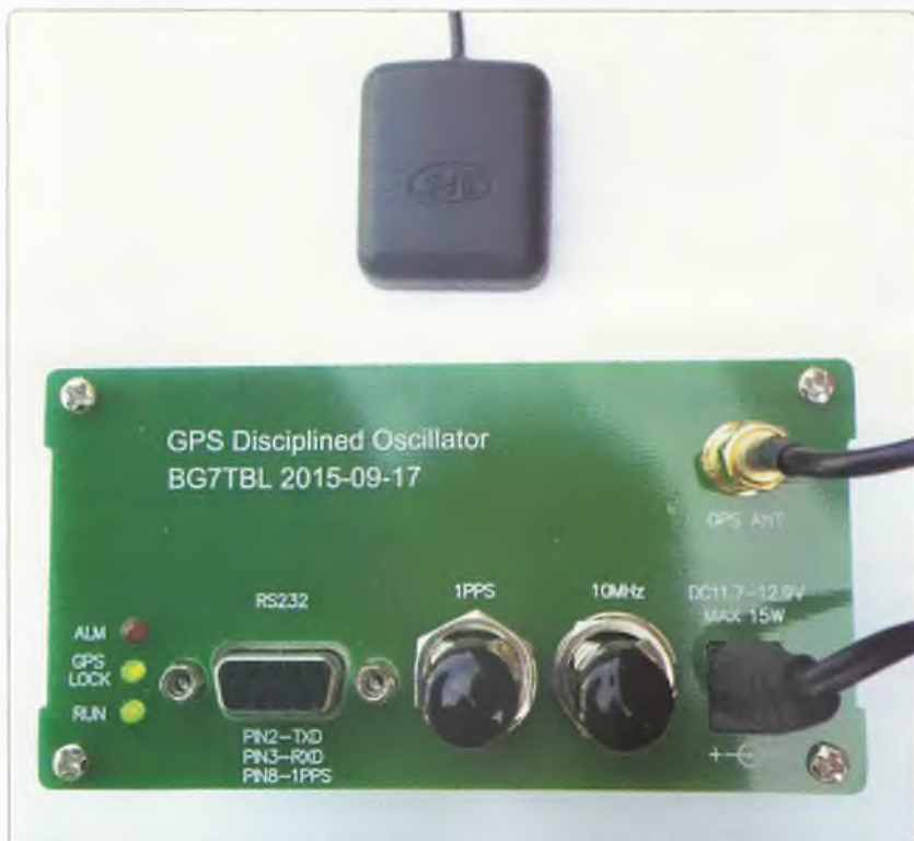
Photo 3: Chinese GPS Disciplined Oscillator Unit for narrow band weak signal work. (Photo courtesy of Justin VK7TW.)
