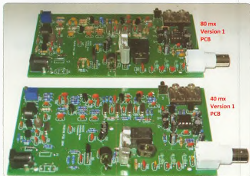
Photo 1: The 80 m and 40 m units built on the version 1 pcb.
