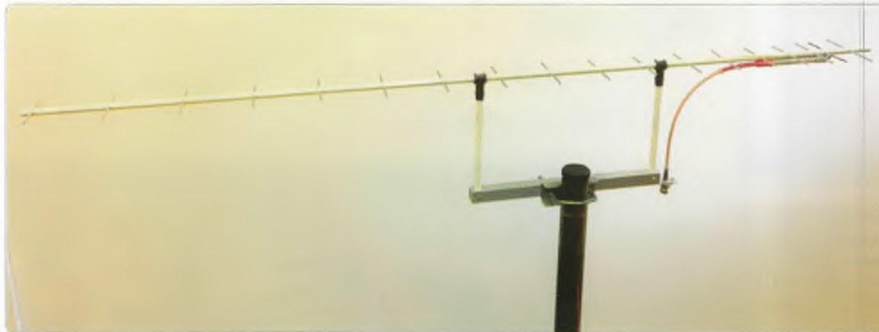
Photo 3: Completed and tuned 23 cm Yagi. (Photo courtesy of Justin VK7TW.)
