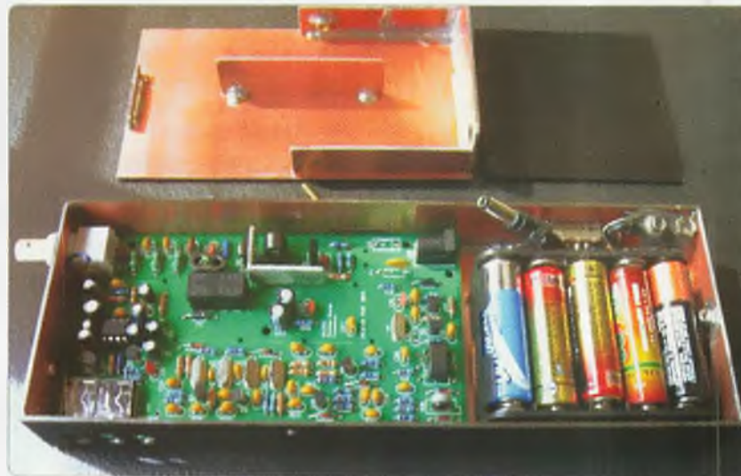
Photo 5: The built 20 m unit in the pcb case.
