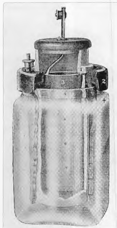
Figure 4: Cutaway drawing of a 60 Ah production model cell.
