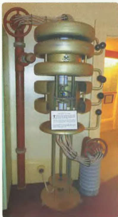
Photo 8: Antenna Tuner switching relay.
