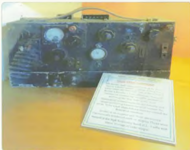
Photo 9: Converted WW2 WS101 used by fishermen. Capable of around 10 W AM from 2 to 6 MHz. Made for the Australian Army by AWA. Tuning dial obscured by reflection in the glass.
