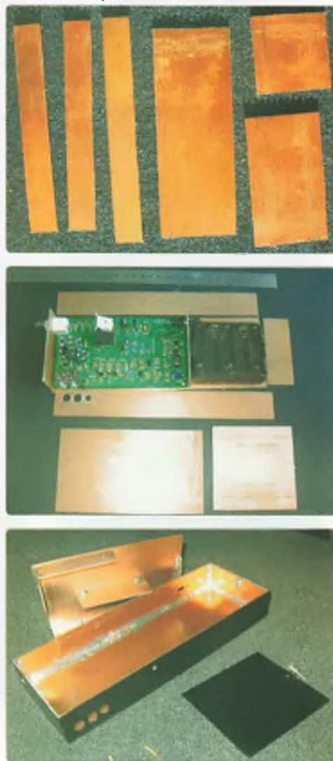
Photo 2: The pcb case under construction.
