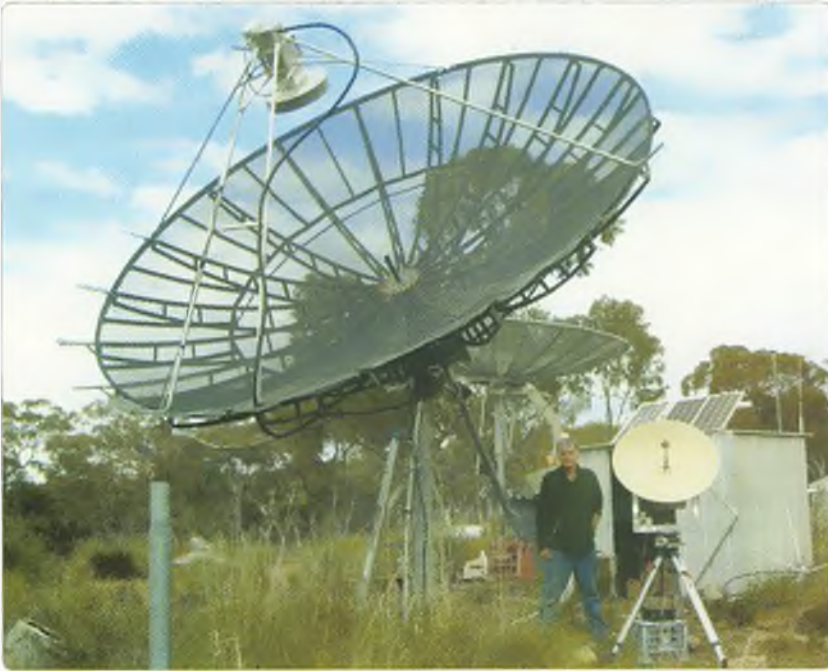
Rex Moncur VK7MO with his 77 cm 10 GHz dish, dwarfed by the 5 m 1296 MHz system of David Scott VK2JDS (QF46PV, near Bathurst, NSW).
