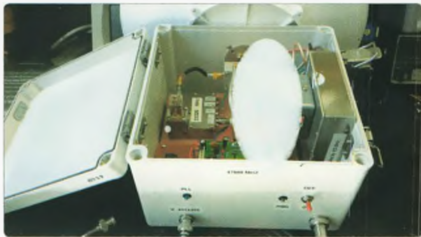
Photo 1: Simon VK5TE's upgraded 47 GHz transverter with Nurad antenna.
