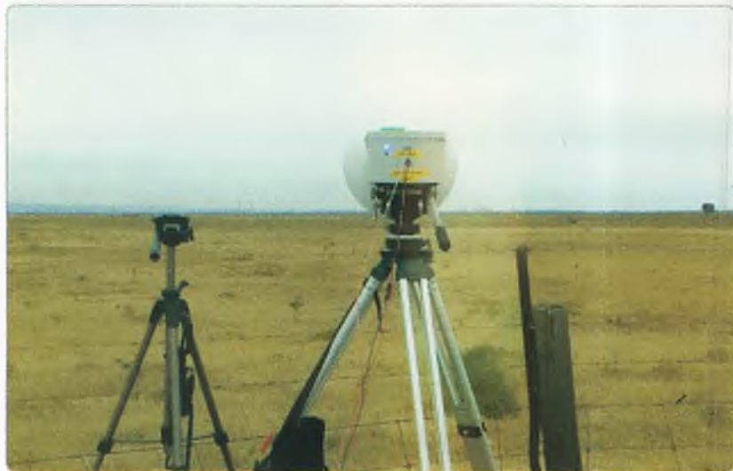
Photo 2: 47 GHz 30 mW system and horizon view at the VK5KK end.
