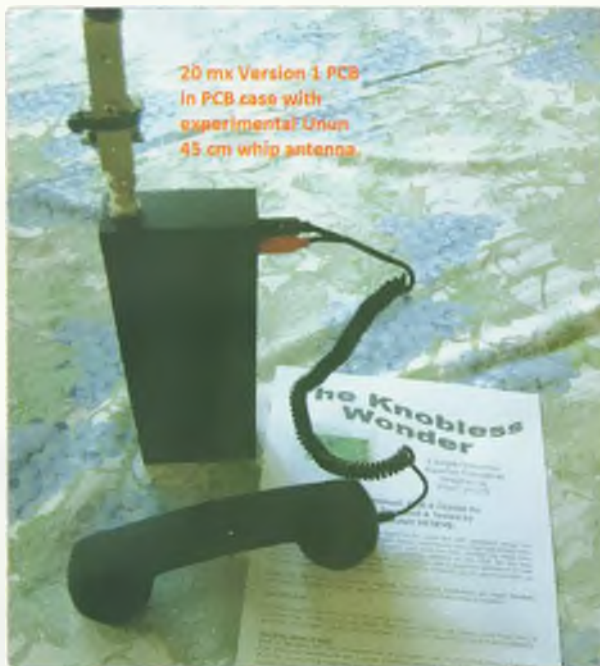
Photo 6: The 20 m complete radio built as a handheld.
