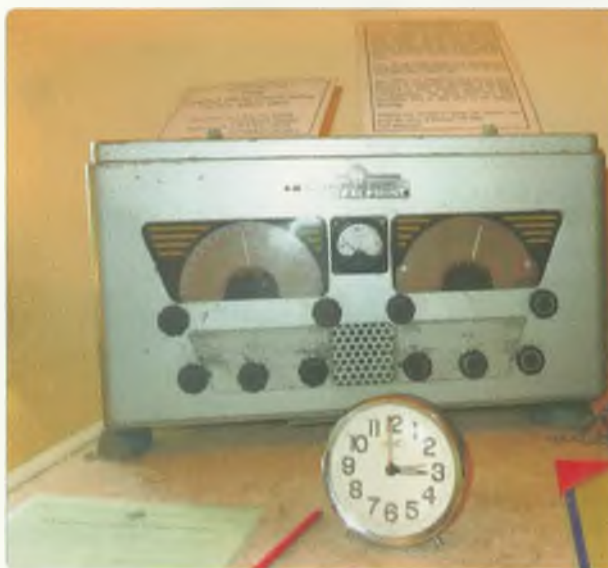
Photo 10: AWA Marine transceiver that replaced the WW2 surplus equipment.
