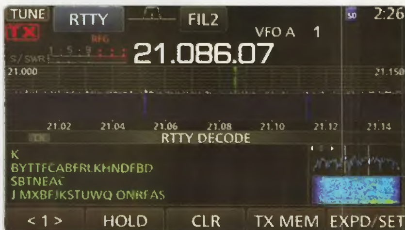
Photo 5: In-built RTTY decoding in action, showing the decoded text and waterfall display.
