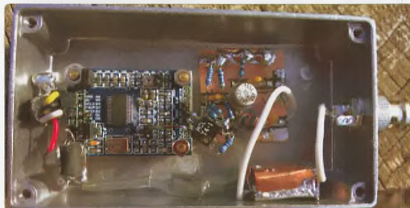
Figure 15: AD9851 Module with Transformer & classic 2N5109 Broadband Amplifier.
