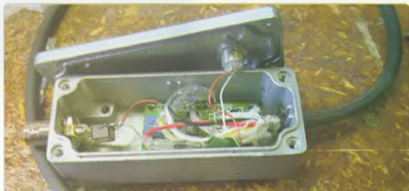
Figure 13: AD9850 module with series diodes in supply.
