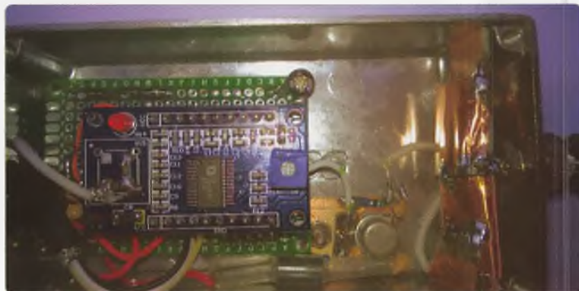
Figure 14: AD9850 Module in box, note Oscillator on board under module.
