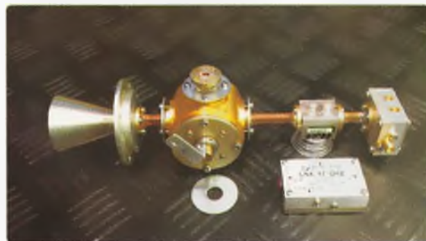
Photo 3: Mudguard washer flange adapters on a 47 GHz transfer switch.
