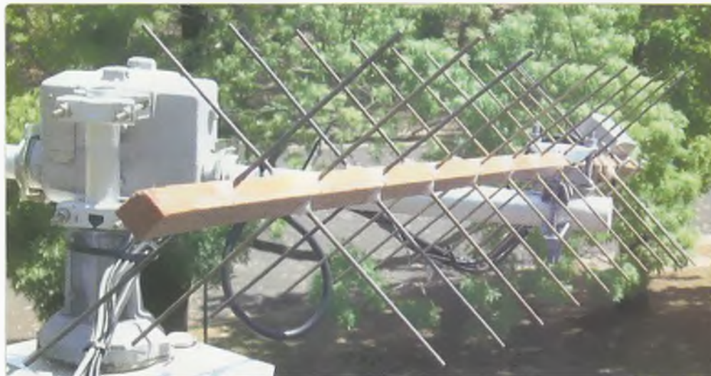
Photo 1: Photograph of the completed antenna looking down the boom towards the LNA box at the far end.
