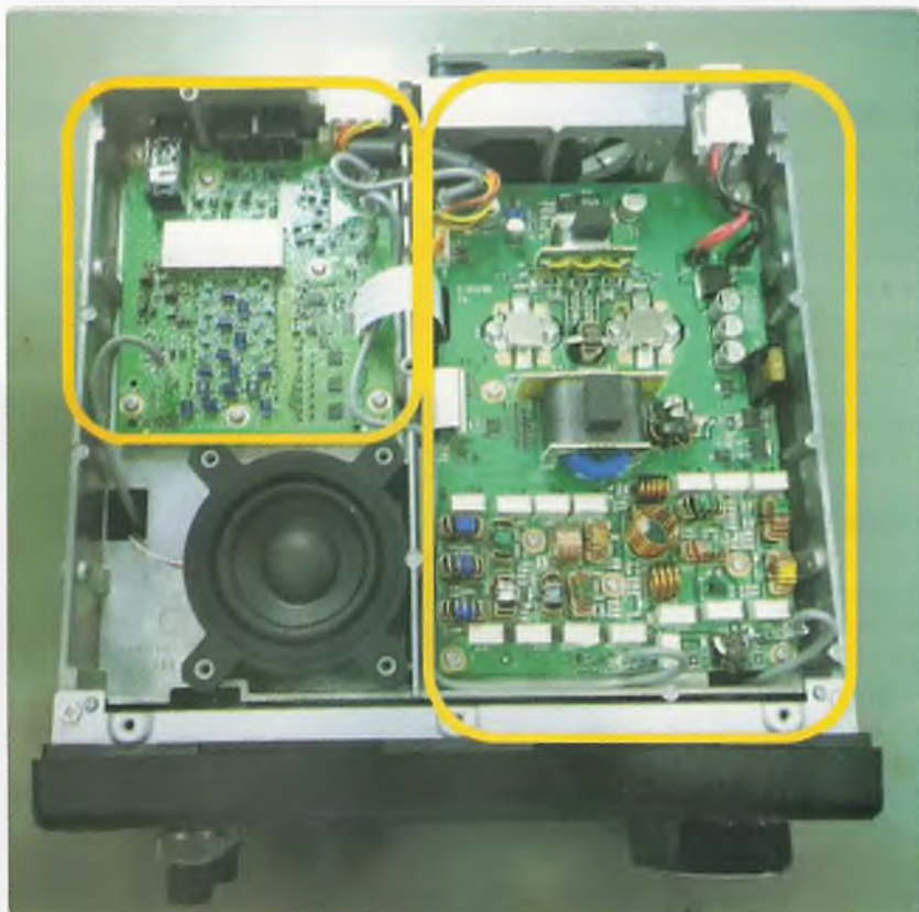
Photo 3: Undemeath the top cover. Highlighted on the left is the RF unit, with the PA unit on the right. Bottom left is the speaker, located in its own compartment.
