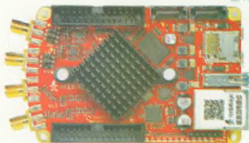
Photo 5: Red Pitaya Open Source Analysis Board. (Photo courtesy of Elektor Online).
