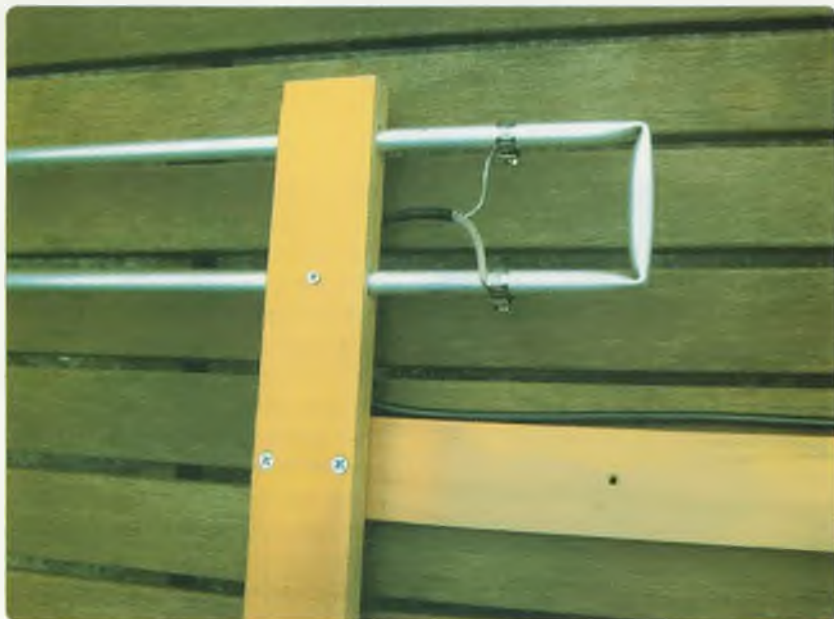
Photo 3: Close up of the antenna feedpoint and mounting method.
