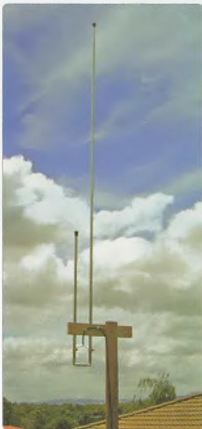
Photo 1: The completed J-pole antenna.
