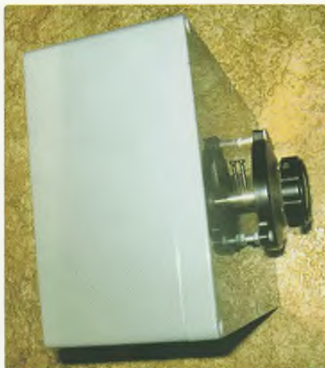
Photo 3: My project box showing grub screw.
