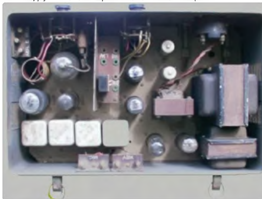
Photo 3: 3B Transmitter: the interior of this model, which has an in-built 240 V Power Supply. The 807 and output coil can be seen at the top left.
