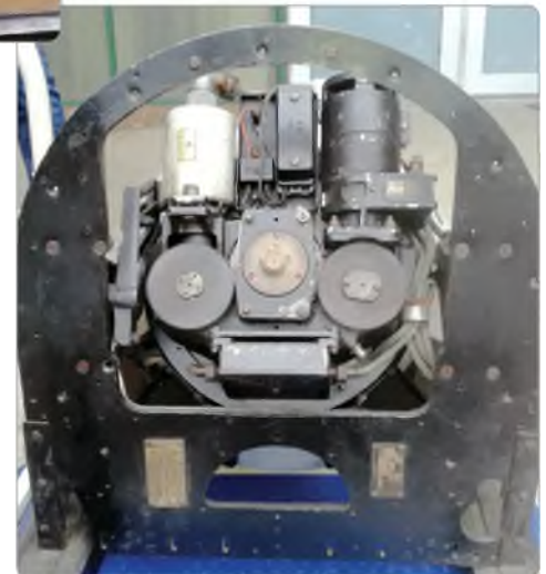
Photo 3: The drive motors and gearing for the rotating feed can be seen. The microwave and other electronic equipment were separate.
