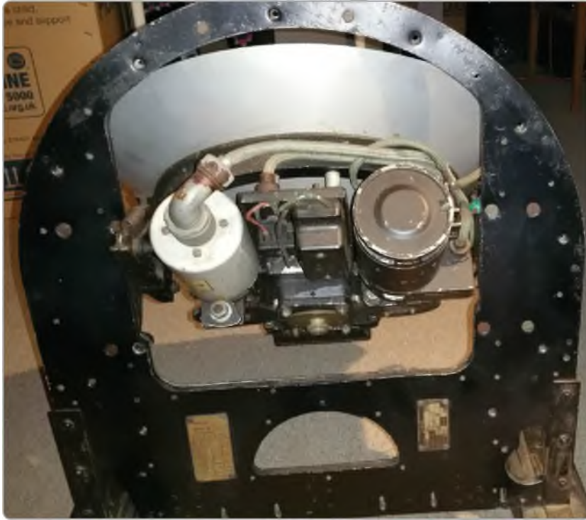
Photo 6: Another view of the hardware for driving the feed and thereby rotating the lobe of the radar to scan the sky.
