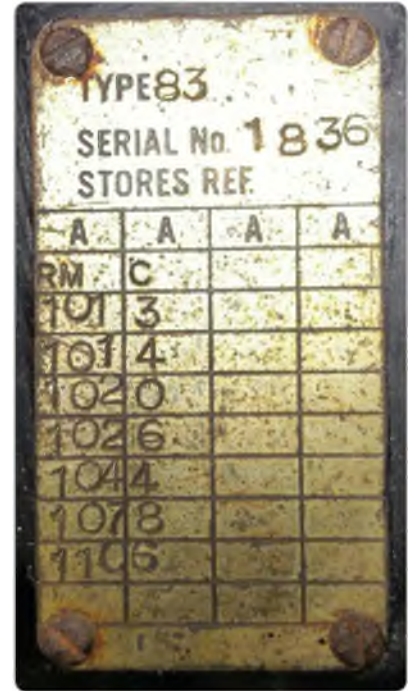
Photo 7: The name plate/modification record. The stampings here are clear. It appears to record the various modifications incorporated in this unit.
