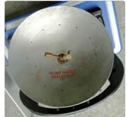
Photo 2: The feed, counterweight and reflector.
