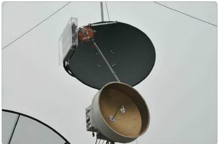
Photo 7: Close up of triband feed 3/5/10 GHz dish and 24 GHz dish.
