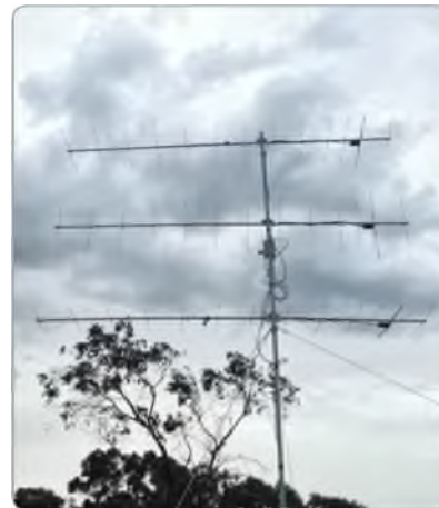
Photo 3: 2 m antennas: 13 element horizontal stack for SSB, 13 element vertical beam for FM mounted on 6 metres rotatable pole.
