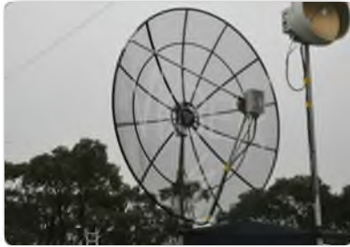
Photo 5: Close up of dual feed 1.2/2.4 GHz dish with masthead preamps, 24 GHz in foreground.
