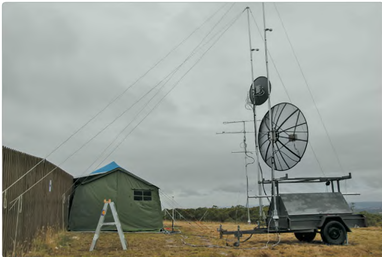
The multi-operator VK3KQ station deploys rigs for all bands from 50 MHz through 10 GHz.
