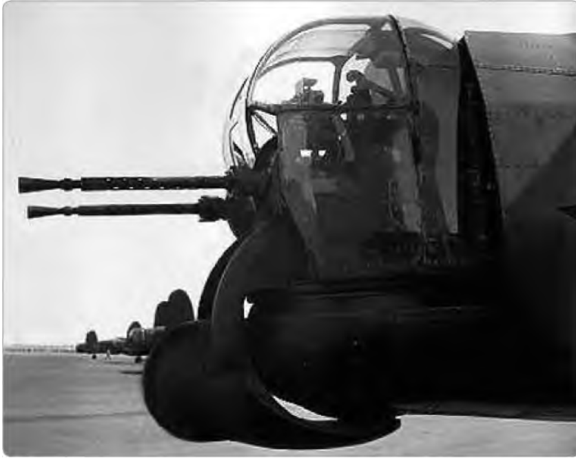
Photo 4: Village Inn installed on an Avro Lincoln. The gunner was located in the main cabin. There wasn't room for him in the turret anymore, anyway. The Australian built versions did not have the radome assembly hanging on the gun turret but appear to have a smaller fixed radome presumably to house an updated Village Inn system.
