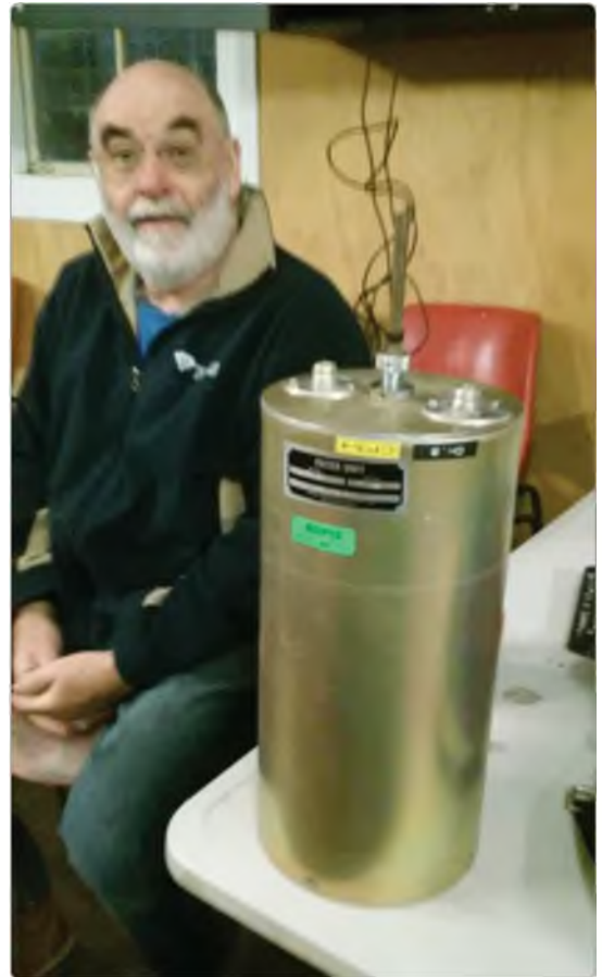
Photo 4: Bob VK4BXI with the newly commissioned 2 metre cavities for our repeater.
