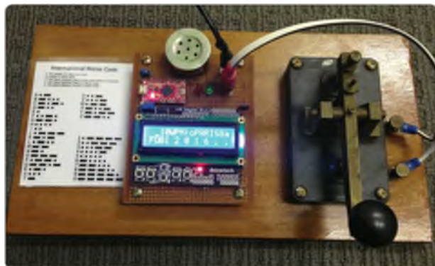
Photo 3: Arduino Morse code decoders. (Photo courtesy of Justin VK7TW.)
