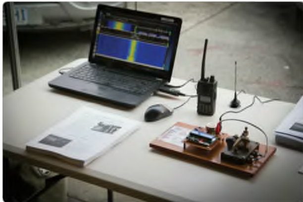
Photo 8: RTL SDR receiver. Skywave Linux notebook with RTL DVB-T USB radio receiver using CubicSDR – this radio was tuned to Triple J – the station of the school kid's generation. (Photo courtesy of Ben VK7BEN.)
