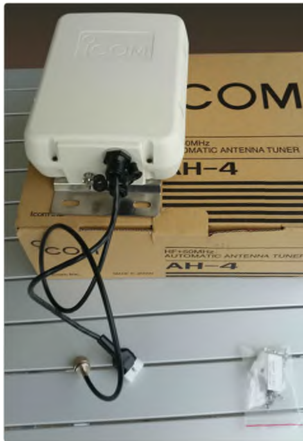
A view of an Icom AH-4 tuner, terminated with short cables to interface to an Icom transceiver.
