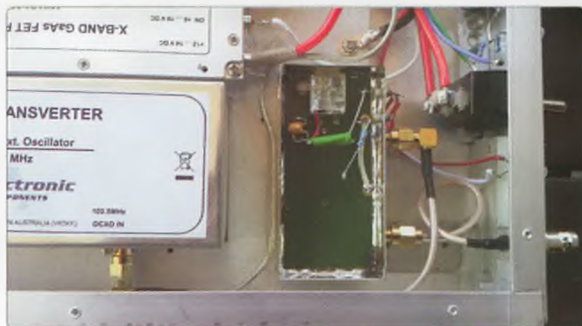
Photo 4: VK5KK's 10 GHz EME Transverter, OE2JOM PLL Source.
