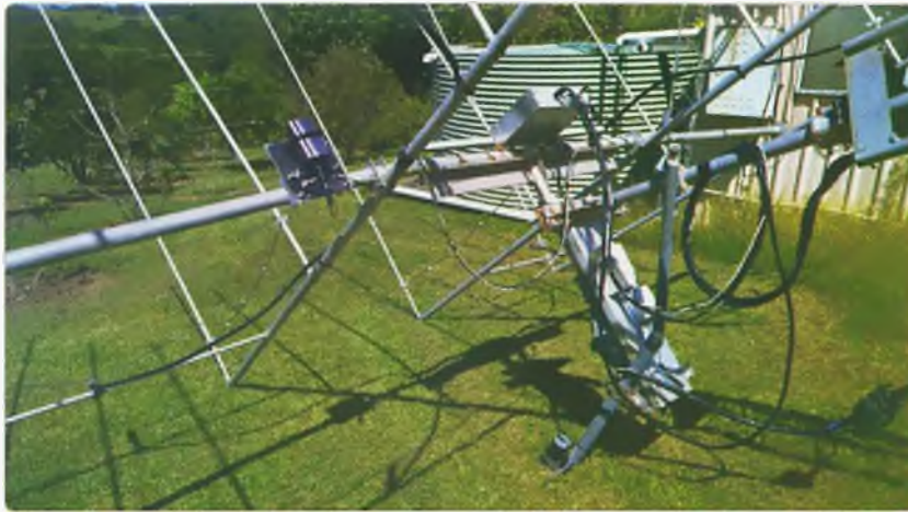
Photo 2: VK4EME's damaged elevation actuator.
