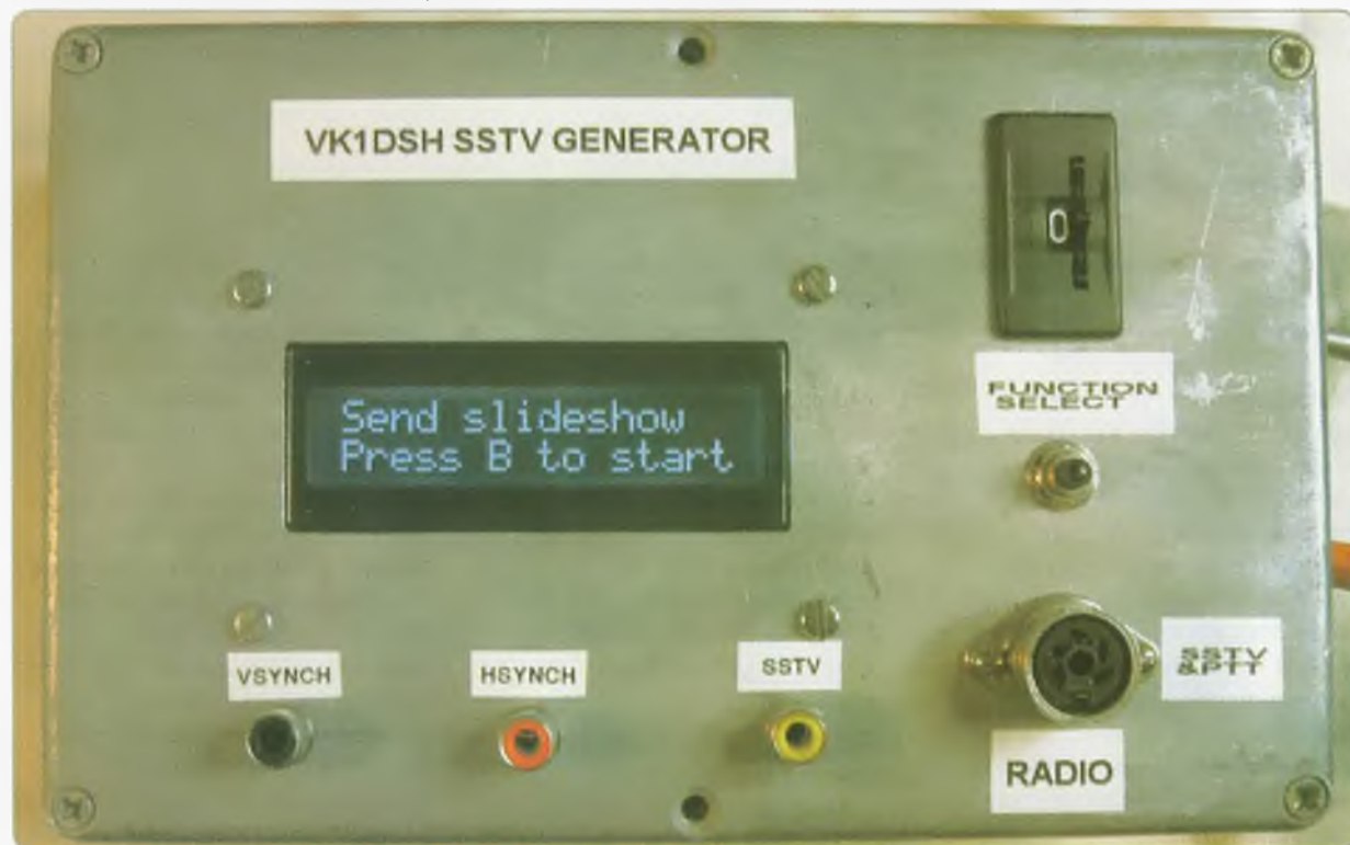
Figure 4: The completed SSTV signal source. Any suitable enclosure can be used to house the transmitter as there are no critical layout concerns for the circuitry.
