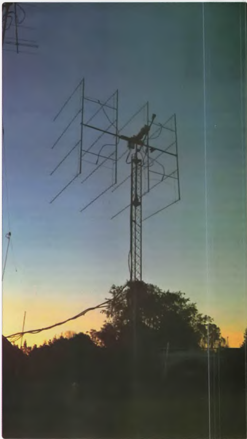
Photo 1: VK4EME's 432 MHz 240 element EME Array.
