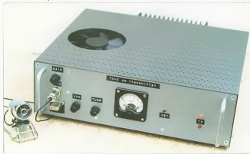
Photo 2: Front panel view of 100 W AM transmitter.
