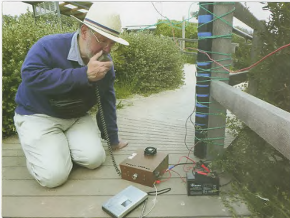
Photo 3: Chris VK3AML on 1825 kHz AM speaking far and wide with a 10 watt converted Seacom. (Photo: Stephen Langley VK3SL.)
