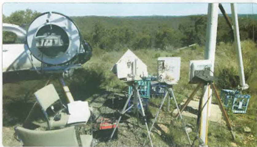
The all-bands portable station fielded by David Scott VK2JDS during the 2016 Spring Field Day, from his mountaintop at Gowan, near Bathurst (altitude 960 metres; QF46pu). Left-to-right: 24 GHz on tripod with 2 foot dish; 6 m, 2 m, 70 cm and 23 cm handhelds on the chair as well as the FT-817, connected to all the transverters by BNC cables. Log sheets on chair, too. 6 cm transverter, 3 cm transverter on top of the cyan plastic crate. 2400 MHz and 3398 MHz on the tripods. AGM battery primary power source, charged by a 2 A solar panel. The blue crates in the background have 47 GHz and 76 GHz transverters on them, run from a separate 12 V deep cycle battery. All antennas aimed at the horizon. Changing bands involves swapping connectors and moving the FT-817 and log sheets, as required. Everything is powered up all the time to keep the OXOs hot.
