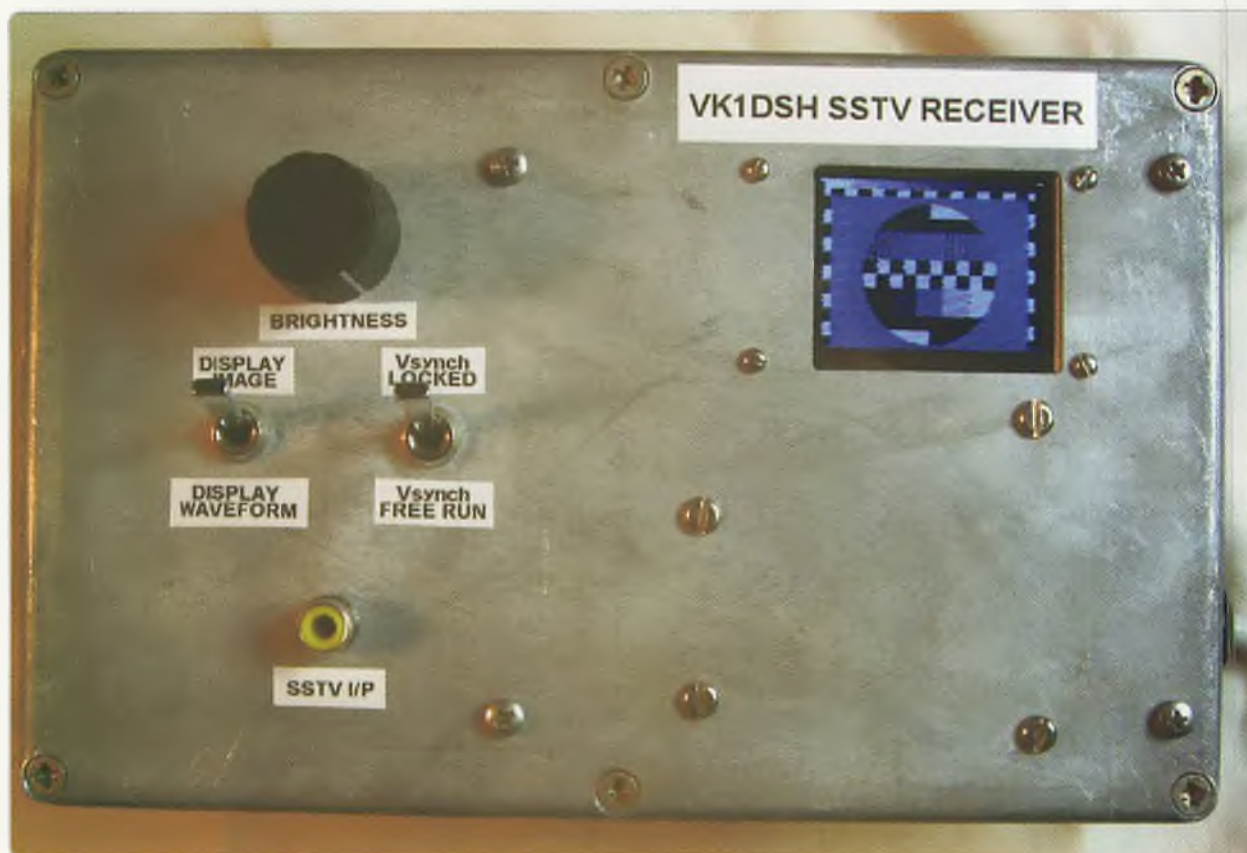
Figure 5: The complete SSTV receiver. Circuit construction is non-critical and the various items of hardware can be assembled in any suitable enclosure.
