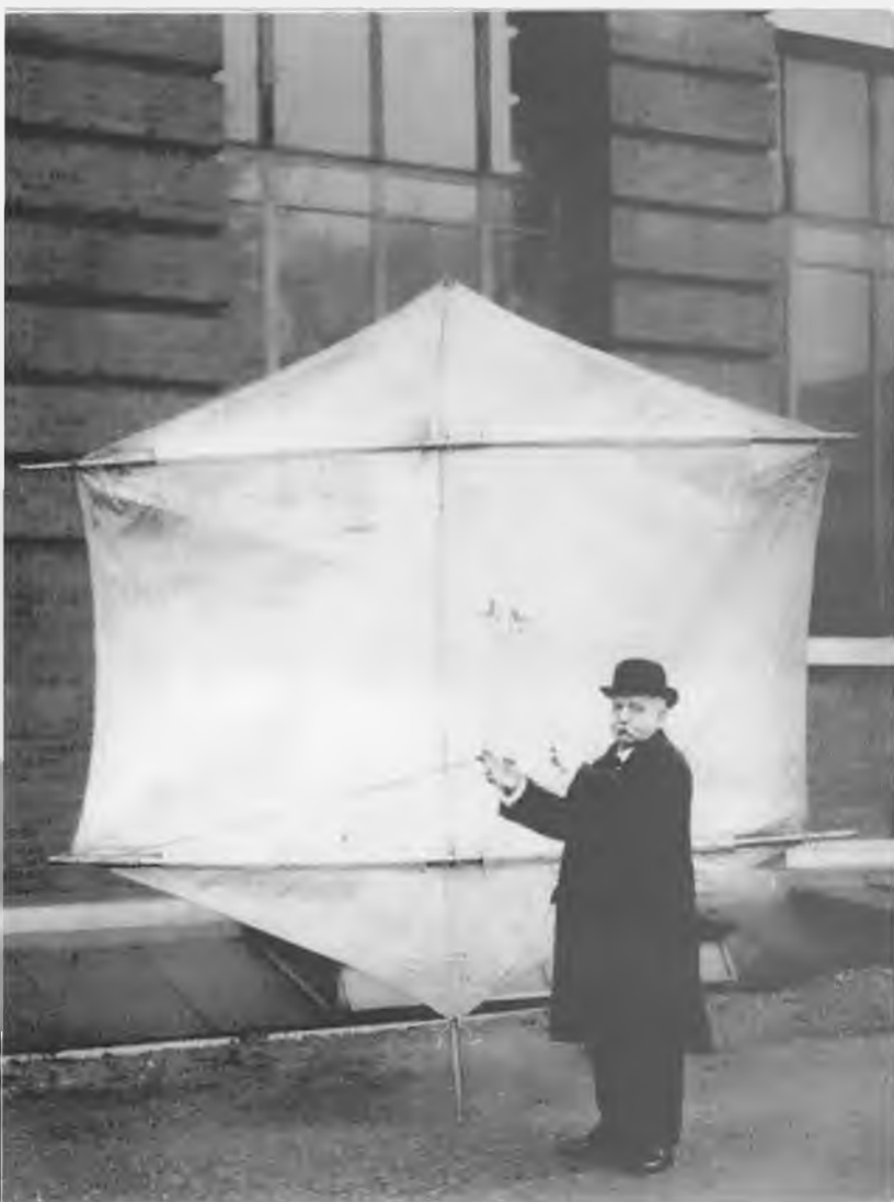
Photo 1: A Baden-Powell "Levitor" man-lifter kite of the type used by Marconi. Person believed to be Captain BFS Baden-Powell (1, 2).
