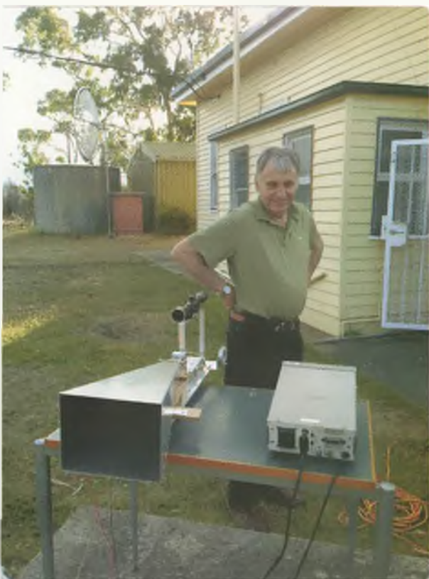
Photo 2: Rex VK7MO showing varying microwave noise levels using a 10 GHz horn and power meter. (Photo courtesy of Justin VK7TW).
