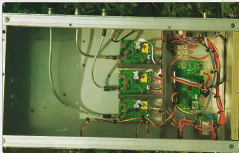
Photo 1: Beacon Drivers: The multi-beacon controller on the right and the three ZLPLL boards with shields to the left. Bottom right is the temperature compensated crystal oscillator and just visible at the top right is the DTMF decoder module. The BNC socket at top right is for the GPS unit on the multi-beacon controller.
