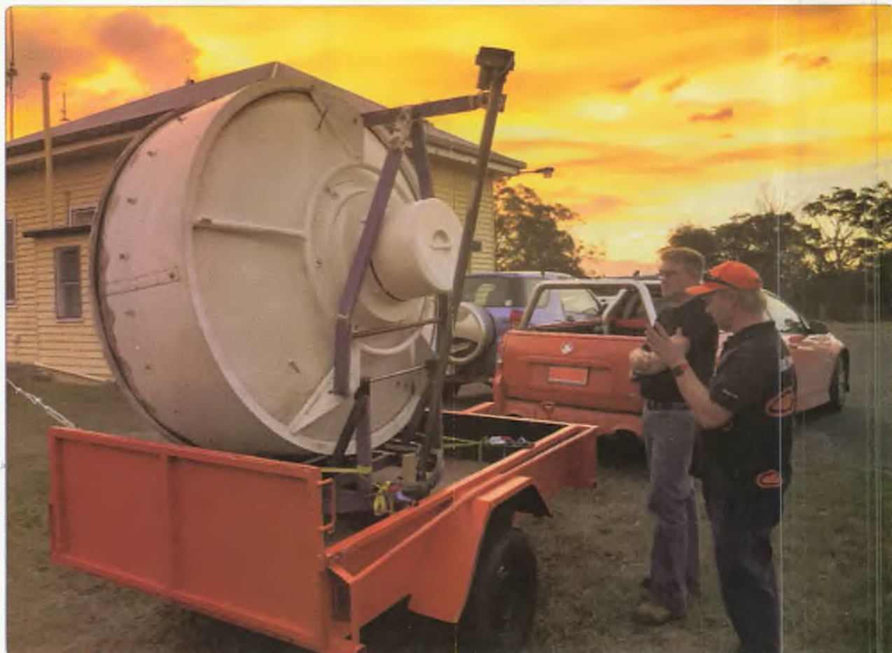
Photo 3: L to R: Sean VK7FAZE and Richard VK7ZBX next to the trailer mounted 1.8 m 10 GHz dish. (Photo courtesy of Ben VK7BEN.)
