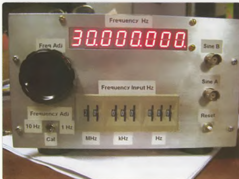
Photo 1: Lou VK3AGH's Arduino Signal Generator.
