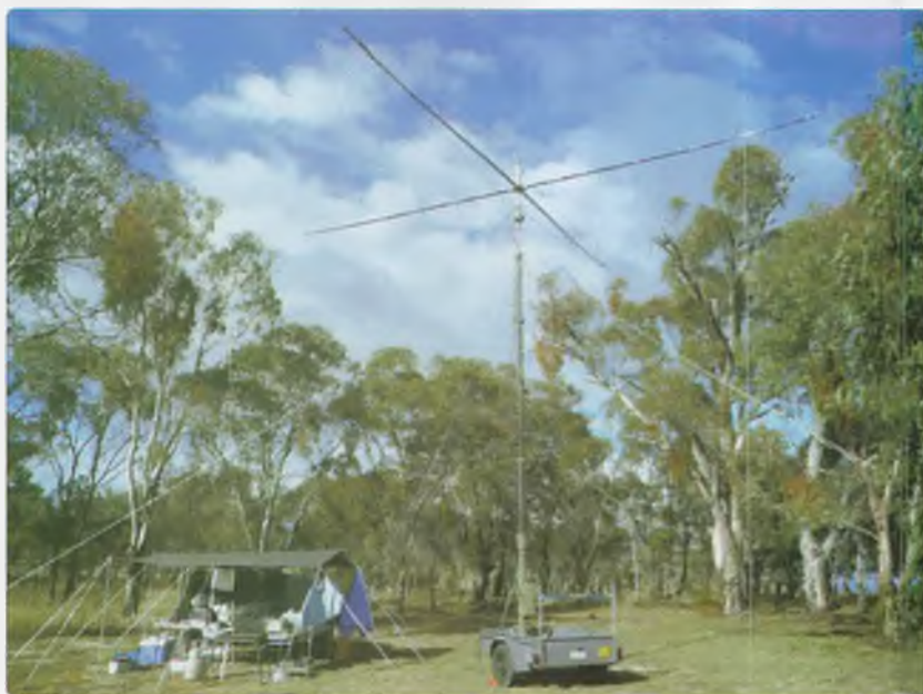
Photo 2: The portable Spiderbeam setup by Catherine VK4GH.
