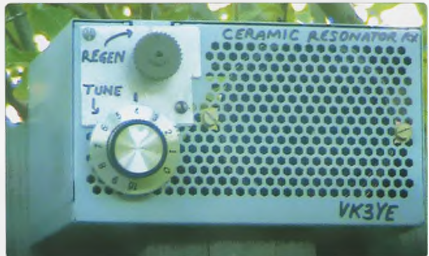
Photo 1: Front of the regenerative receiver.
