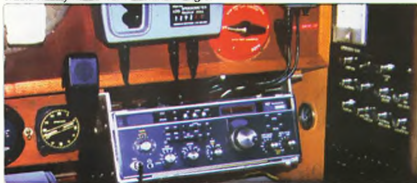
Photo 3: A shot from the navigator's cabin showing the Drake TR7 mounted in a cradle hastily made from aluminum angle.
