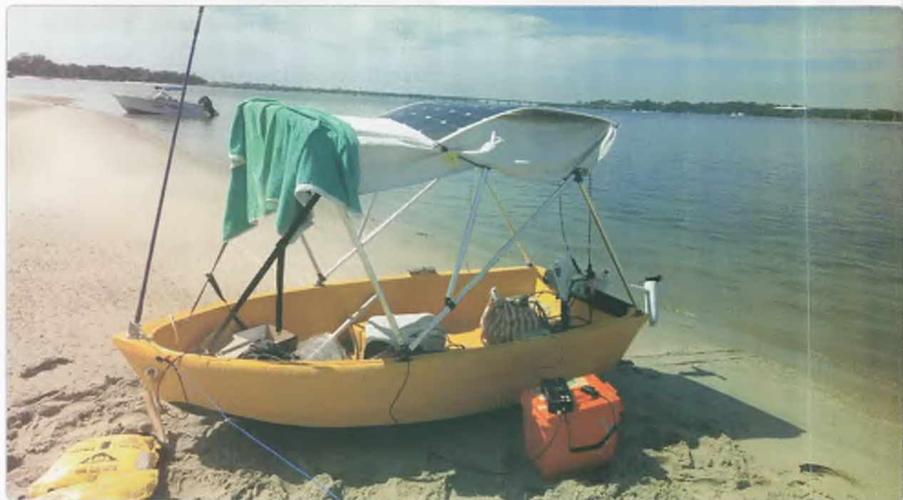
Photo 1: The solar powered boat. The Bimini top holds the 200 watt flexible solar panel.
