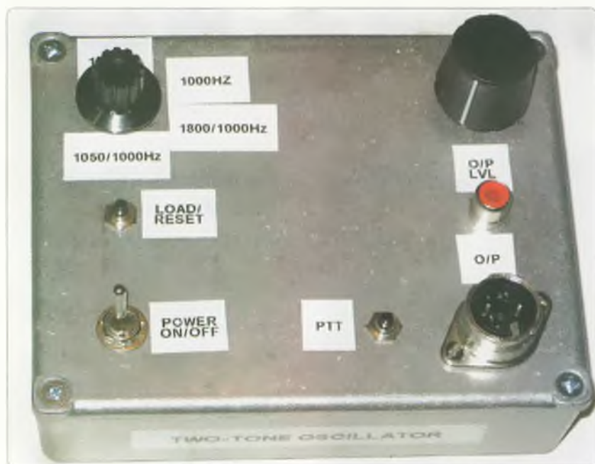
Figure 5: The complete unit built into 119 x 94 x 34 mm diecast box (Jaycar HB-5067 or equivalent).
