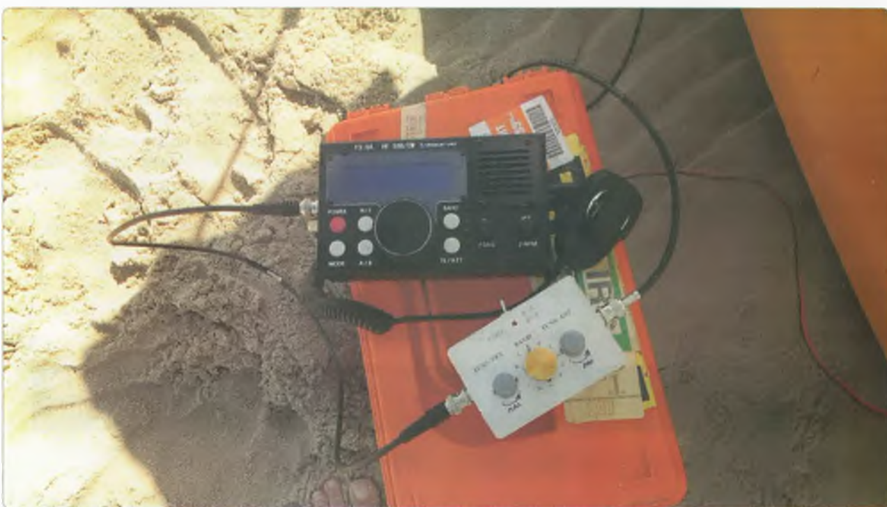
Photo 4: The FX-9A transceiver and antenna matching unit sitting on the battery box.
