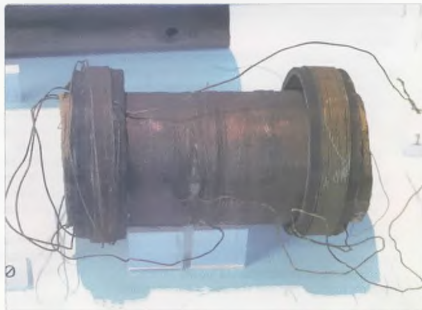
Photo 3: Marconi Jigger – the device kept secret as it made the system more selective - really a form of resonant coupling (patented by Oliver Lodge in 1897) used in the aerial circuit of the receiver and later the transmitter. Image courtesy Peter Wolfenden VK3RV.
