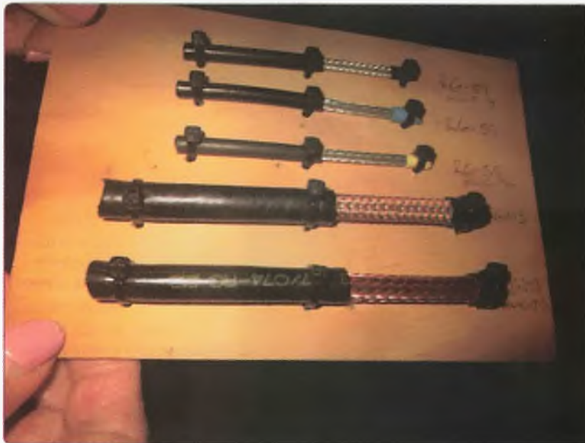
Photo 3: Some samples of RG-59 and RG-213 coaxial cable.
