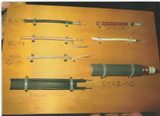
Photo 1: Smaller size transmission lines.
