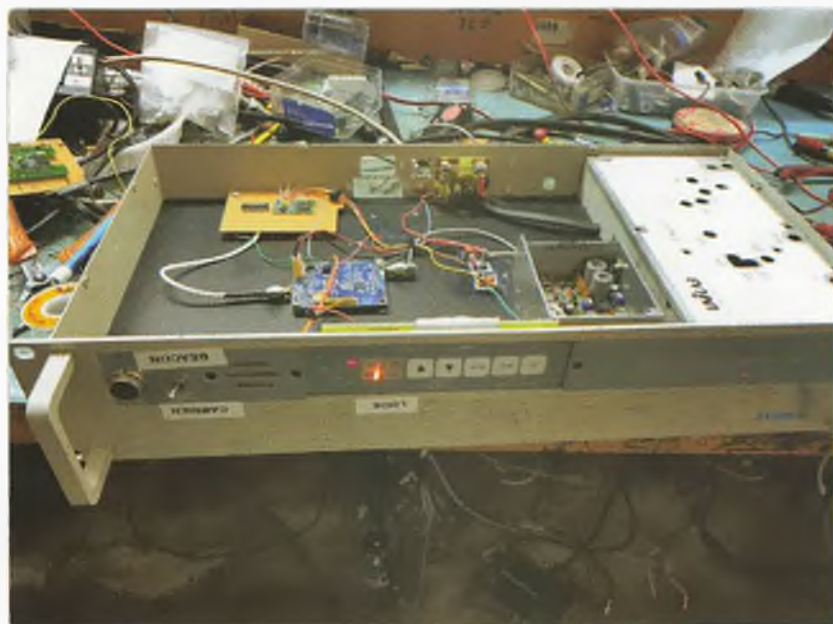
Photo 3: Inside the new VK2RSF 144.415 MHz Beacon. Photo by Joe VK7JG.
