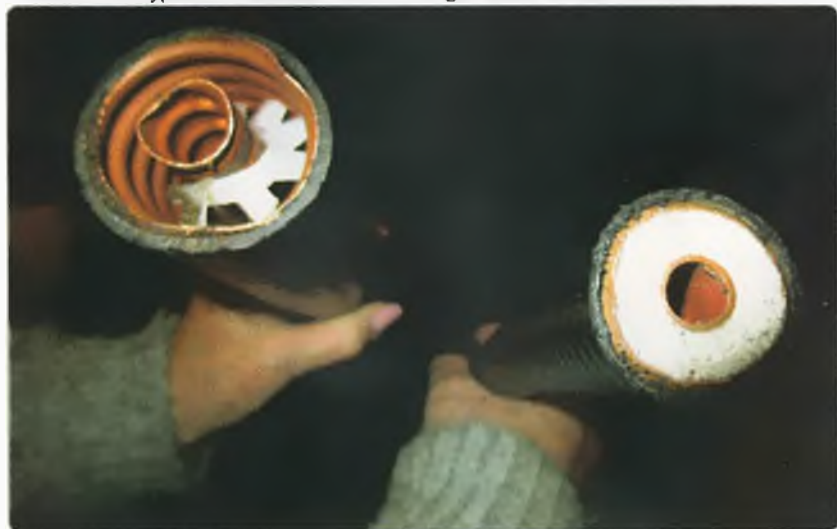
Photo 2: Two types of insulation found in larger sized coaxial cables.
