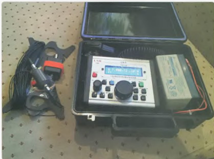
Photo 2: The transceiver, SLA battery and end fed antenna make a compact combination.
