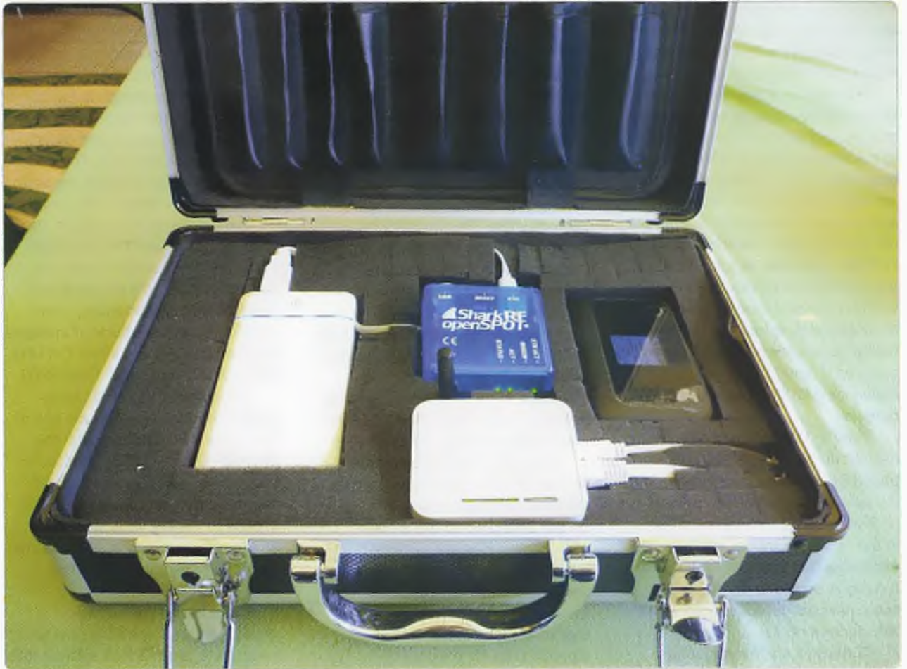
Photo 4: VK5JP's OpenSPOT setup, operating from within its transport case.
