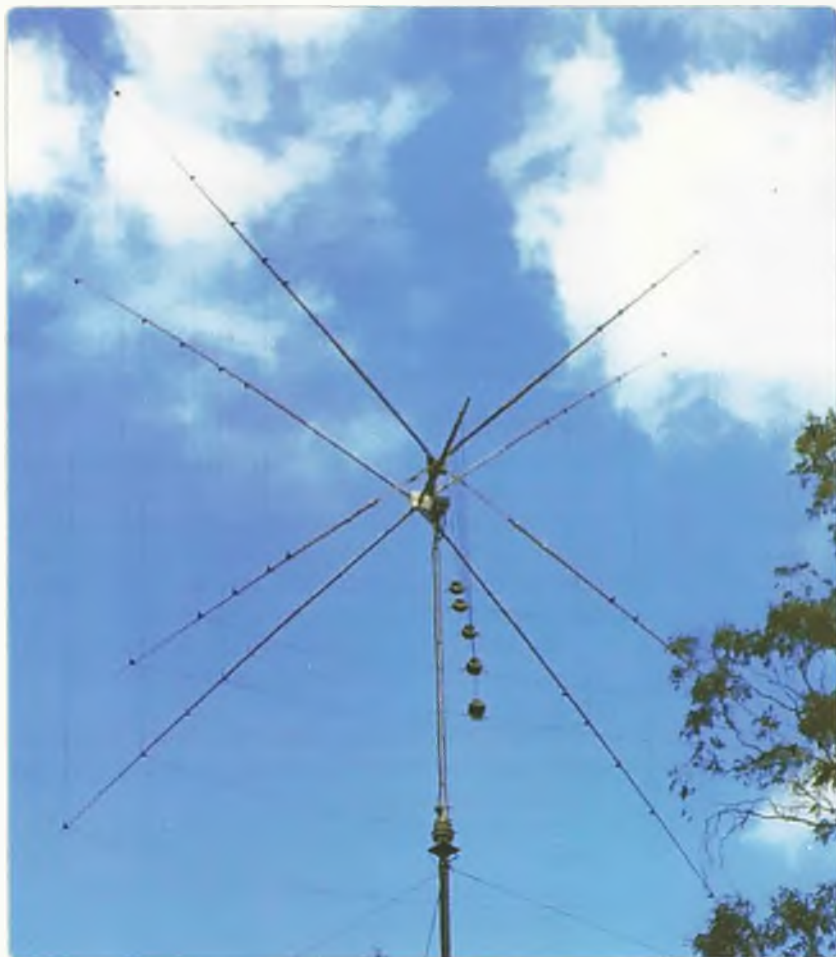
Photo 4: The 5-band quad antenna.
