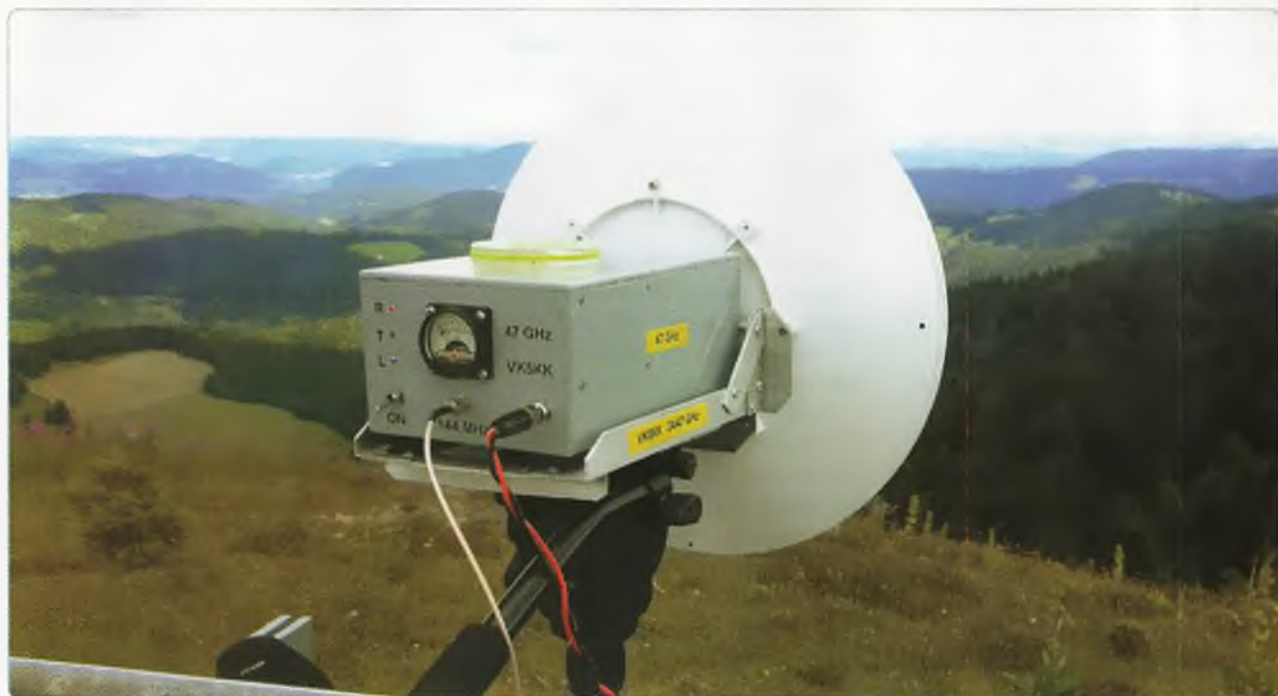
Photo 2: Plug n Play system - 47 GHz transverter mounted.
