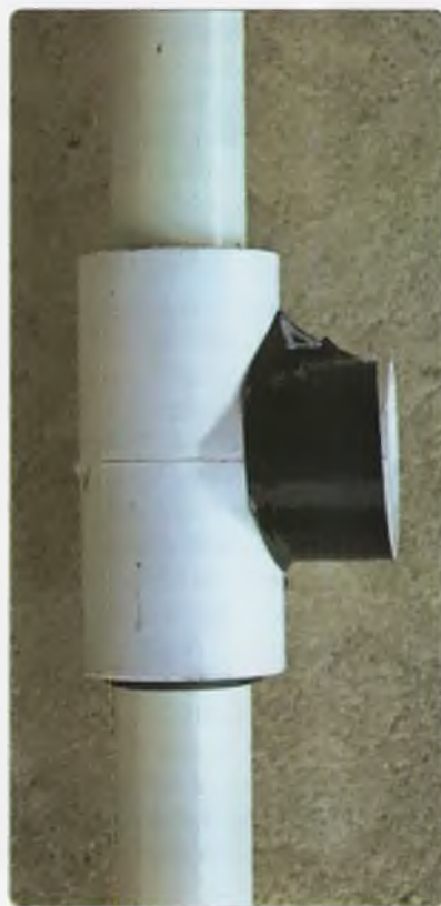
Photo 7: The T-piece over the boom, with electrical tape to fasten to the mast. Just visible at right is one of the O rings which stabilise the T-piece on the boom.
