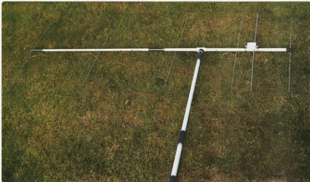
Photo 6: The Yagi and mast assembled and ready to raise to the vertical position.
