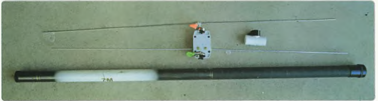
Photo 3: The Driven element, mast and mast-boom bracket
