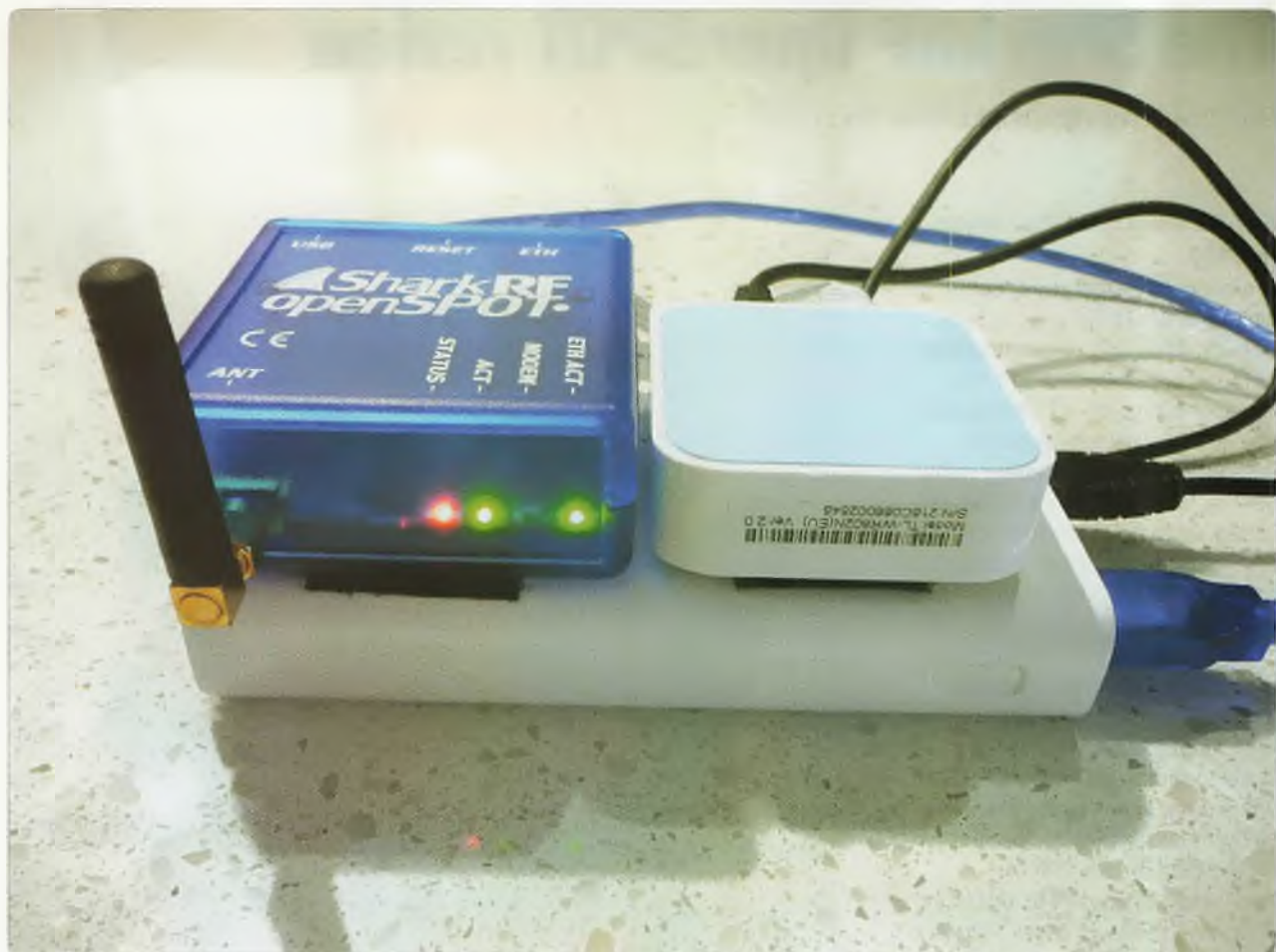
Photo 2: The OpenSPOT in operating mode, the OpenSPOT and the TP Link router affixed on top of the 5 volt battery power pack. VK5BB.
