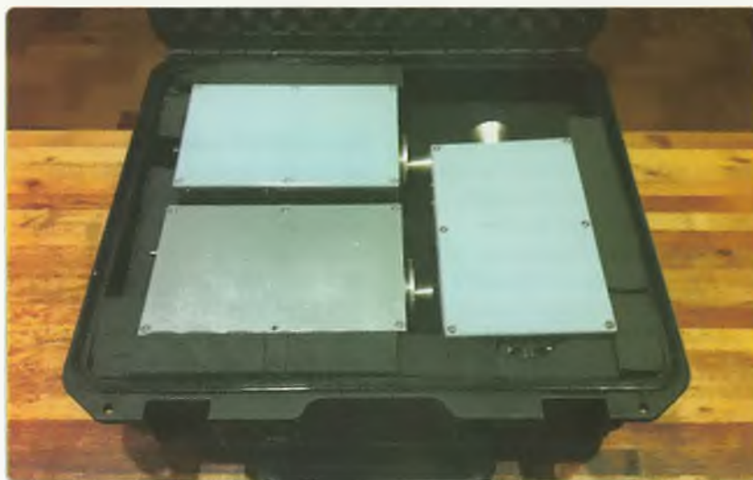
Photo 4: 24, 47 and 76 GHz Transverters in their transport case.
