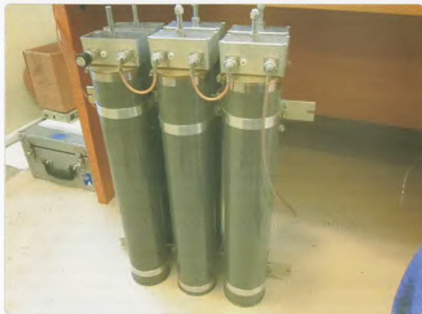
Photo 3: The refurbished W1GAN duplexer nearing completion showing 19" rack-mount frame and lugs.
