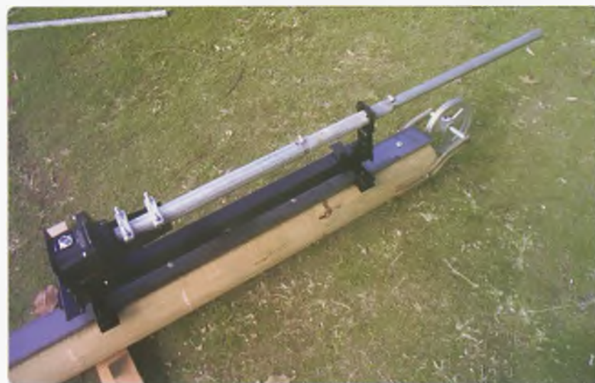
Caption 2: The stub mast and rotator carriage installed on the carrier rail.
