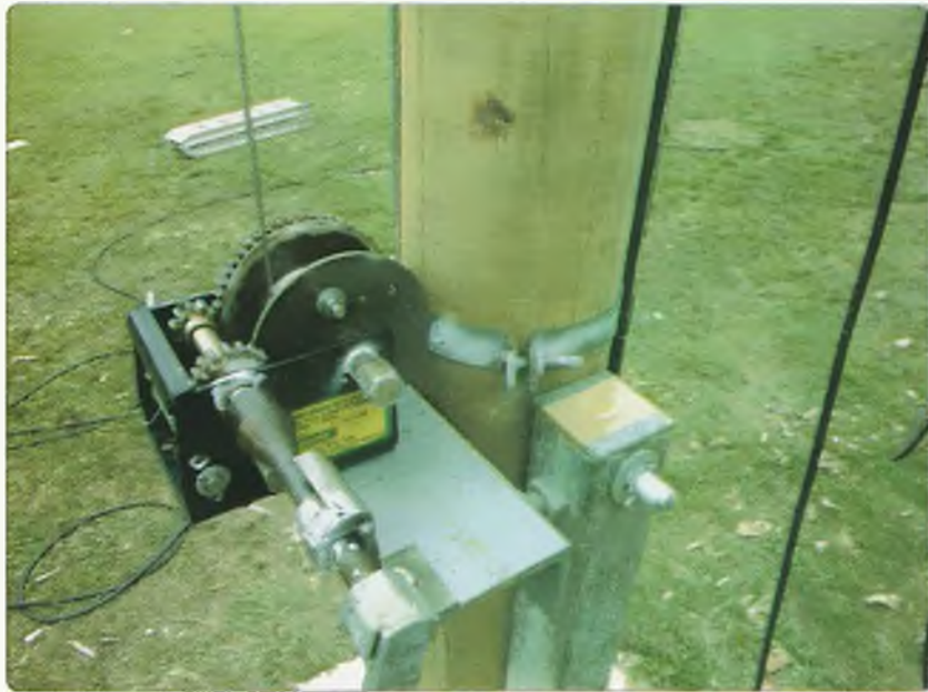
Photo 7: The winch to raise the carriage assembly up the track.
