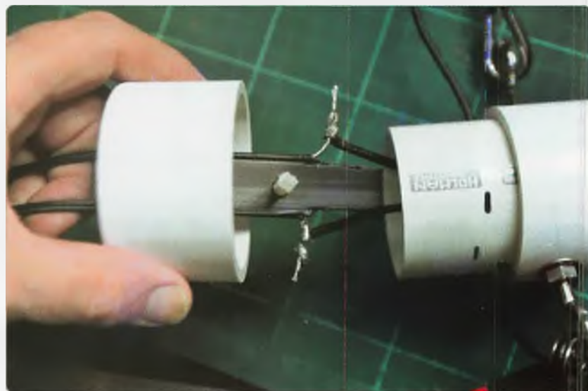
Photo 2: The window line soldered and ready to be potted.
