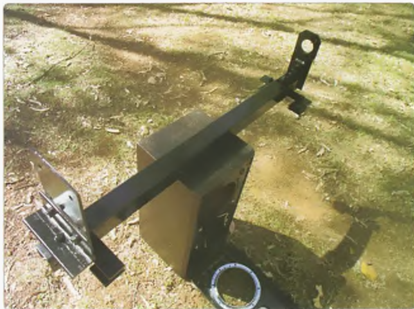
Photo 1: The stub mast and rotator carrier.
