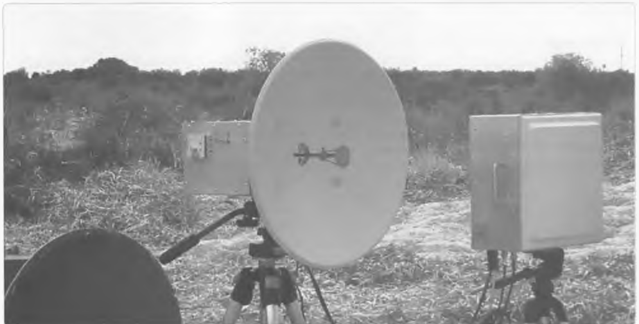
Photo 5: VK5ZD 47 GHz system with 400 mm dish.
