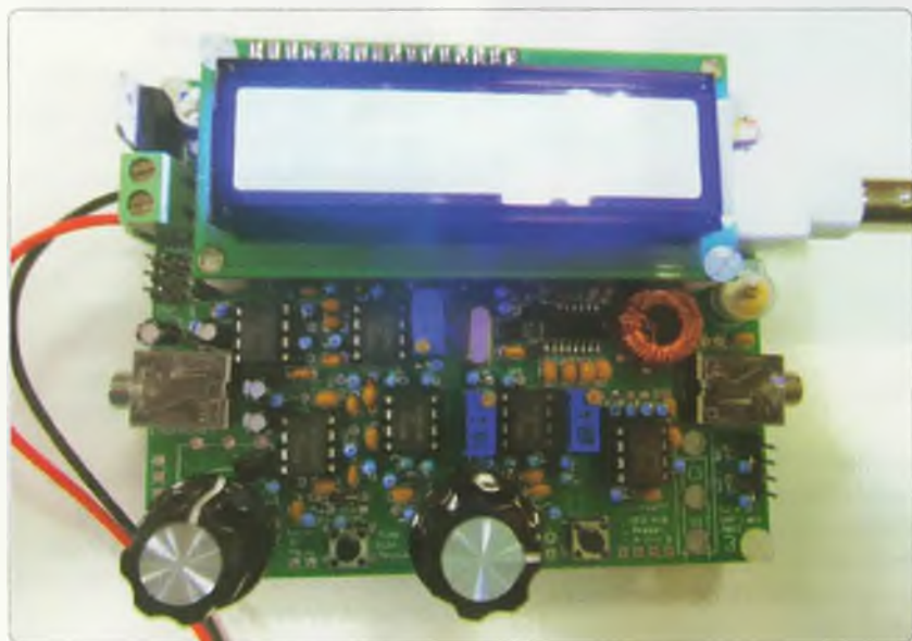
Photo 1: The QRP Kits CW transceiver built by Trevor VK5AZQ.
