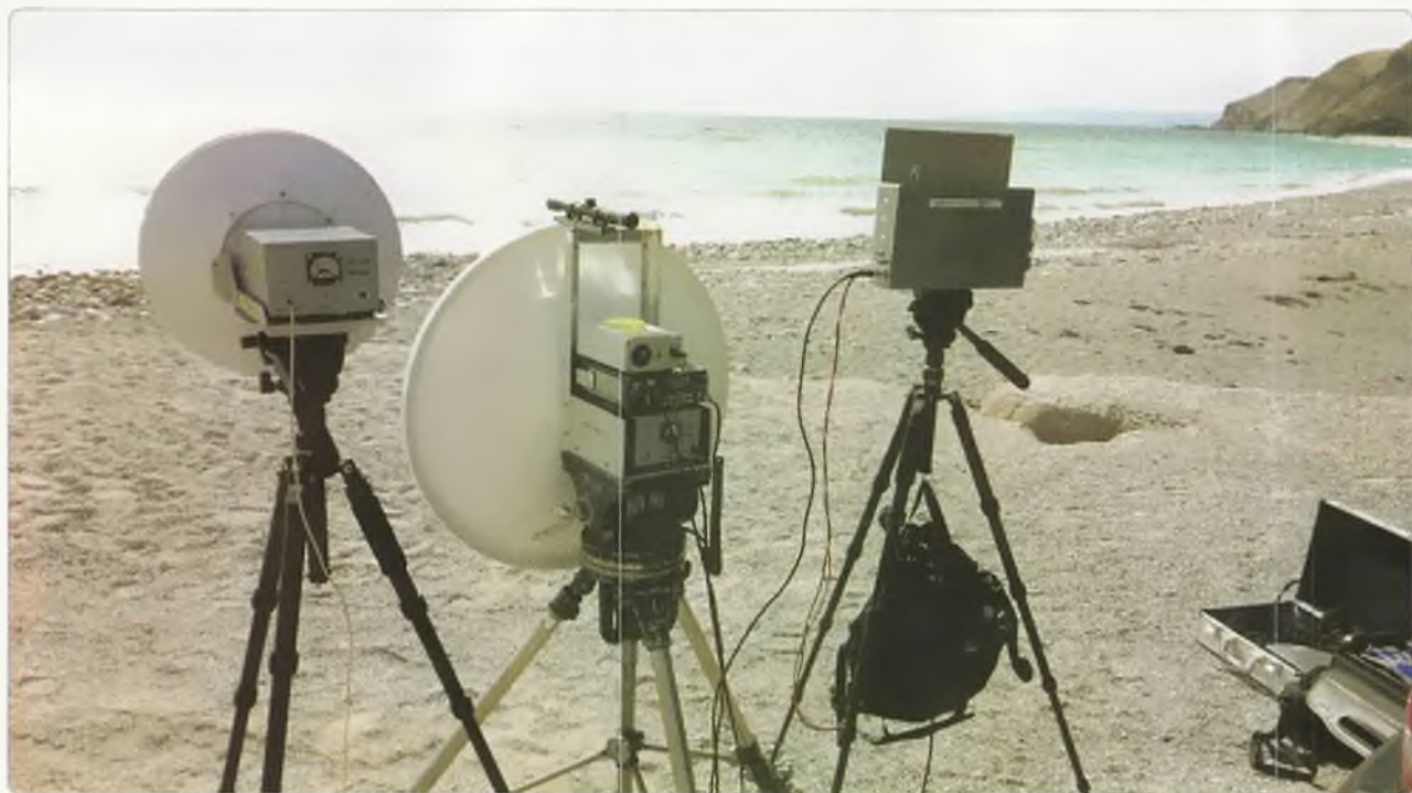
Photo 4: VK5KK 47 GHz 600 mm dish flanked by 24 & 10 GHz.
