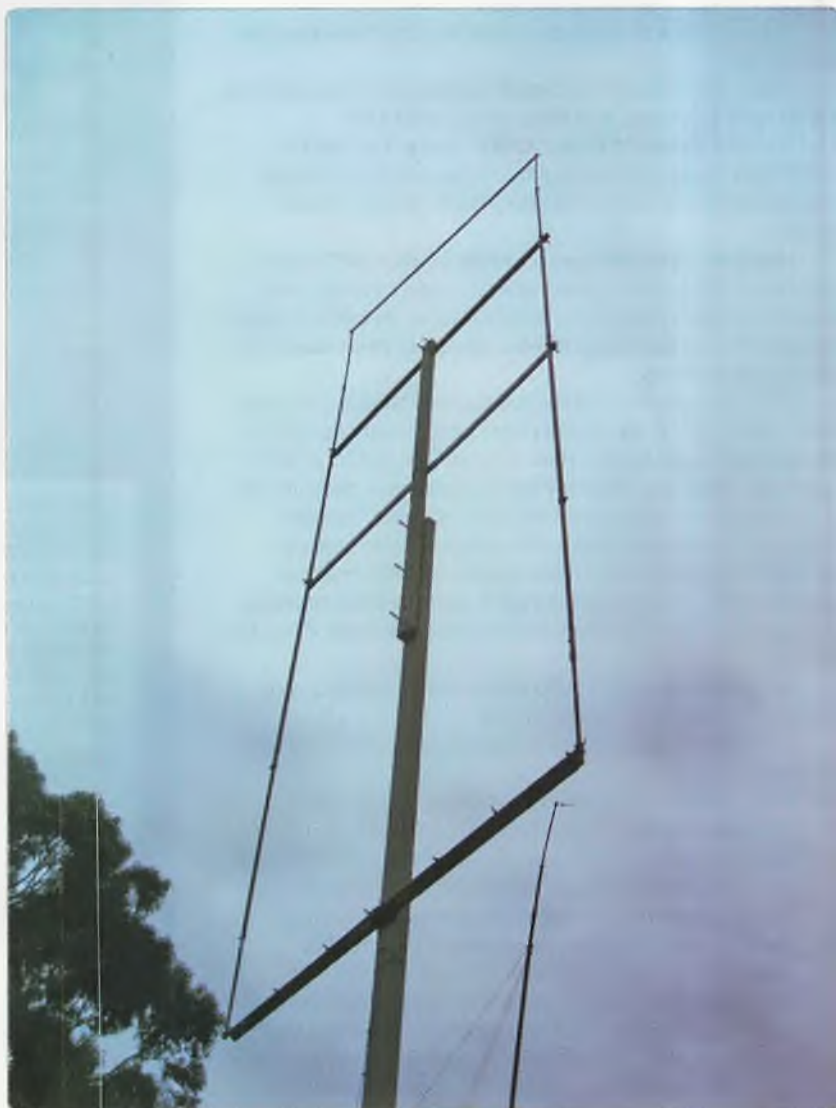
Photo 1: A vertically-mounted, single element, horizontally-polarised 28 MHz loop only 4.5 m above ground.
