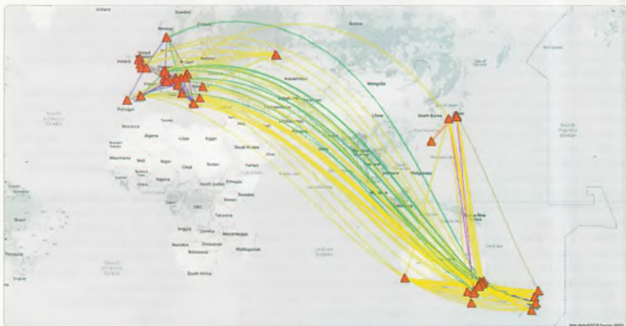
Photo 1: Map of S2S contacts made, showing the short path connections between stations. Many of the contacts between VK/ZL and EU were likely to have been made via the long path. Acknowledgments to Manuel HB9DQM, ( https://neon1.net/sota/s2sviz/20180310/ ) and Google Maps.
