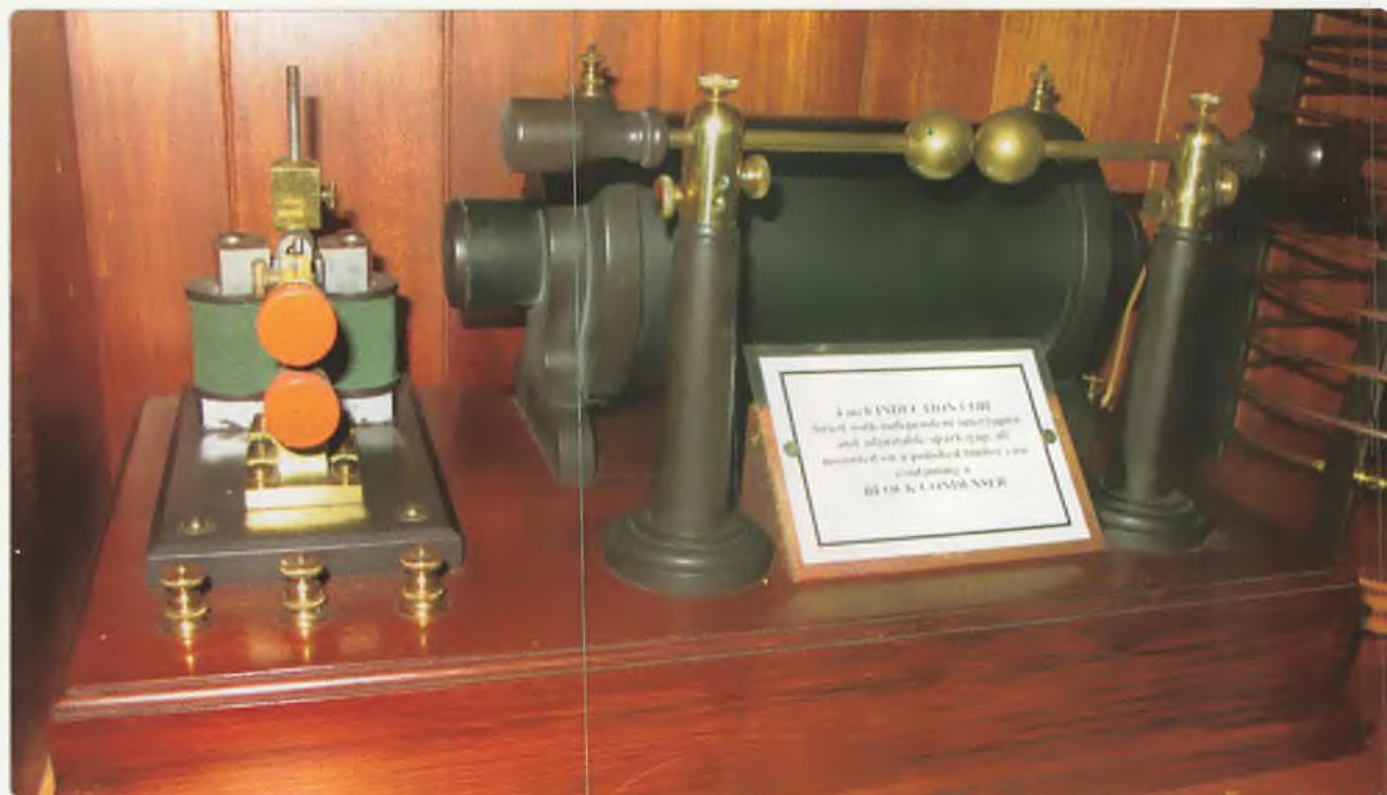
Photo 3: Close up of XQA Spark Transmitter, showing Induction Coil, Interrupter and Glass plate capacitor in box underneath (Photograph Kevin Zietz VK5AKZ).
