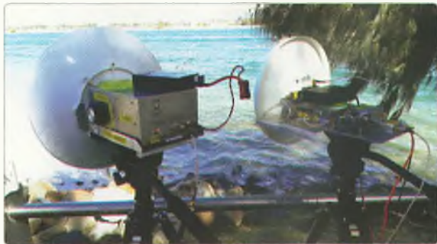
Photo 7: 76 & 122 GHz "Over water test" at the Gold Coast WIA AGM.
