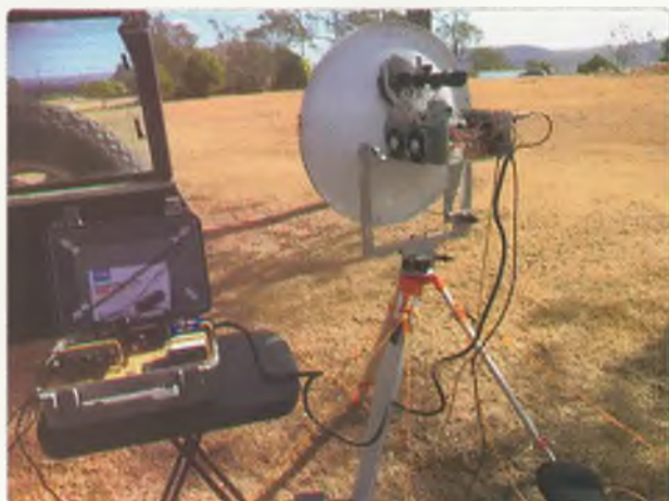
Photo 5: 10 GHz equipment used at the VK4UH end of the VK4 Record.
