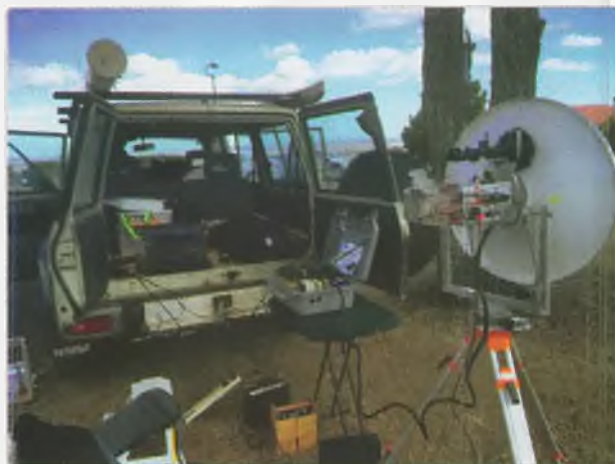
Photo 6: The complete VK4UH 10 GHz portable station.
