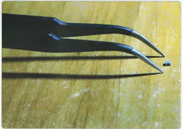
Figure 6: Tweezers and 0805 SMD capacitor.
