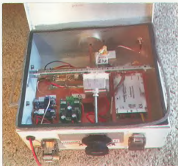
Photo 8: VK2GG's 76 GHz Transverter with rotating RX/TX Amplifier.
