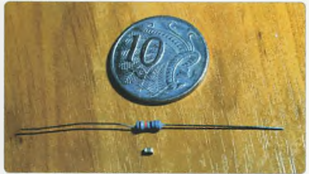
Figure 5: Comparison of leaded resistor and 0805 surface mount capacitor.
