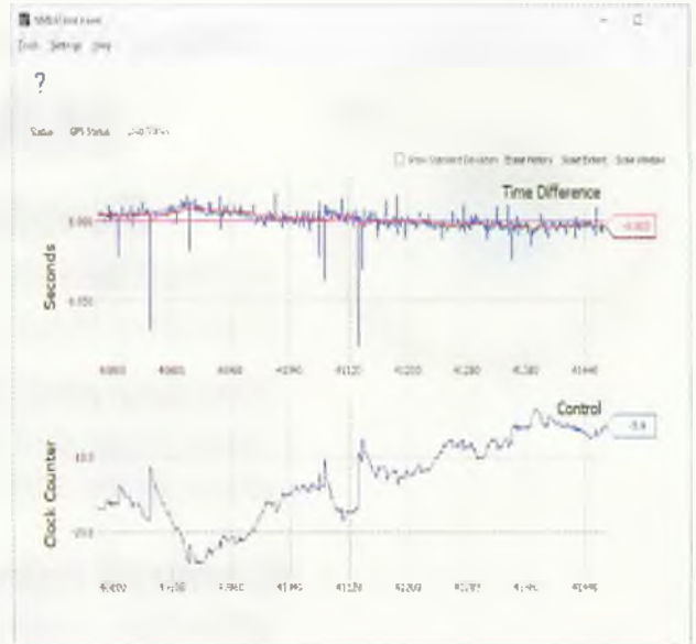
Photo 9: The NMEA Time software Loop Status screen showing the status history of the receiver and software. (Source: Primary)
