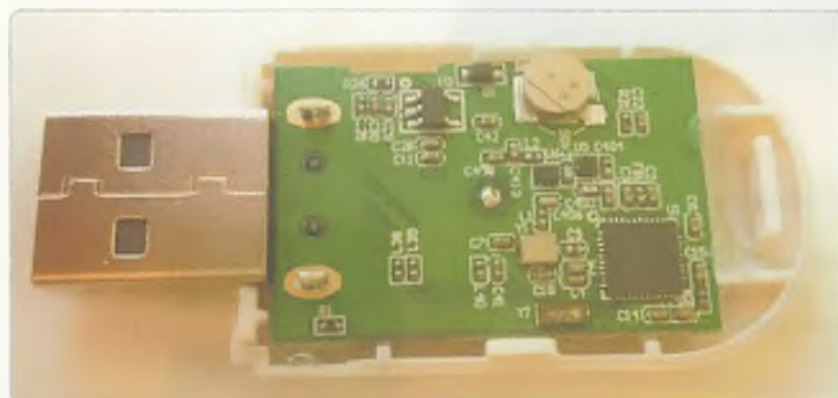
Photo 3: An internal view of the NEO-7M deployed in a “VK-172”. (Source: https://forum.u-blox.com/?qa=blob&qa_blobid=11316380723856418927 )
