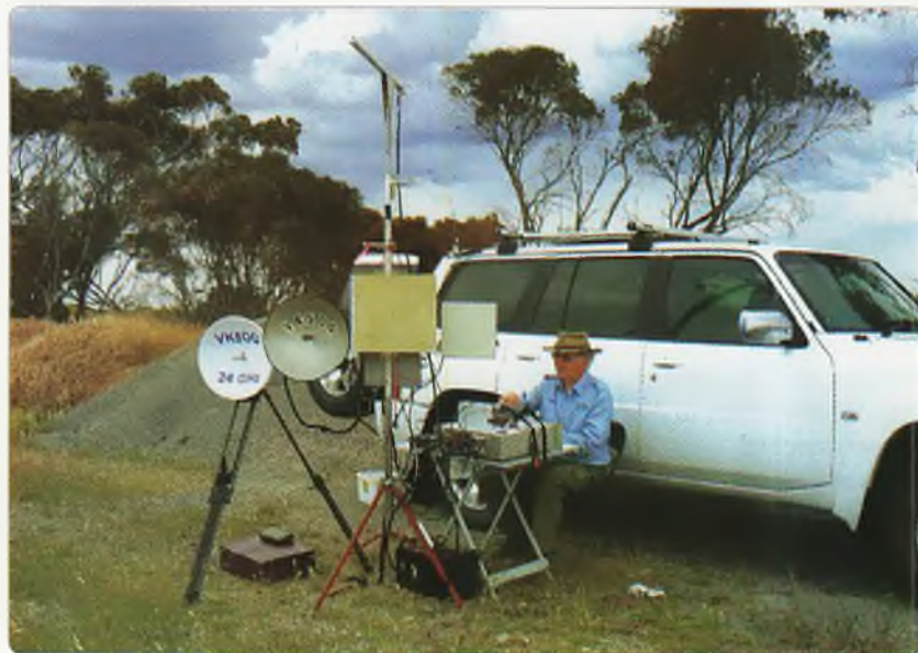
Photo 12: Keith VK5OQ's 1.2 to 24 GHz Portable Station.
