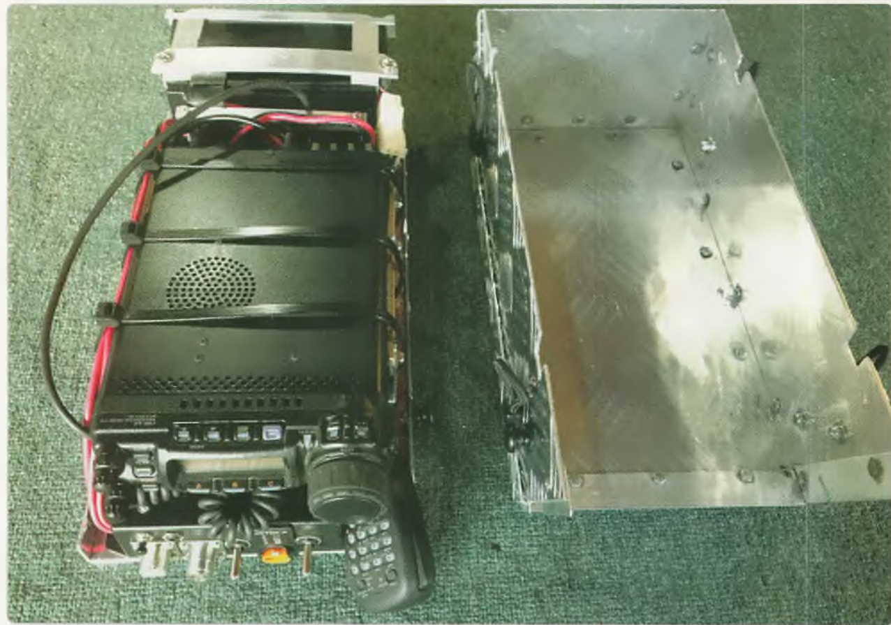
Photo 1: All components secured on the base plate, and the large cover.
