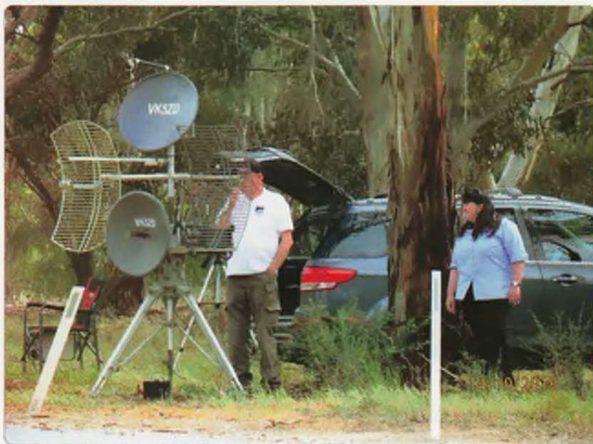
Photo 11: Iain VK5ZD's 1.2 to 10 GHz Portable station.
