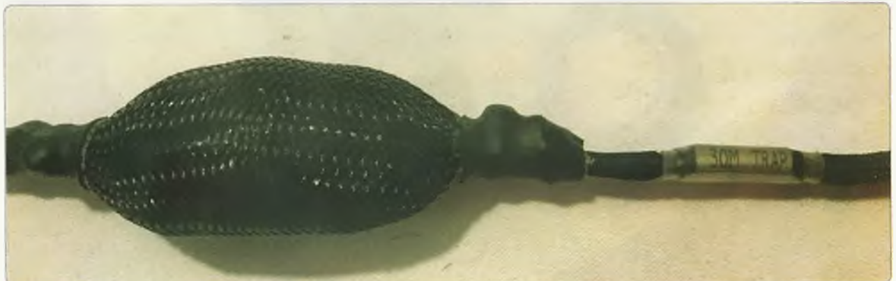
Photo 5: The braided wrap in position over a trap, secured to the cord with heatshrink, and the label of the trap.
