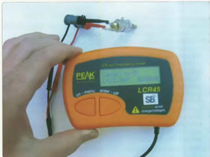
Photo 1: LCR45 testing a beehive trimmer capacitor.
