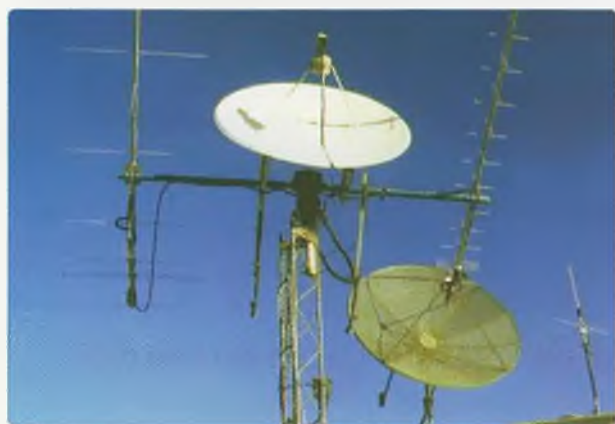
Photo 3: VK6MJ 1.2 and 2.4 metre dish antennas.
