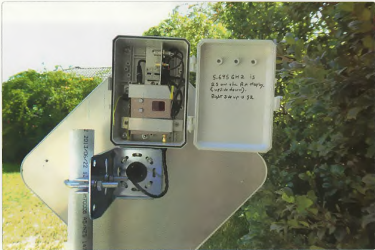
Photo 2: The 6 cm receiver mounted at the rear of the antenna.
