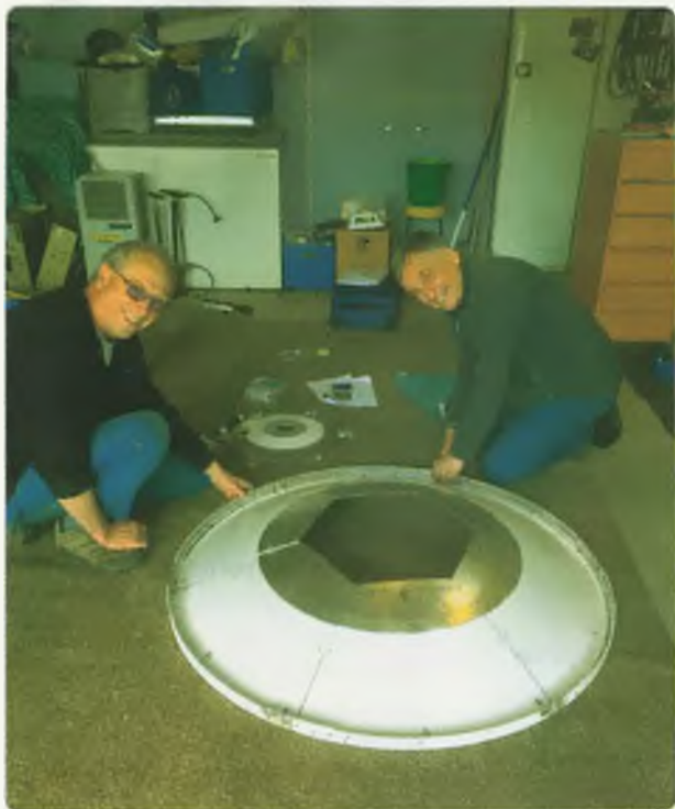
Photo 3: Roger ZL3RC (left) and Rex VK7MO (right) assembling cut-up petal dish.
