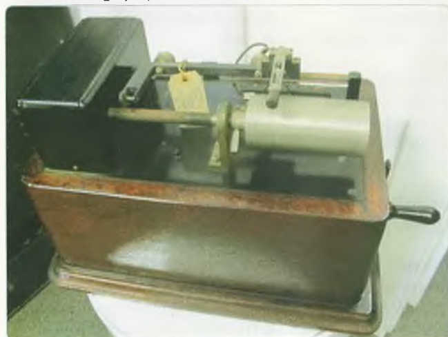
Photo 3: Fultograph picture receiver.
