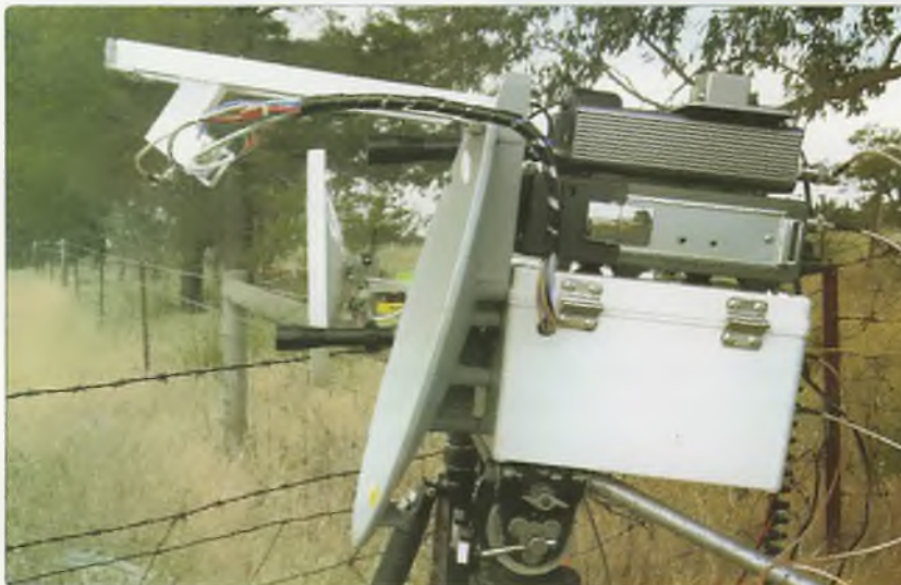
Photo 4: Close up of 122 GHz Feed and Offset Angle.
