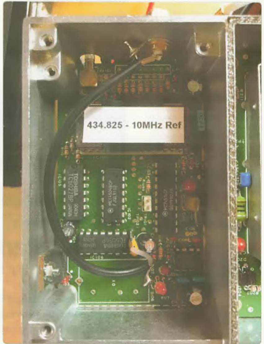
Figure 5: PLL compartment of the KL receiver.
