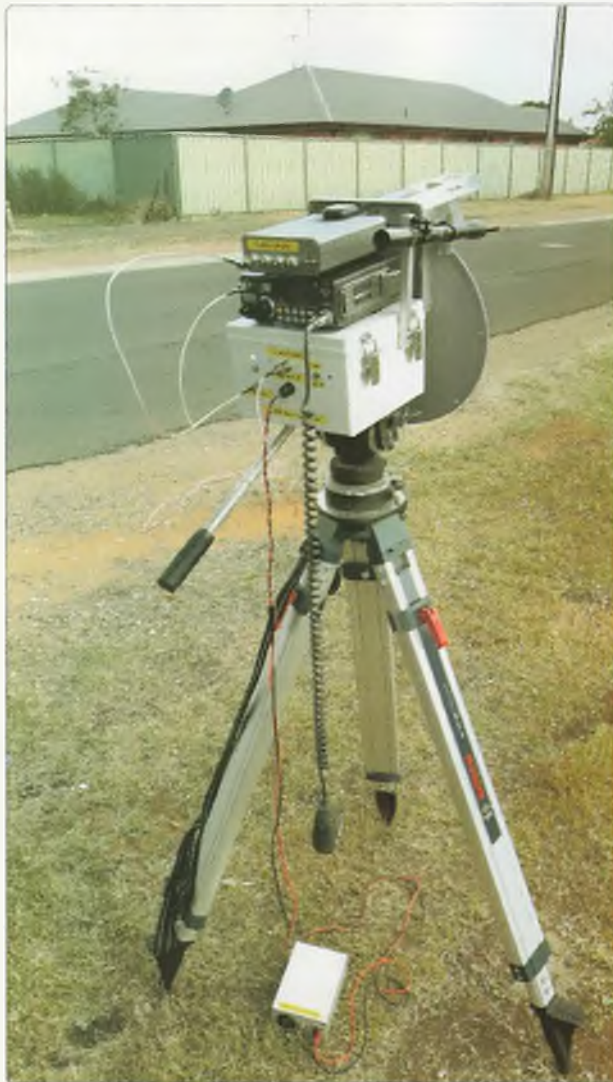
Photo 3: VK5KK's 122 GHz Offset Dish System with GPS locking.
