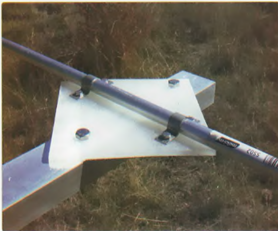
Photo 5: Detail of an element to boom mounting.
