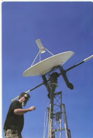
Photo 4: Dish Antenna at the ARISS ground station.
