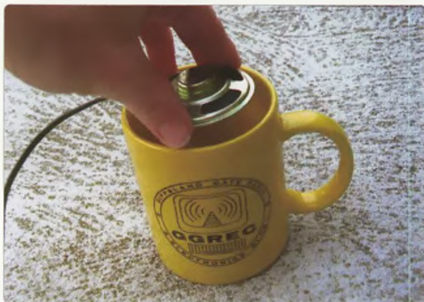
Photo 3: An audio filter can assist reception of weak signals, especially if there is interference on an adjacent frequency. Here is a crude one, using a cup and a salvaged speaker, for CW.
