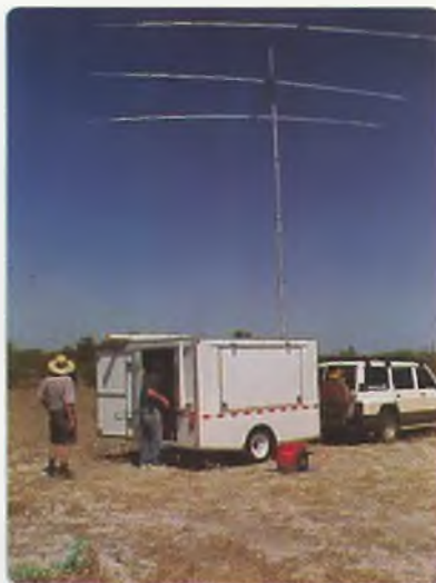
Photo 5: The TH3 beam on its mast.
