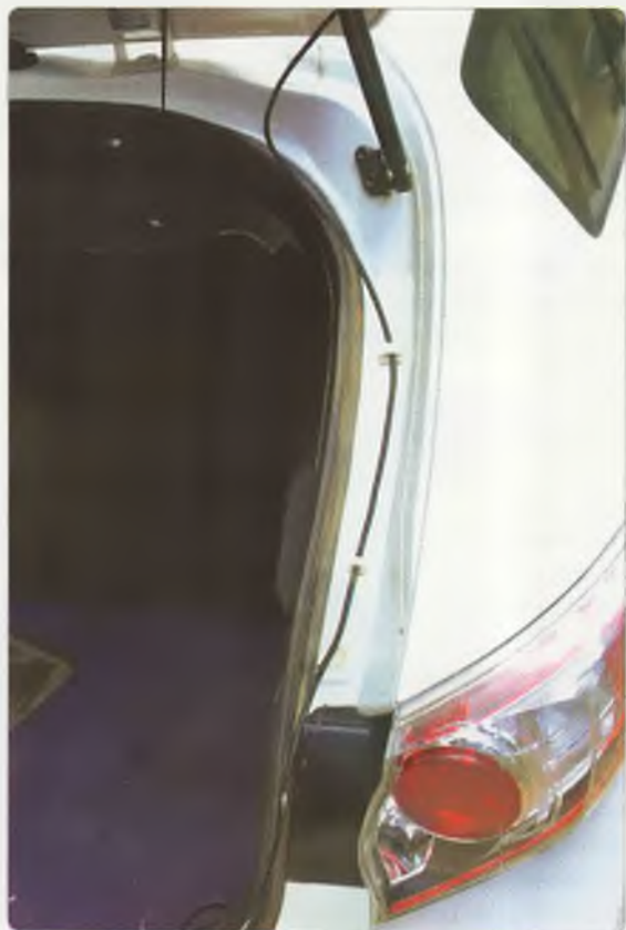
Photo 2: Routing the antenna cable down the hatch.
