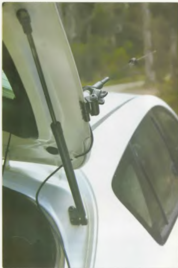
Photo 3: The antenna lies horizontal with the hatch open.
