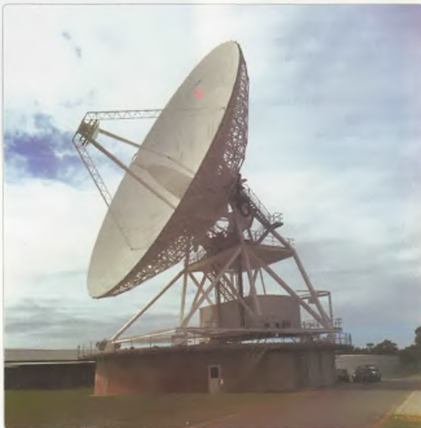
Photo 1: Dish used for the 5.7GHz EME contacts.
