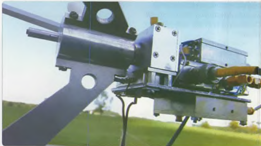
Photo 5: Wolfgang OE4WOG's new miniature 122 GHz transverter.
