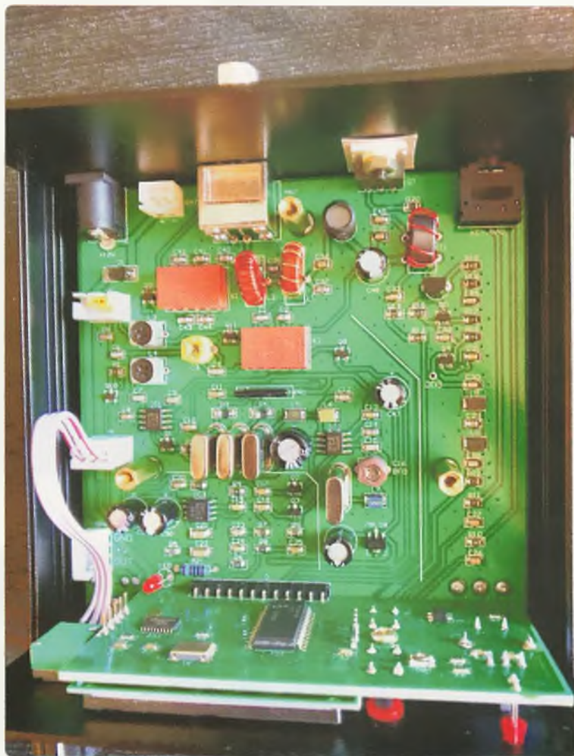
Photo 3: HT-1A Internals - Mix of SMD and "thruhole" components.
