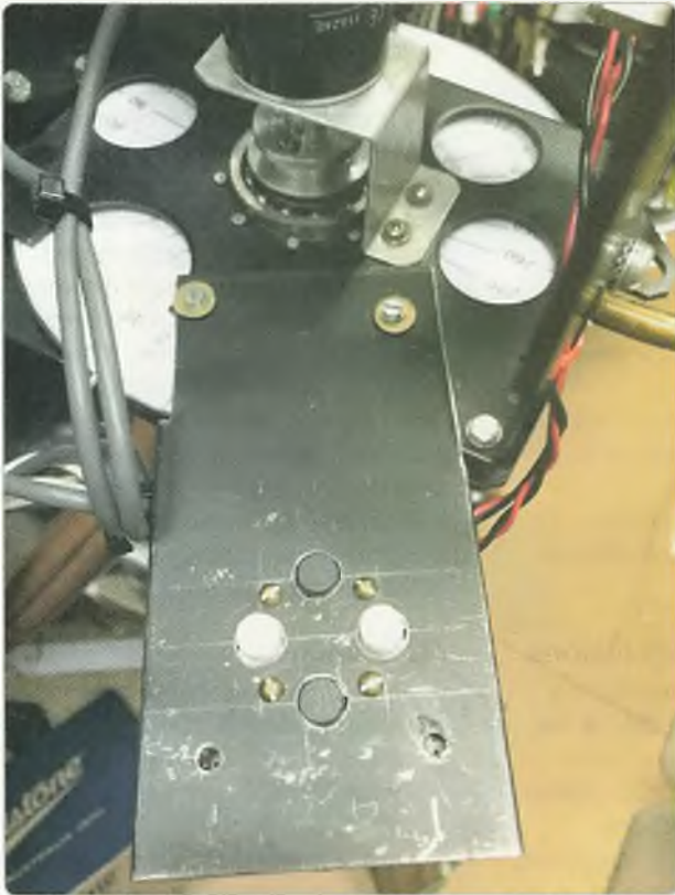
Photo 7: Satellite Az/EL control on the actual mount.
