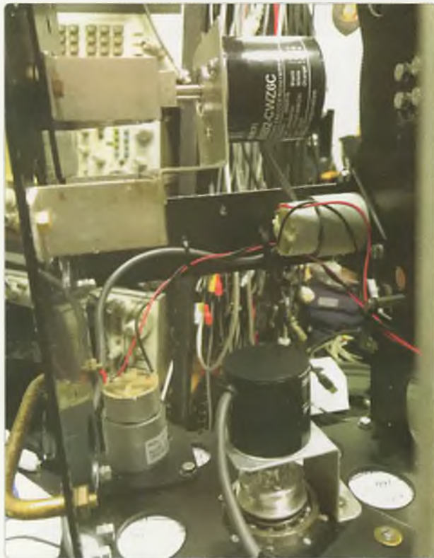
Photo 4: Shows the two silver 12VDC motors and the two black OMRON incremental encoders.
