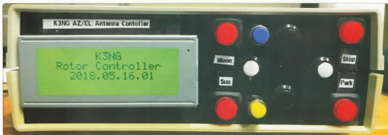
Photo 2: Front Panel – Blue button is calibrate on Moon and yellow button is calibrate on the Sun. Black buttons are up/down and white buttons are counter clockwise/clockwise.
