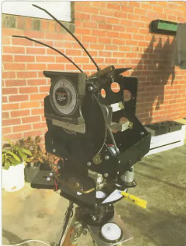
Photo 3: K3NG dish mount with sighting tube – note peg is to hold the azimuth scale whilst the mount is moving.
