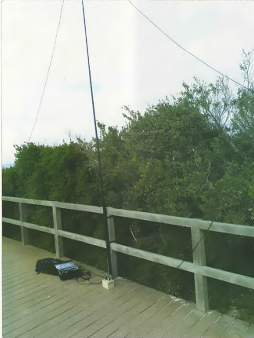
Photo 1: Magnetic loop in use (with 15m RG58 as radiating element).
