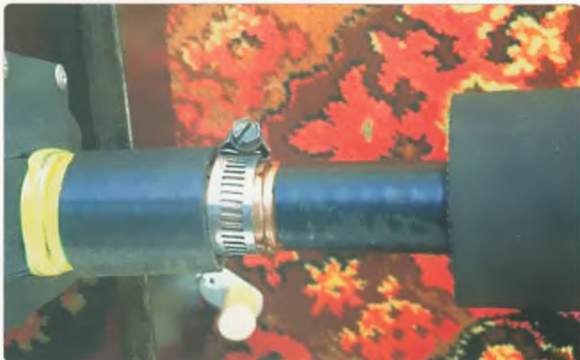
Photo 5: Coax to tube connection.
