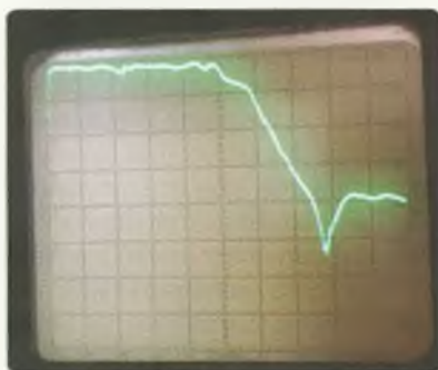
Photo 4: GARC Transverter IF filter plot from 0 – 1000 MHz.
