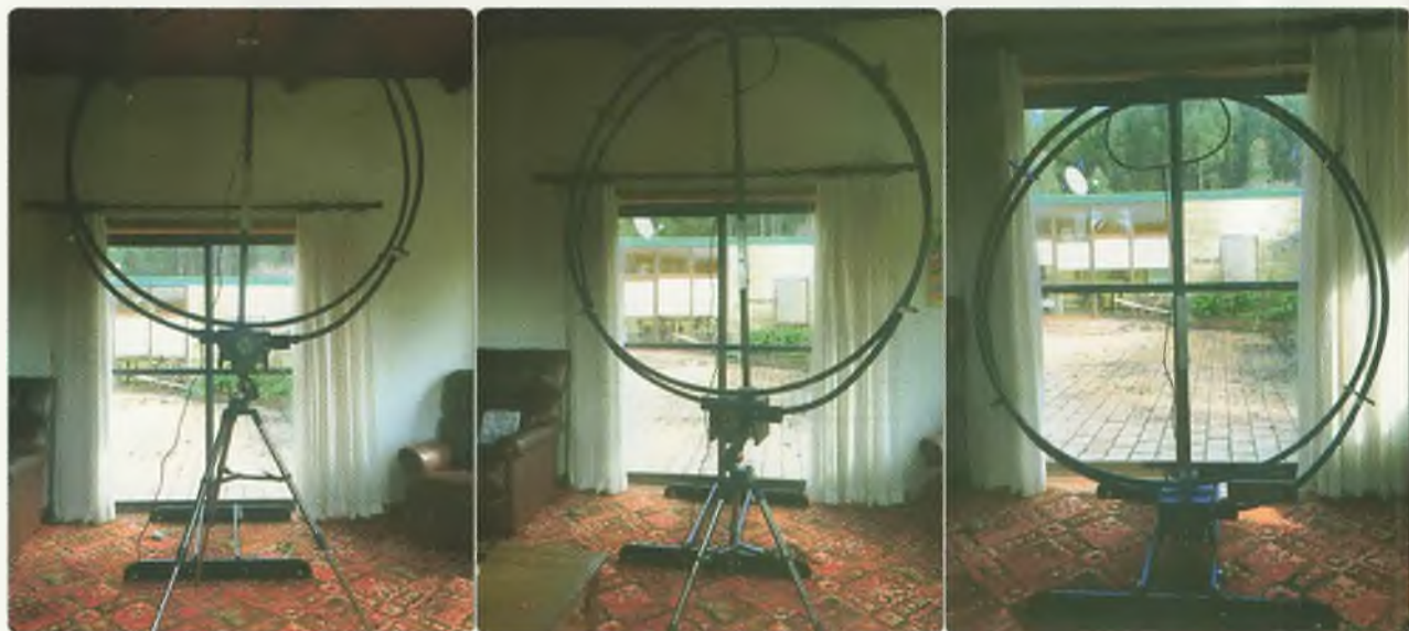
Photos 1, 2 & 3: Loop showing different mounting arrangements.
