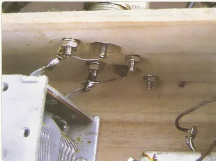
Photo 4: Magnetic loop tuner connections.
