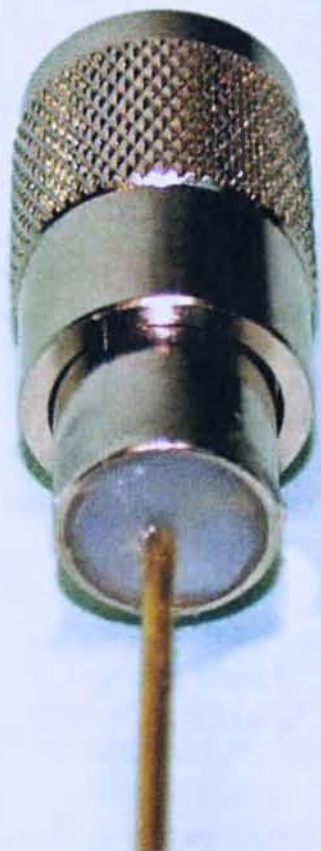
Photo 3: Close up of the homebrew base on the antenna shown in Photo 2.
