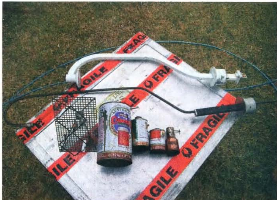
All dish feeds 1.2, 3, 5, 10 GHz with coax feed and alternative 10 GHz waveguide feed for 1.2 m dish.
