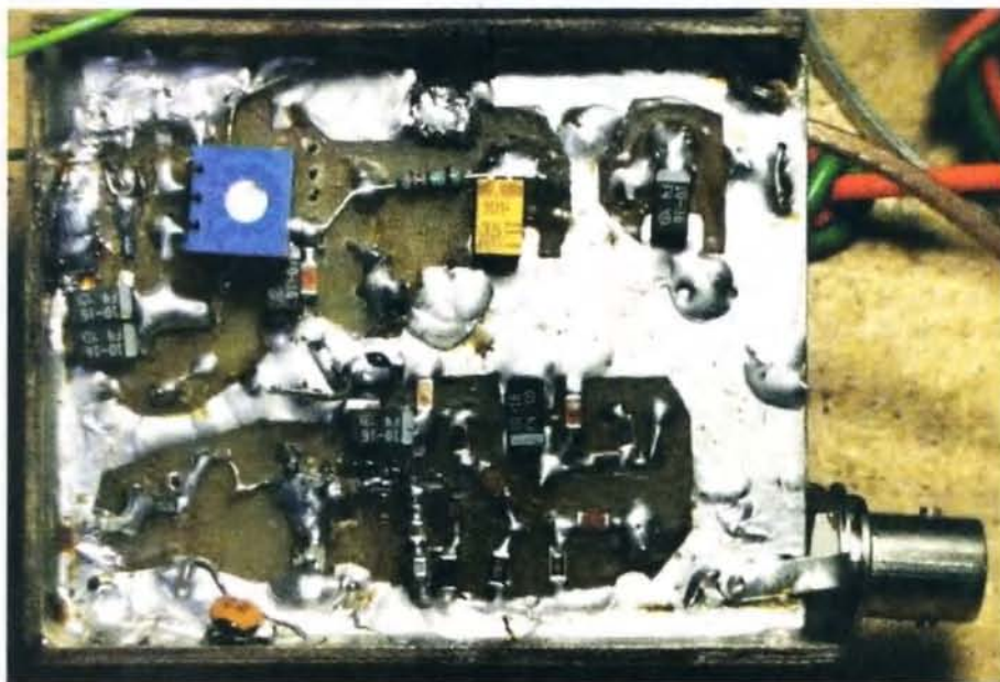
Photo 2 (lower right): The test oscillator, bottom side.
