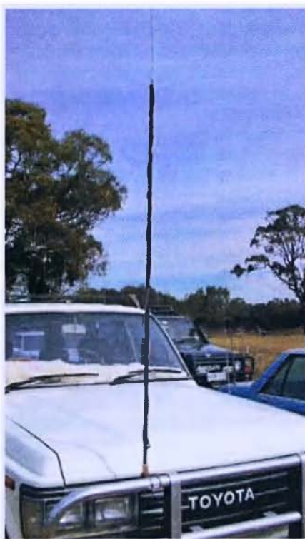
Photo 4: The FAMPARC HF whip shown mounted on a vehicle.
