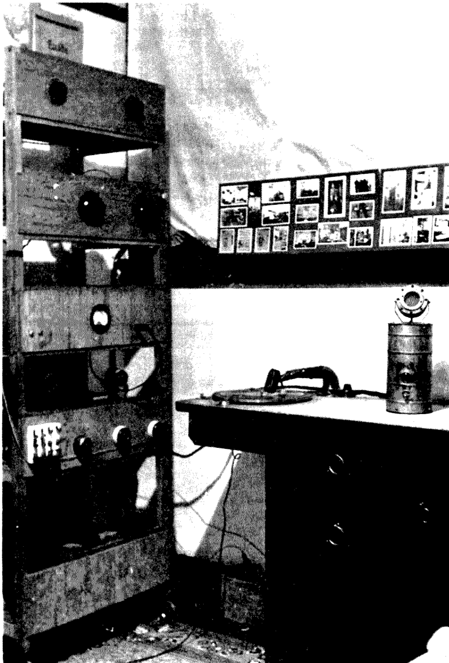
Figure 9: Amateurs also shared the broadcast band. They frequently sent photographs of their equipment with QSL cards. This one was sent to VK3HK from ZL3BQ and it shows the turntable and home-made condenser microphone used at ZL3BQ's "broadcast" facility c1930 (WIAA).
