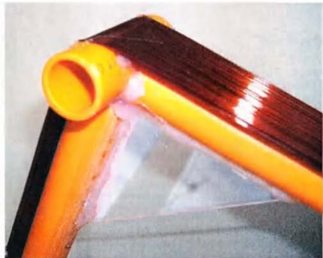
Photo 4: One corner of the loop, showing turns wound side by side upon an 'out-rigger'.
