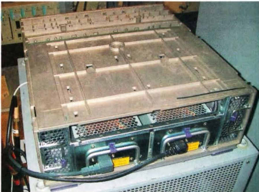
Photo 4: The 46 amp power supply.
