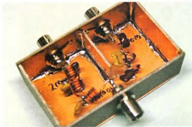
Photo 6: Isolation panel inserted and spot soldered coils.
