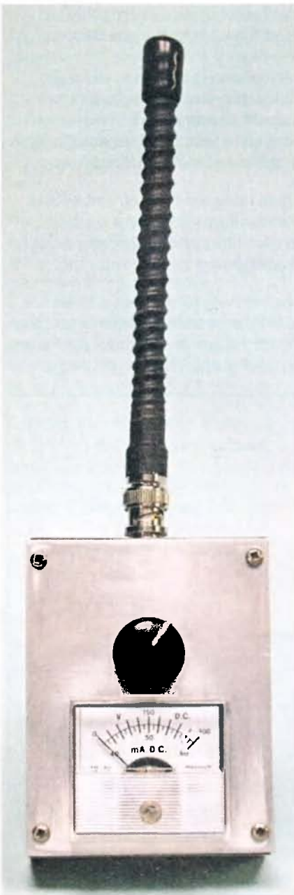
Photo 2: Using a surplus analogue meter for the display.
