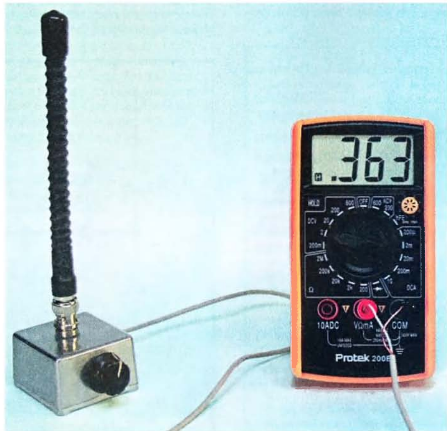
Photo 1: Using a DVM for the display.
