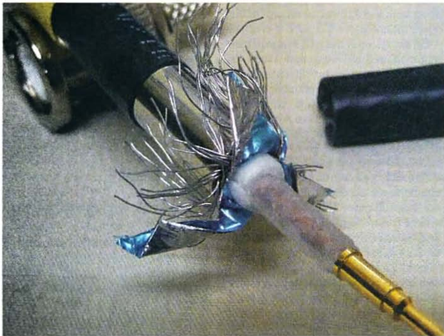
Photo 1: RG6 cable which has insulation on the inner surface of the foil, with the foil twisted to ensure electrical connection.
