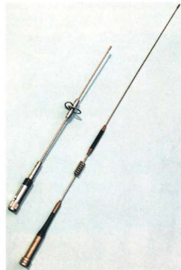
Photo 1: Two commercial dual band antennas.
