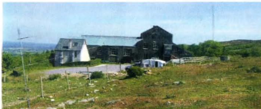
Looking more or less north west showing the vertical and the caravan. The doublet is running parallel with the fence. The vertical is positioned off the end of the doublet and the 'wire' you can see crossing it is the nylon supporting cord.
