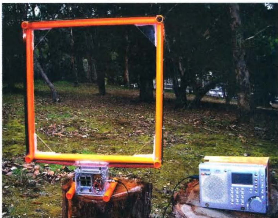
Photo 1: The active loop receiving converter in operation.
