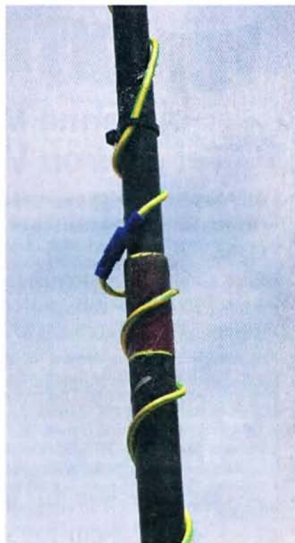
Photo 2: The join in the wire where the rod joins, utilising the bullet connector, allowing the antenna to come apart in two pieces.
