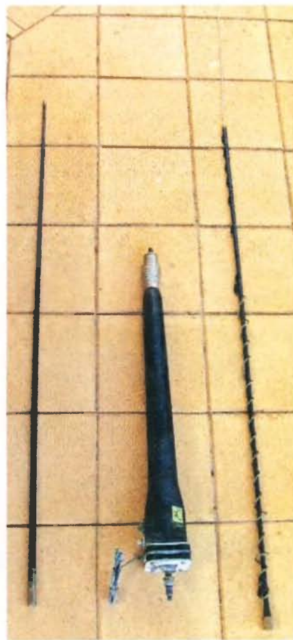
Photo 5: A Codan base unit and its whip lying beside a FAMPARC HF whip to show relative size. Note the earth braid on the Codan base; the pavers are 30 cm square.
