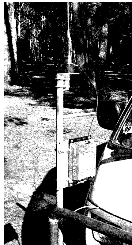
Photo 1: Stainless steel whip with auto tuner and flying lead. This arrangement performed poorly.
