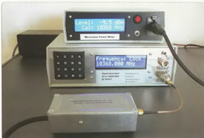
Photo 1: Wideband Power Meter.
