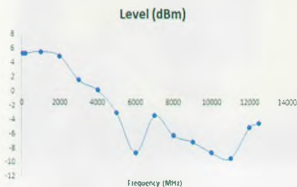
Figure 3: Showing the variation in output level versus frequency for the ADF5355.
