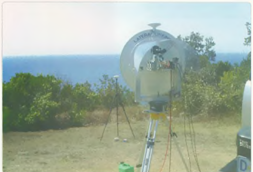
Photo 3: VK7MO/2's portable station (note differential GPS antenna's for bearings).
