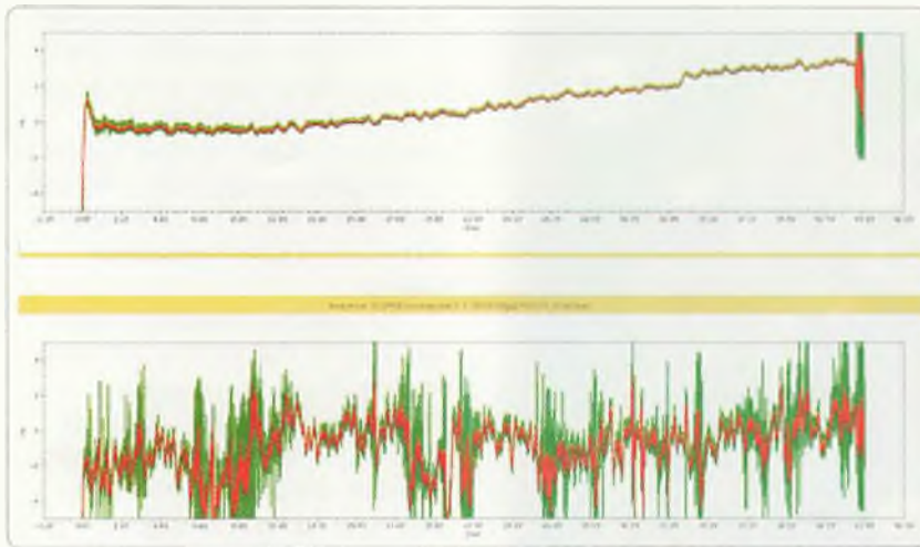
Photo 7: Comparison of spreading between 432 MHz (top graph) and 10 GHz (bottom graph).
