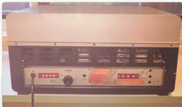
Photo 5: The unexciting rear view shows the external speaker connections adjacent to the power cord, while the antenna connections are at the right.
