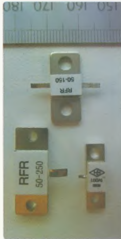
Photo 1: Thin-film, high-power rated resistors suited for making simple dummy loads for rig testing.
