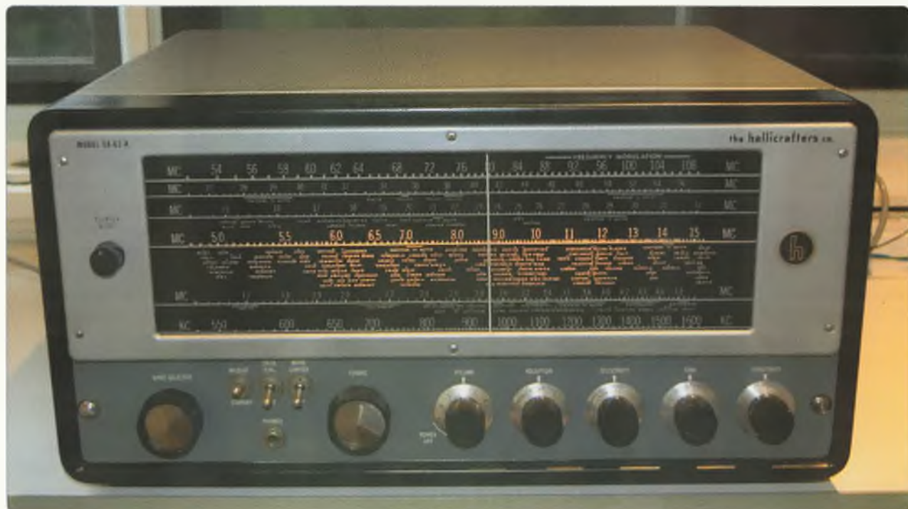
Photo 3: The band you select is lit-up behind the impressive slide-rule dial.
