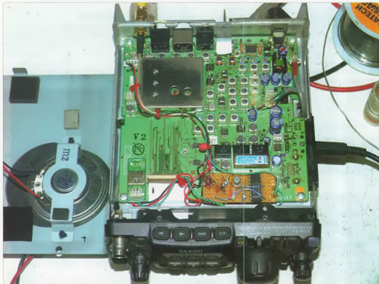
The FT-817 radio with the top cover removed showing the reference switch near the front centre, the original reference on the left, and the coax cable entry on the rear panel.
