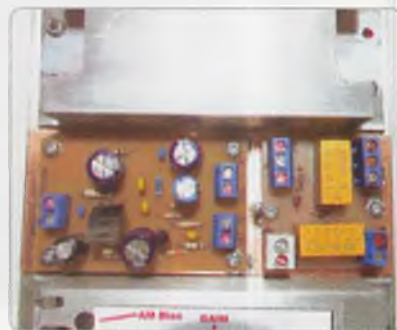
Photo 1L: (From the end of the Second Article) Speaker amplifier and input switching boards before wiring.
