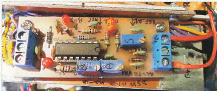
Photo 2J: The ALC and SWR control unit PCB (Figure 26) is small and crowded, but does a big job!
