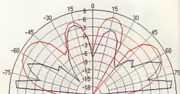
Photos 6 & 7: Models of the antenna design's radiation performance at 7 MHz (left) and 28 MHz (right). The blue trace on each is for the antenna at 12m height, the red trace for lower height.
