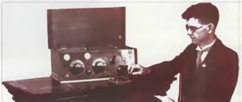
A transceiver powered by a pedal-operated generator was invented by Alfred Traeger in 1927. The technology became central to the success of the Royal Flying Doctor Service and, later, long-distance School of the Air education across the Australian outback.
