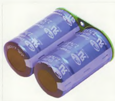
Photo 2 and 3: These two cans, and the board that holds them together, make up a 'super capacitor' of 250 Farads. The board comprises a circuit that balances the charging.
