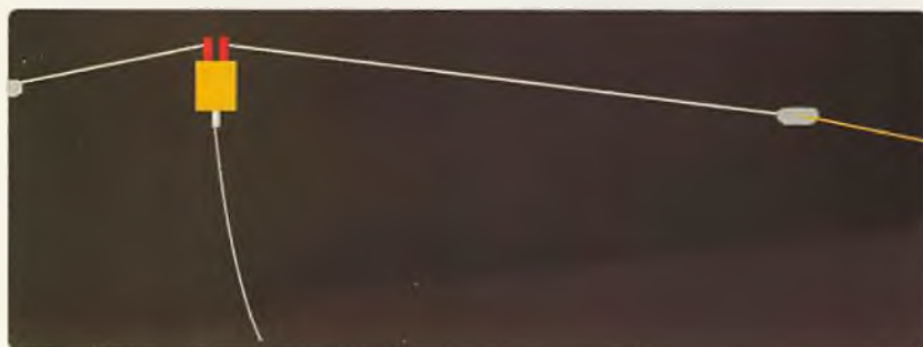
Photo 8: You can mount the feedpoint and balun as high as you can and slope the antenna wires downward. This is good if you don't quite have the space.
