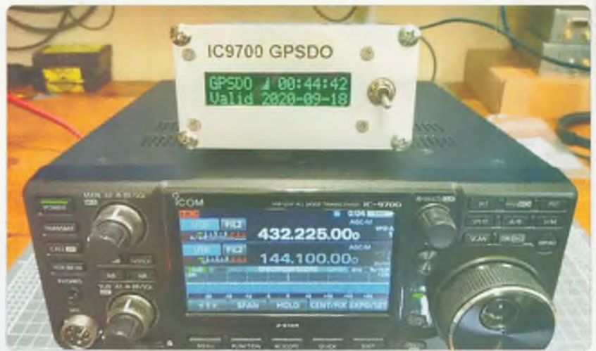
Photo 3: The IC-9700 GPSDO with LCD readout.
