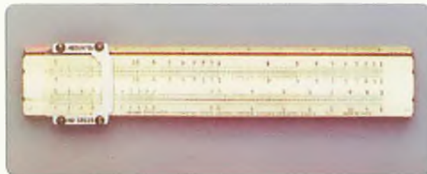
A popular calculator for technical work of yesteryear was the slide rule. This Japanese-made Hemmi slide rule represents a product that was widely used in Australia through the 1940s to 1970s. From the Museum of Applied Arts & Sciences, Sydney. https://collection.maas.museum/object/378620
