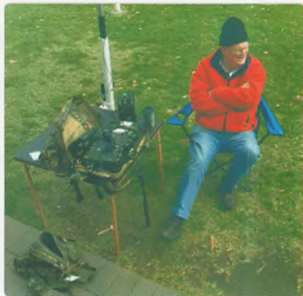
Photo 2: Colin VK2JCC and his Clansman setup, with end-fed antenna using a homebrew 9:1 unun and customised squid pole.
