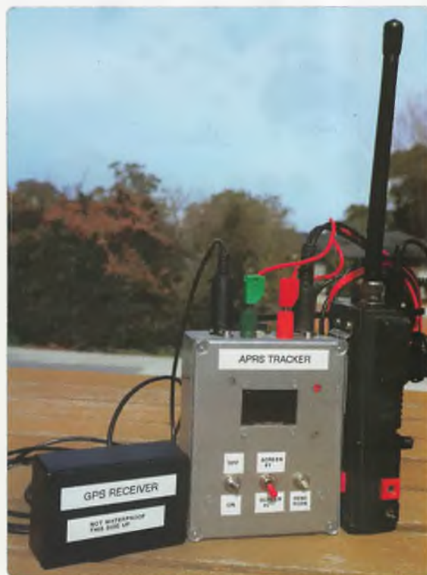
Figure 1: The APRS tracker, GPS receiver and FT-23R transceiver. The GPS receiver module can be positioned to give best reception of the GPS satellites.
