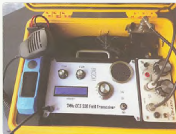
Photo 6: Carmel's homebrew 7 MHz portable QRP transceiver and antenna matcher, housed in a clamshell case.
