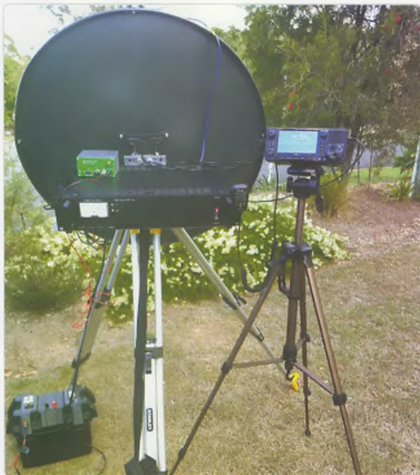
Photo 3: A tangle of tripods! The 705 working as an IF for my 3.4 GHz transverter.
