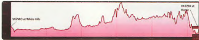
Figure 3: 133 km path with very poor take-off.
