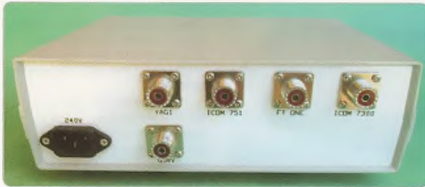
Photo 2: All the antenna and transceiver sockets are mounted to the rear panel, with the "switching magic" happening behind it.
