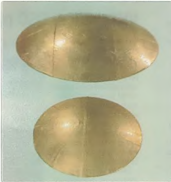
Photo 1: 3D printed Cassegrain reflectors with adhesive copper foil covering.
