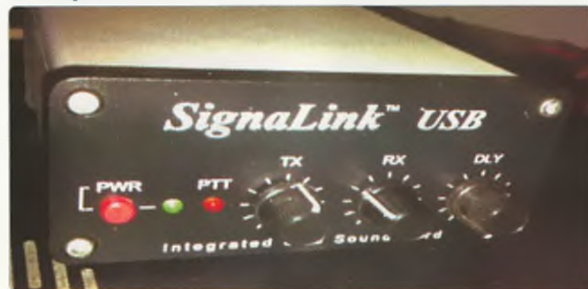
Photo 2: To run digital modes with your older rig, you need an interface unit, such as this Signalink.
