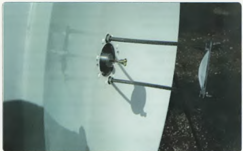
Photo 3: Hand fab 76 GHz conical feed horn with 600 mm NEC dish; very sharp!
