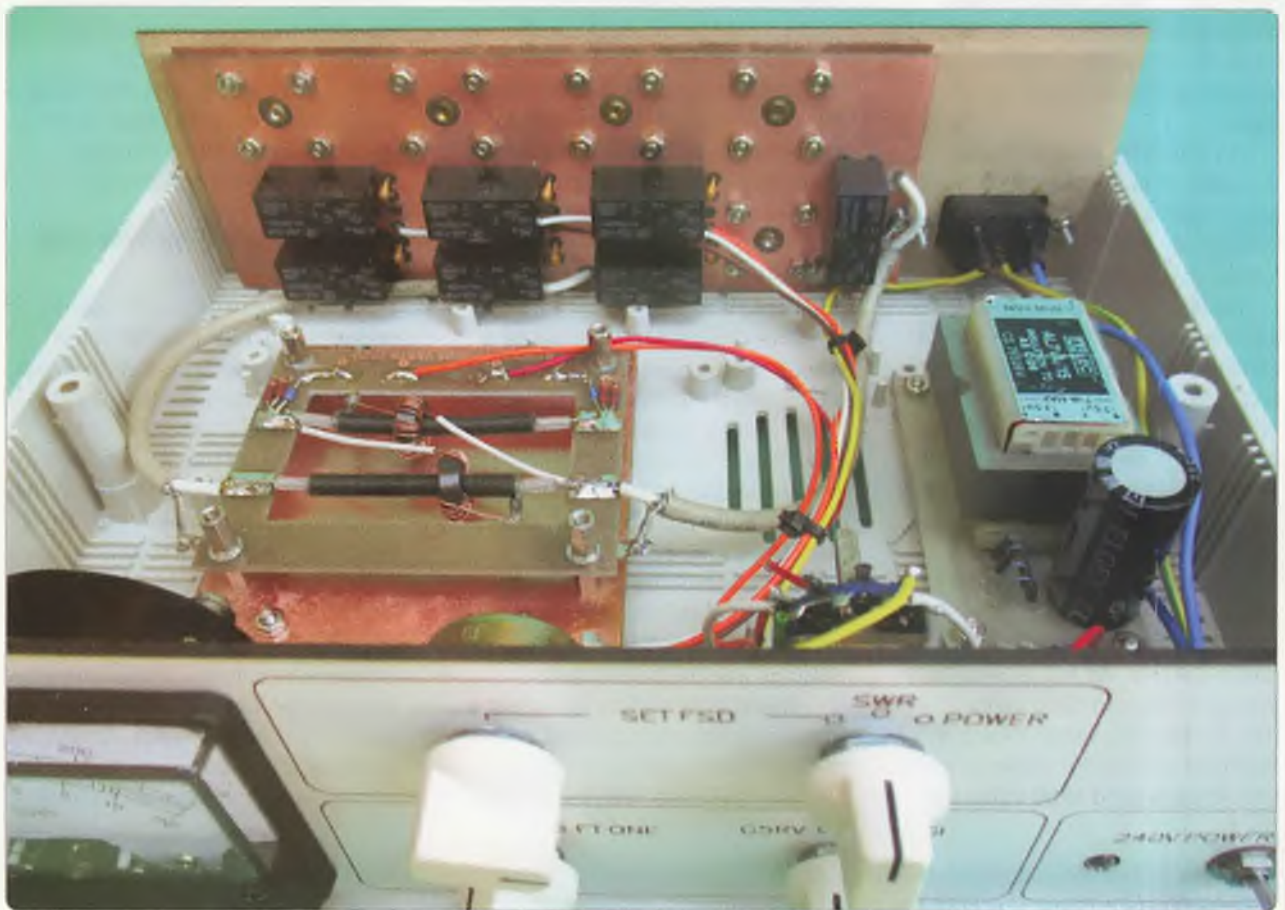
Photo 3: Internal view of the antenna switcher, showing the relay switching board mounted to the rear panel, the Stockton bridge VSWR and RF power meter section at left, mounted to a 'ground plane' of an un-etched PCB. The VSWR/power sensor circuit comprises two ferrite toroids wound with 22 turns of enameled wire and a 'single turn' primary – a length of coax with the shield grounded at one end (only); you can see that each length of coax has the shield grounded at the opposite end to the other. The simple power supply is at right. Although I used a PCB, the circuit is so simple it's not necessary.
