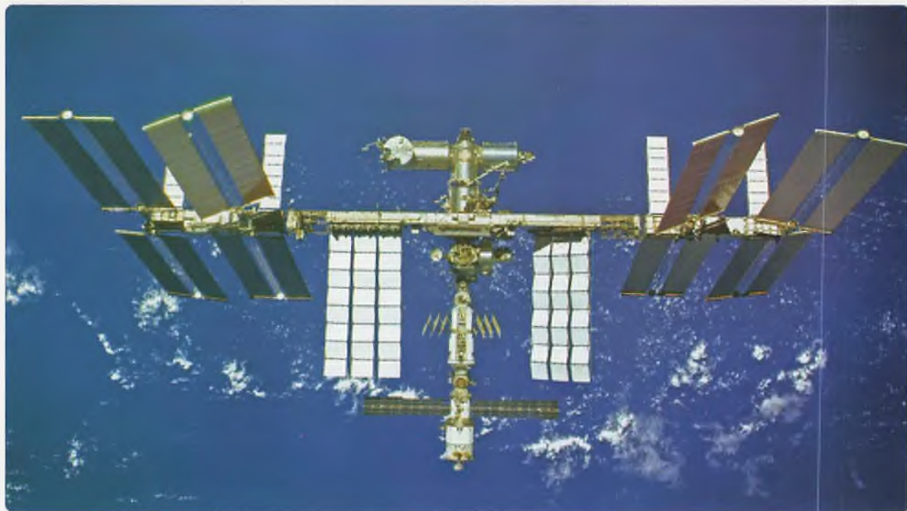
Photo 1: The international space station (ISS), showing its solar panels deployed (European Space Agency photo).
