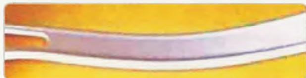
The 300 ohm feedline of yesteryear, widely known as "TV ribbon".
