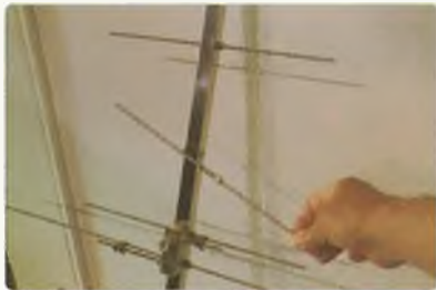
Photo 2: The stainless steel elements are light and strong, with a threaded ferrule that fits a captive nut on the boom.
