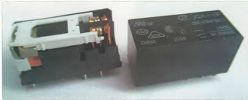
Figure 1: I used these PCB-mounting relays, designed for switching 250 Vac.
