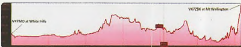
Figure 2: 153 km path from a good take-off at Mt Wellington at VK7ZBX's end, but still well short of line-of-sight when you take account Earth curvature.
