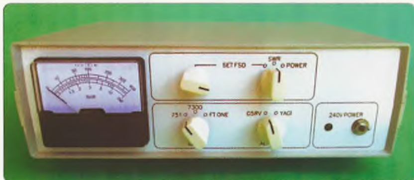
Photo 1: I housed my antenna switch project in an ABS plastic case, 260 x 190 x 80 mm (width, depth, height). I replaced the front and rear panels with 3 mm-thick melamine coated MDF to suit this project. Either operator at this station can select any of three transceivers to connect to either the G5RV multi-band HF antenna, or the Yagi HF beam. Domestic bliss prevails!
