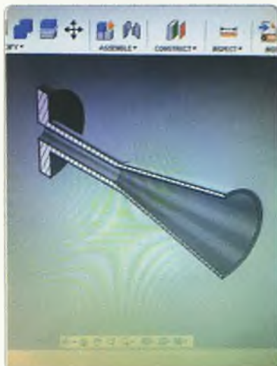
Photo 2: CAD design for a 47 GHz conical feed horn for a Nurad dish.
