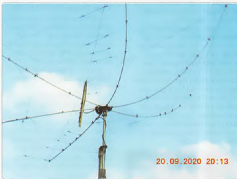
Photo 1: Poor VK6DON's hex beam became an inverted umbrella after the September storm.
