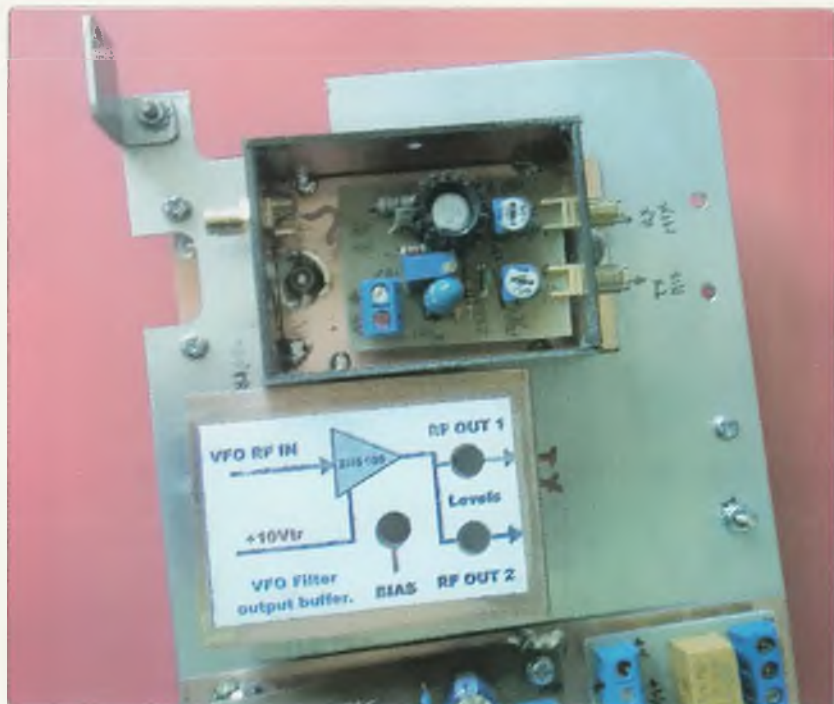
Photo 3GA. The VFO mixer driver amplifier is on a small board housed in a box made of PCB offcuts.
