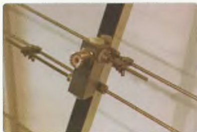
Photo 4: The feedpoints of each Yagi are adjacent to one another; this shows the gamma match assemblies used to set the feedpoint impedance of each antenna. A pity that the SO-239 socket isn't really designed for this sort of application, but it has given no trouble.
