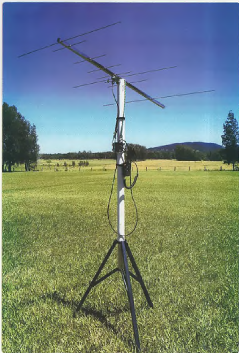
Photo 1: This modest-cost dual-band Yagi comes as a kit that can be assembled and disassembled for portable field use. The white tube is the PVC tube that it came packed in. The tripod is part of an old projector screen stand, obtained from the local tip shop. (I have a few similar tripods which I use to mount small Yagis, dishes or panels on when I go out playing portable radio).
