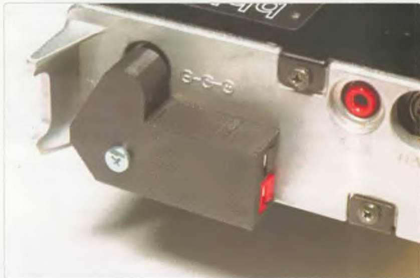
Figure 1: After-market DC connection for the '817 protects the flimsy DC plug/socket and provides more robust Anderson powerpole connectors.
