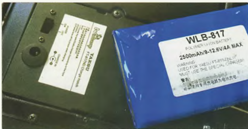
Photo 1: An aftermarket internal battery, such as the WindCamp LiPo battery pack, avoids some failure issues.
