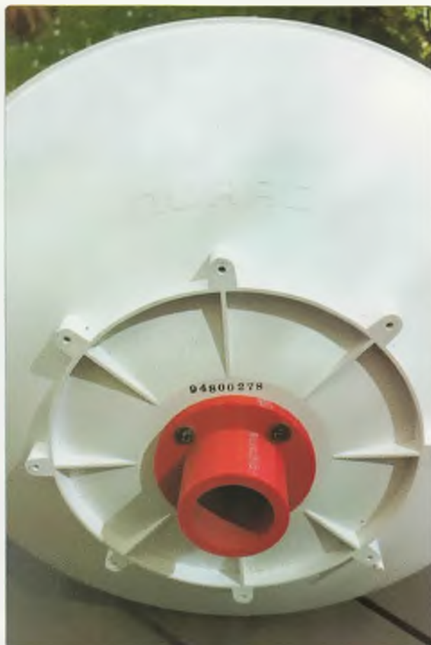
Photo 5: 3D printed 30 mm hub adapter for the Nurad 300mm dish.
