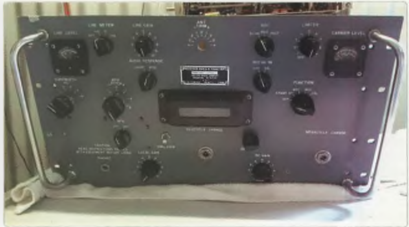
Photo 5: The first act of refurbishment is to remove the receiver's front panel. Most controls and the frequency display window are mounted to the front panel (photo by VK4QS).
