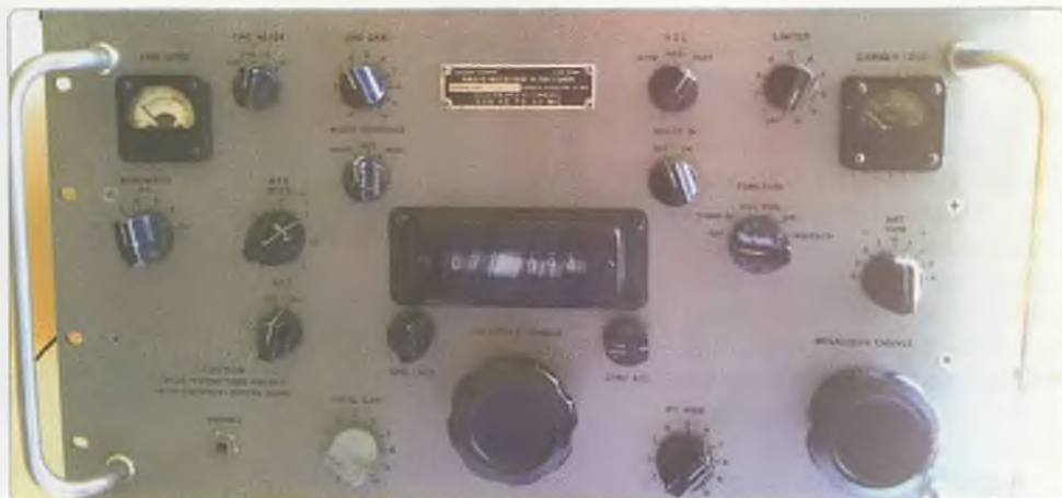
Photo 3: The Collins R-391/URR kept the orthogonal panel layout and frequency display features and included an 8-channel 'auto-tune memory'.
