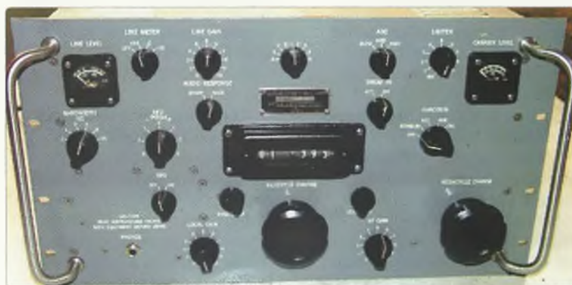
Photo 1: The front panel of the Collins R-390 has a clean, orthogonal layout. Note the mechanical digital frequency display.
