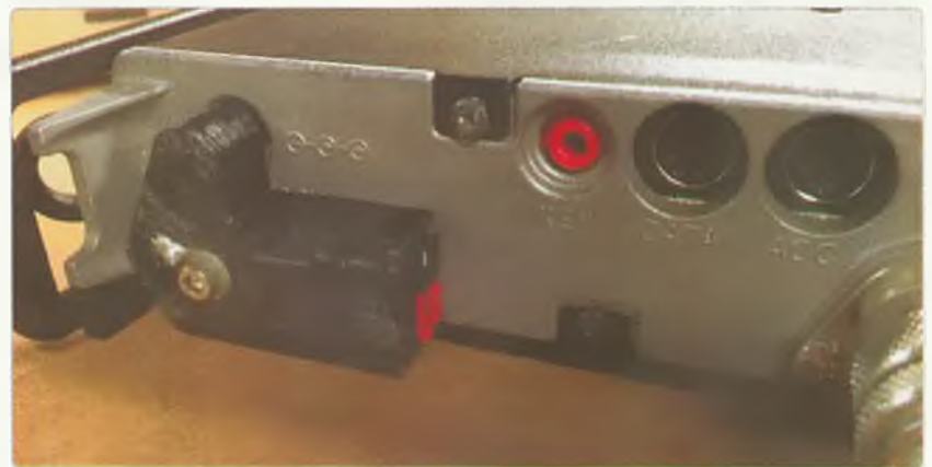
Photo 4: If you use one of the Anderson style adapters, bring a separate negative lead out of the block and ground that to the earth post.
