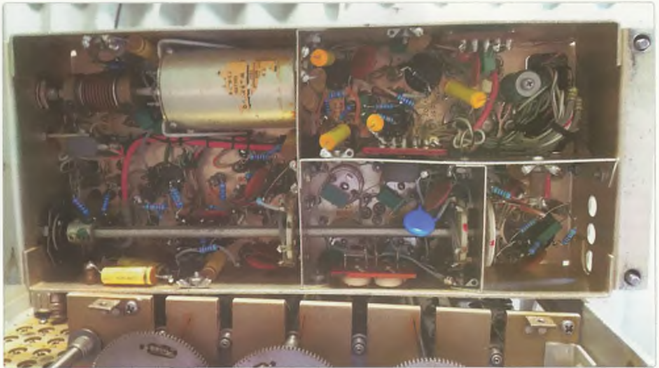
Photo 7: Underside of the IF unit – where the sidecutters hit the component leads! All the new blue resistors you can see are high quality 5% values that I used to replace the old ones (Photo VK4QS).
