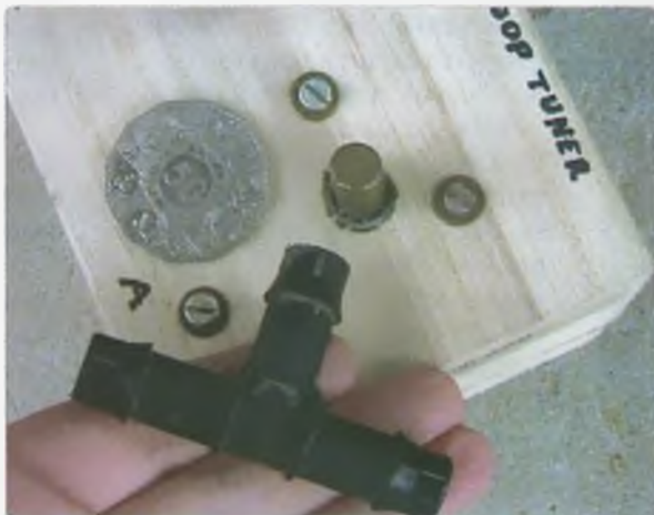
Photo 2: A poly T-piece is a press-fit to a 9.5 mm shaft and provides a convenient, though unconventional, knob.
