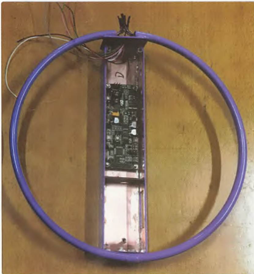
Picture 5: The painted shielded loop antenna fitted to the completed receiver box.
