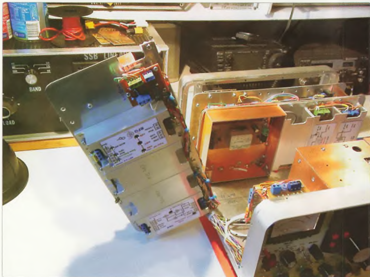
Most of the modules are mounted on both sides of vertical aluminium panels, which swing up and out to give access to the adjustments on each module. The cable looms go to the panels from one side of the case so that the panels remain connected when swung out.
