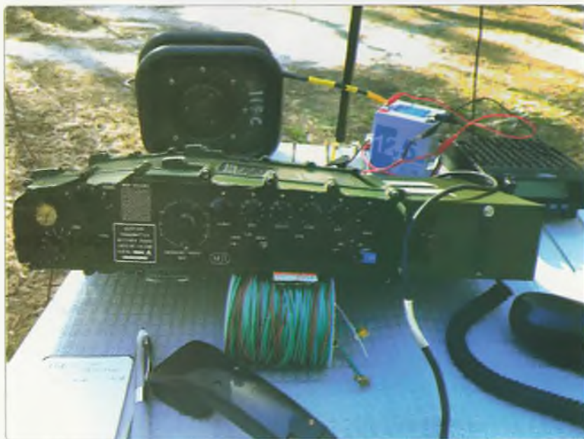
Photo 1: The Clansman PRC 320 military HF radio cover 2-30 MHz and comes with an inbuilt ATU. The telephone-style handset includes a "press" switch in the middle used to transmit.
