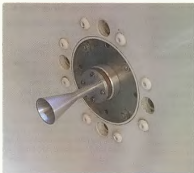
Photo 4: 47 GHz horn feed location for a Cassegrain reflector.
