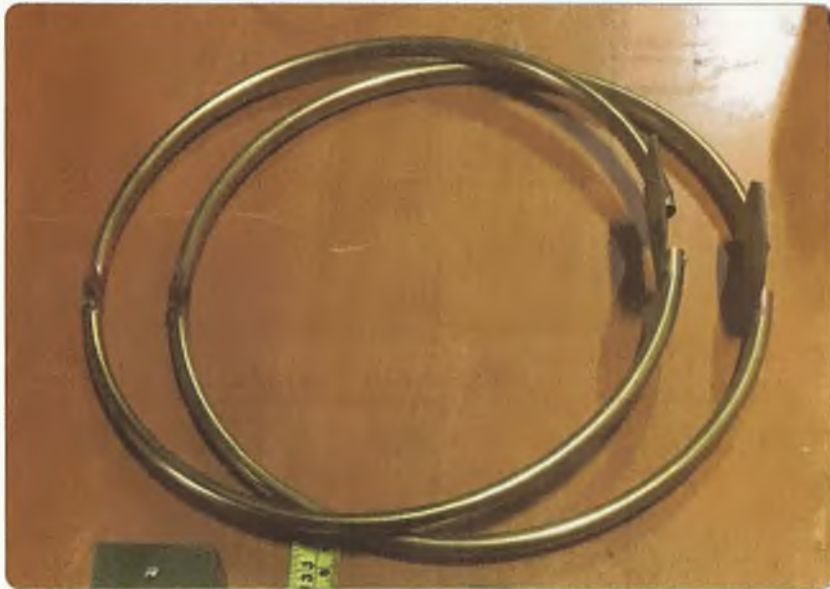
Picture 4: Two of the copper tubes used to make the "shielded loop" antenna.
