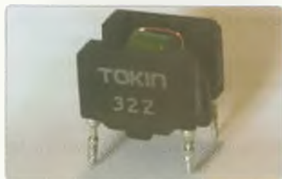
Photo 2: The DC supply line common-mode filter, T1035 (Figure 2), is wound on this miniature ferrite core.
