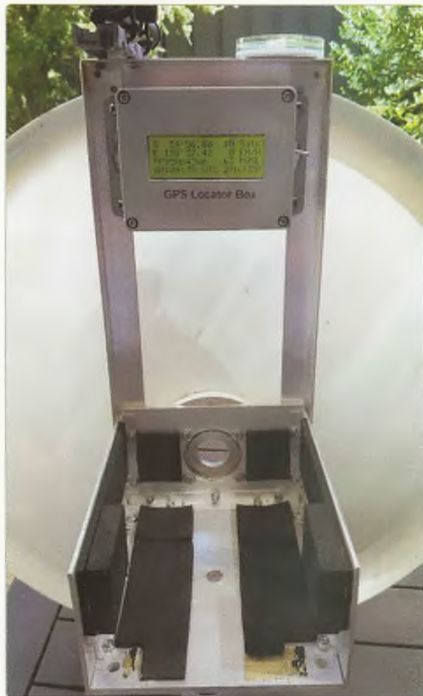
Photo 3: NEC 600 mm mmWave quick-change transverter mount with 30 mm hub
