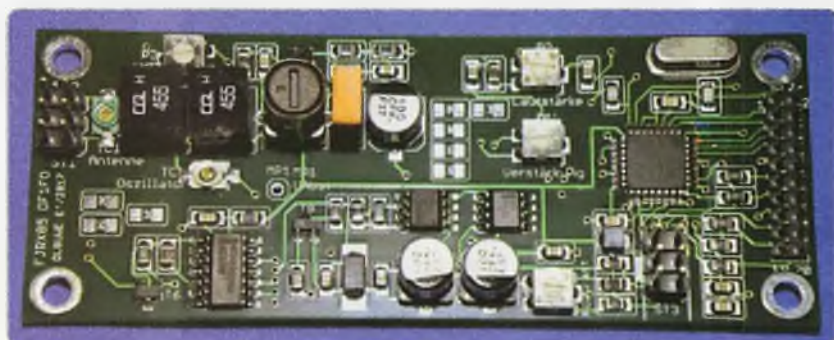
Picture 3: Top side of the DF1FO receiver board. Note the microcontroller at the right.
