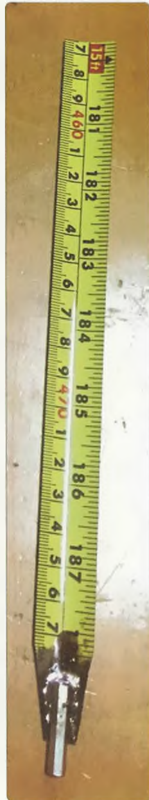
Picture 6: The sense antenna, made from a short length of old broken tape measure with an M3 Hex standoff soldered to it.
