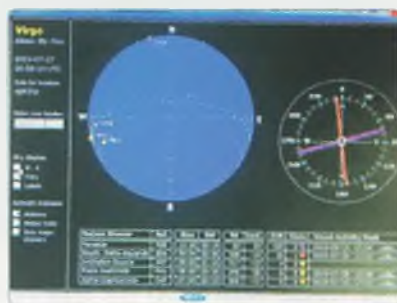
Photo 2: Typical Virgo Skymap image showing the relative position and track of the Perseids (PER) Meteor Shower in PURPLE at the north of the screen (on the left) and the corresponding optimum antenna orientation (radio path) also in purple on the compass rose (on the right) - which is almost East-West. Also shown is the position of the Southern Delta Aquarids (SDA) Shower in red, almost due West at the same time. This shower supports North-South paths from the author's location in grid square OG64.
