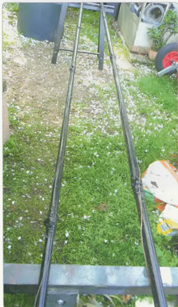
Photo 2: Winding of both parasitic elements placed on sawhorses.
