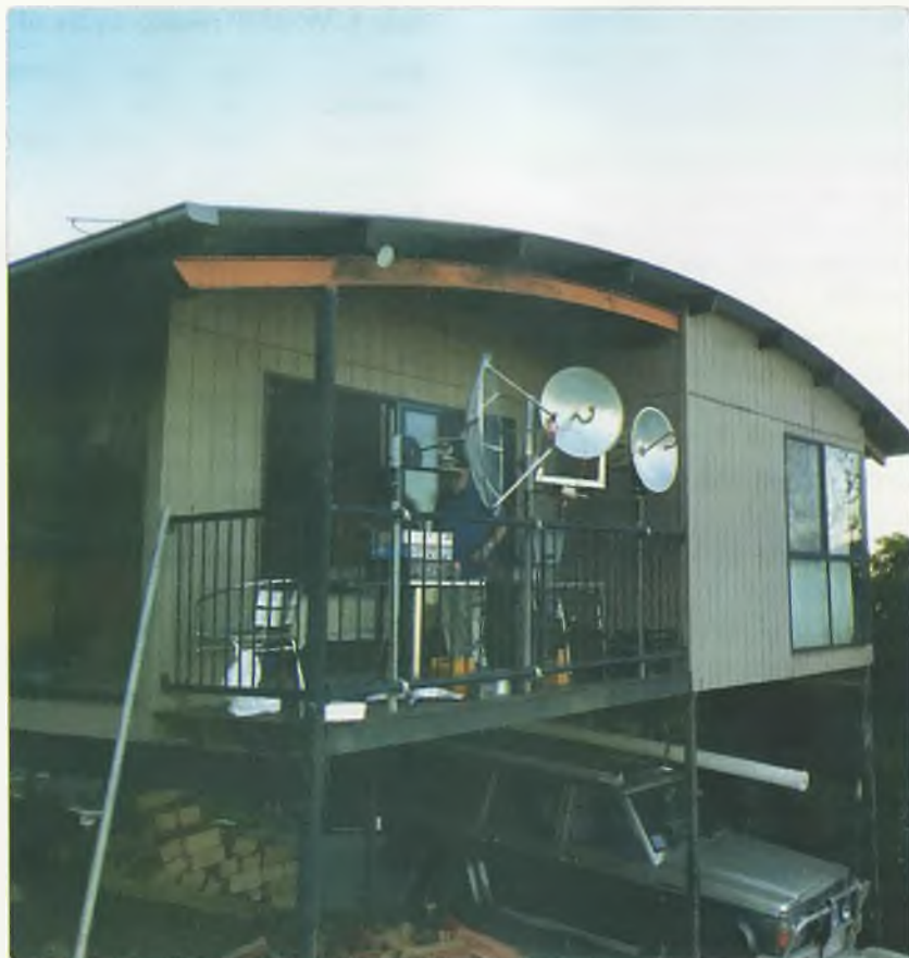
Photo 5: Operating position for the microwave bands from 2.4 GHz through 24 GHz, showing the three dishes which were able to cover from west through to the southeast.
