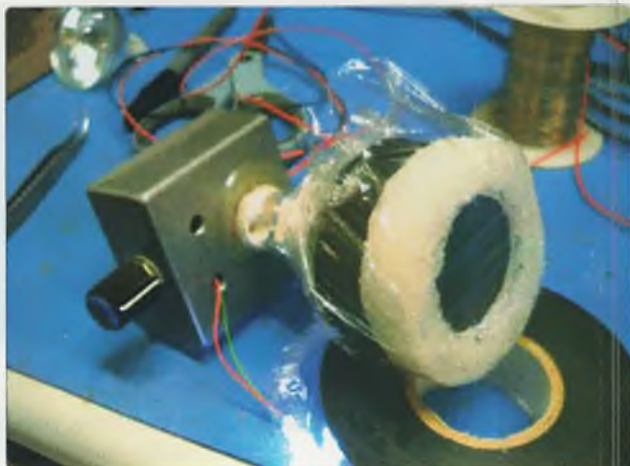
Photo 4: VK3CV's experimental 30 THz sensor (receiver).
