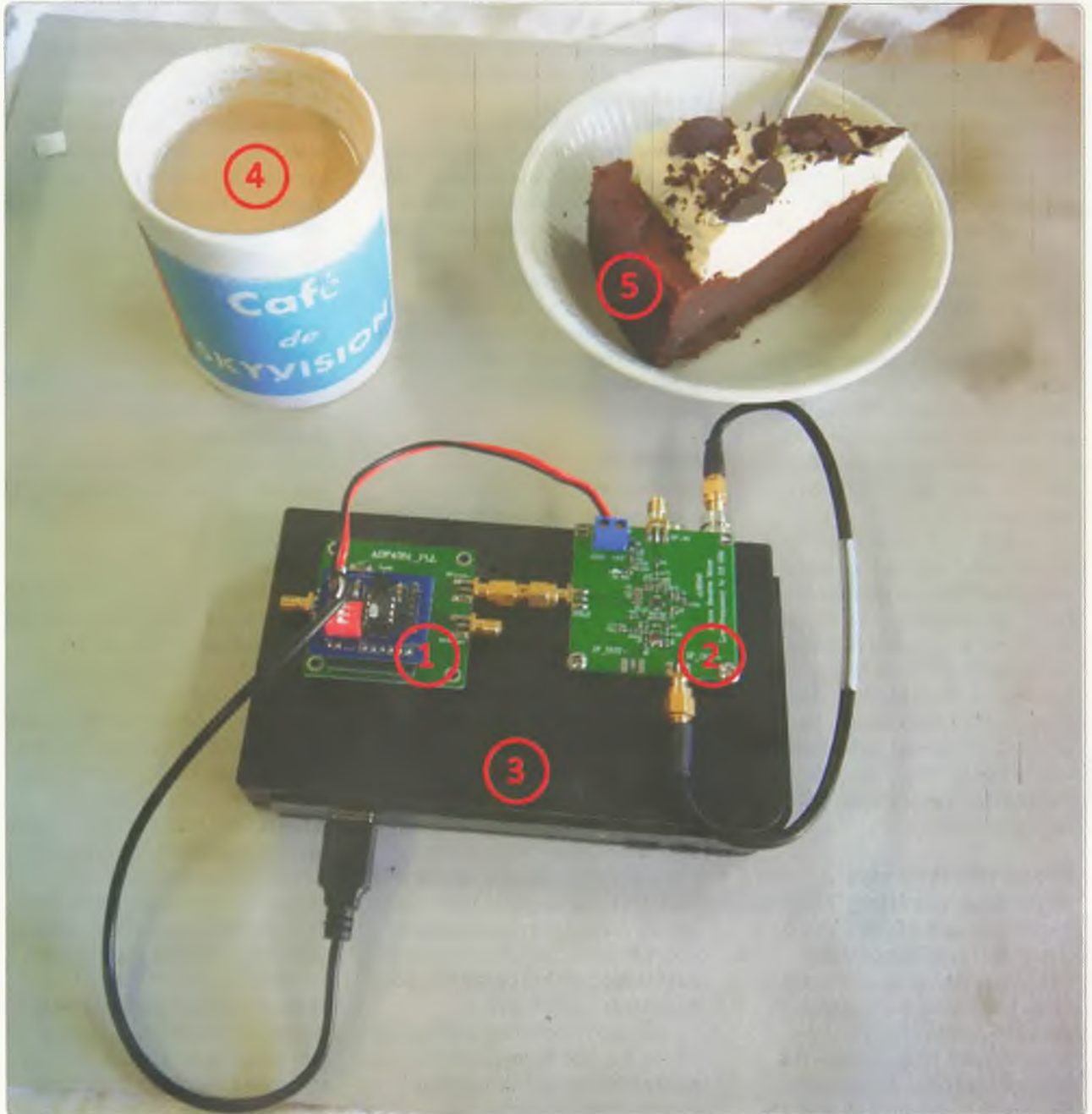
Figure 5: Another modular approach. 1 - Local Oscillator. 2 - Active mixer down converter. 3 - Strong DVB-T set-top box. 4 - Celebratory coffee. 5 - TV watching comfort food.
