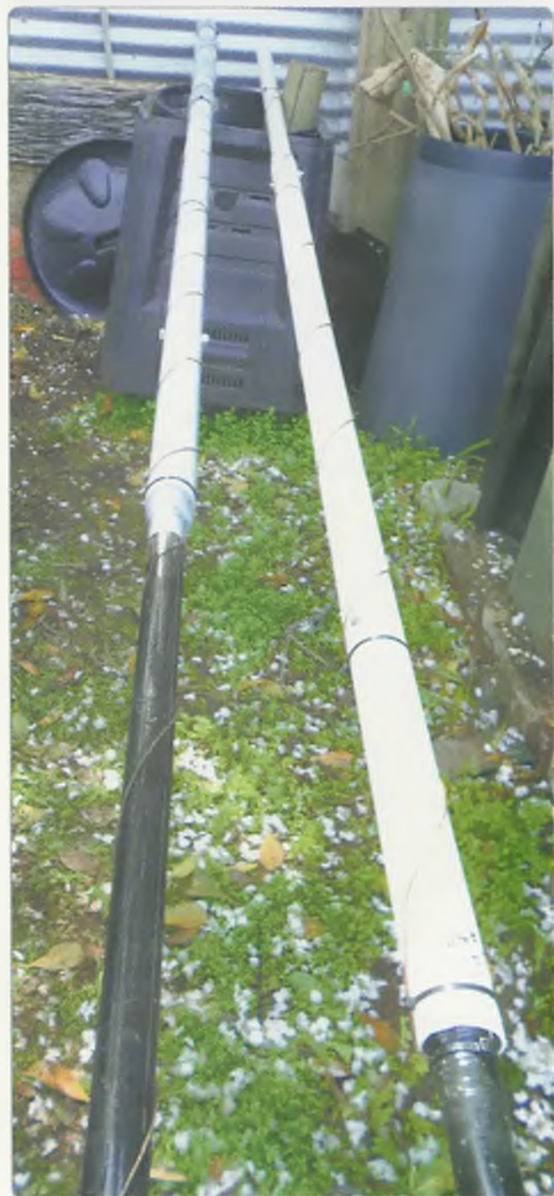
Photo 3: PVC pipe element extensions prior to painting.
