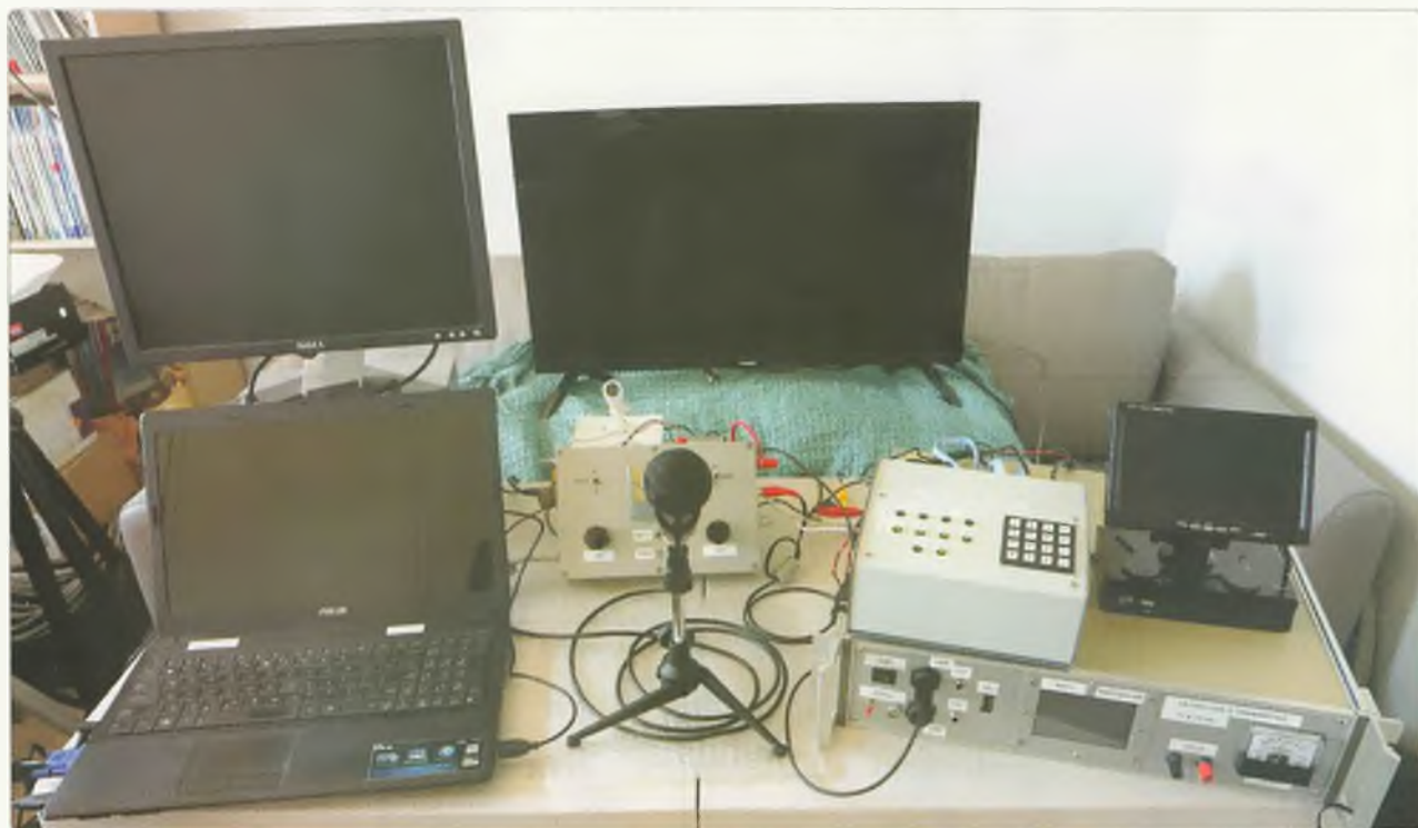
Figure 2: The VK1DSH DATV station, with the Portsdown transmitter, video switch, DVB-S set-top box and preview display on the right-hand side, then the MiniTiuner PC and second PC VGA display on the left-hand side. The centre contains a small TV camera, audio mixer and microphone. The preview monitor is a 7-inch truck-reversing monitor, which has analogue video inputs.
