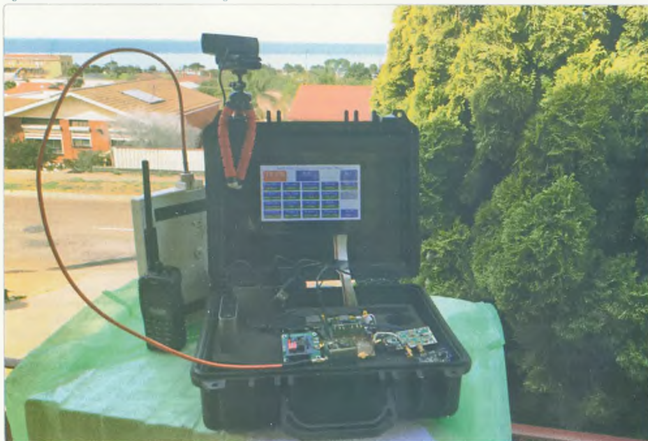
Figure 3: The ultra-QRP Portsdownunder rig.
