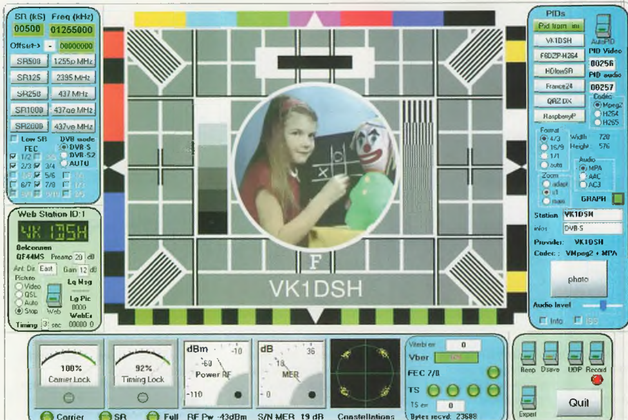
Figure 6: The MiniToune software display on a PC screen. The test pattern is generated by the Portsdown software.
