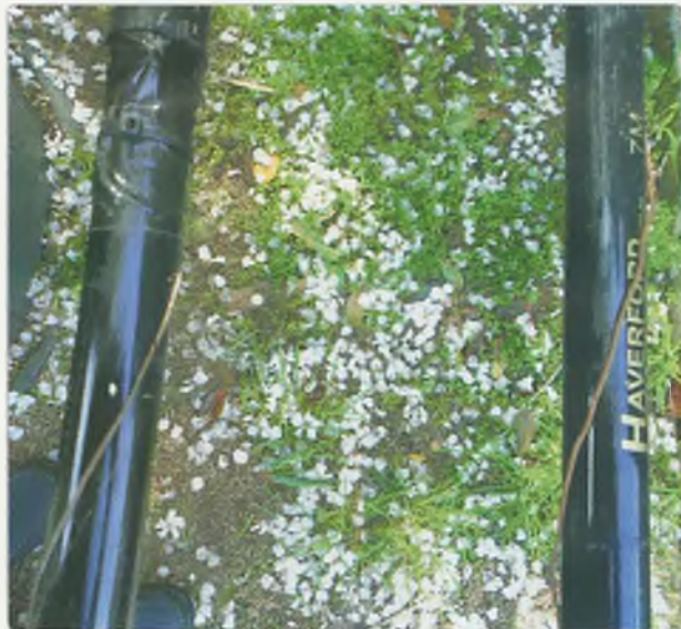
Photo 4: Close-up of two parasitic elements, showing the windings and Gaffer tape wrap with zip-tie.
