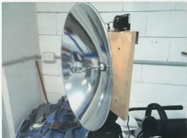
Photo 3: Andrew VK3CV's experimental 30 THz transmitter.
