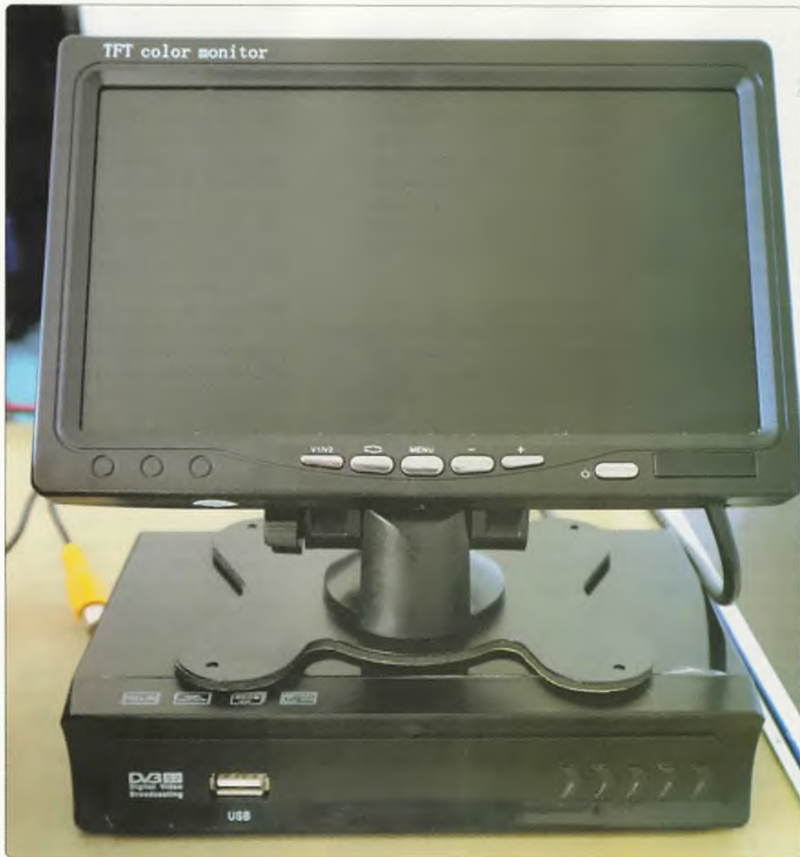
Figure 8: A small satellite set-top box and TV monitor. The total cost was about $60. The receiver operates from 12 Vdc and appears to be designed for use in caravans and motor vehicles, but is limited to reception of standard DVB-S signals, rather than amateur reduced-bandwidth signals.
