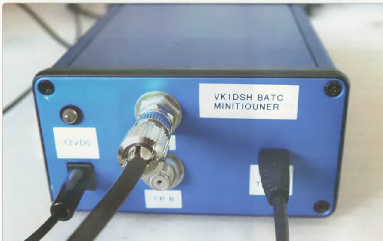
Figure 5: The MiniTiuner receiver module. The receiver has two separate RF inputs and connects to the host PC through a USB connection.
