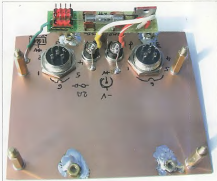
Photo D3: Rear panel with power supply components.
