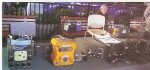
Hallicrafters S-39, Gibson Girl, R210 receiver, and C42 VHF transceiver (Left to Right).
