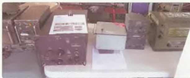
ARR-15 HF receiver (left) and ARC-114 and ARC-115 VHF transceivers (right)
