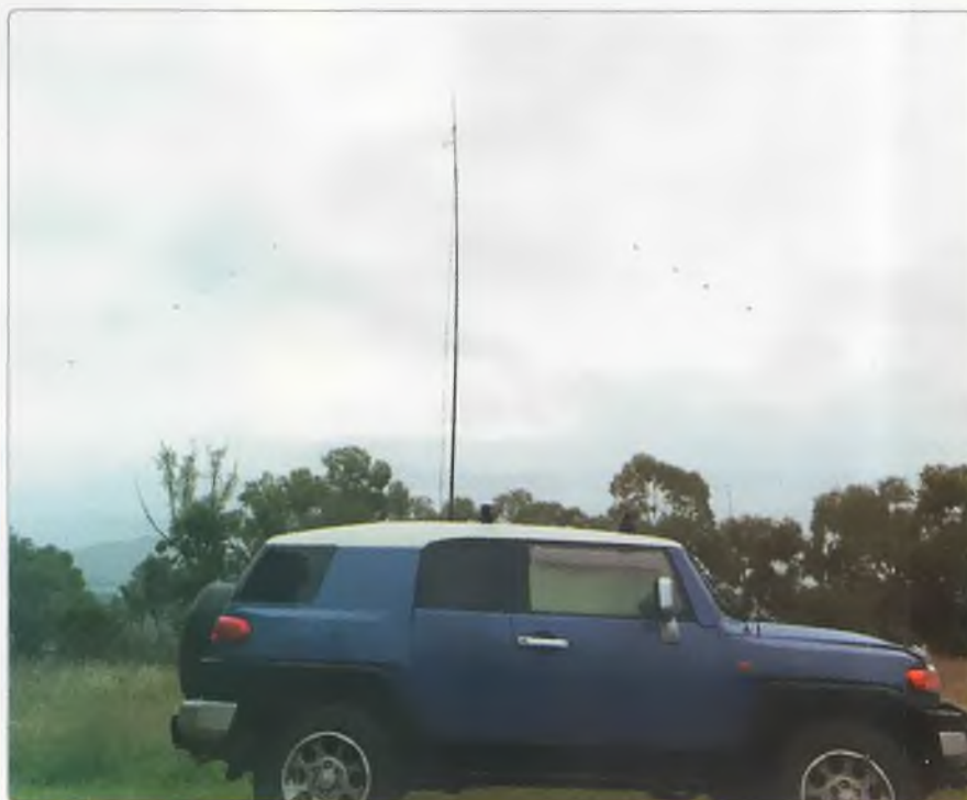
The VK1WIA multi-band inverted-vee dipole antenna. Photo: VK1DA.
