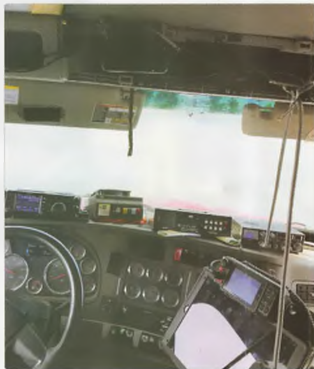
Photo 1: Interior of KK6OKI's cab with amateur radio and commercial communications gear.
