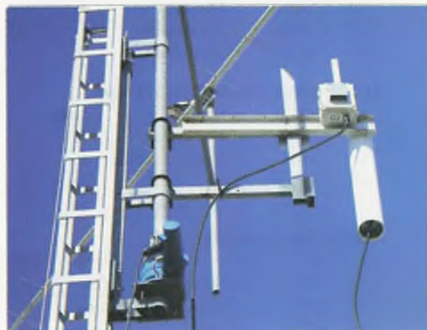
Close-up photo of the 24 GHz PA and slot antenna.
