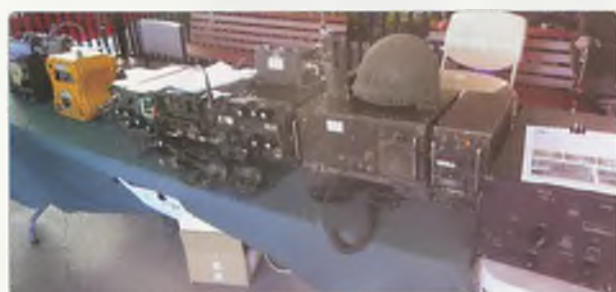
RT-524 and R-442 American VHF radios. Also PRT-4 and PRR-9 squad radio (on top)
