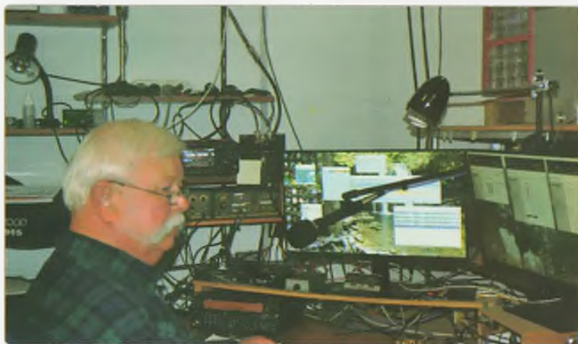
The home setup for operating my remote station. The right-hand screen controls antenna switching, rotator and linear. The left screen is the logging program. Just visible is a TS590 that links to another slave TS590 at a remote site.
