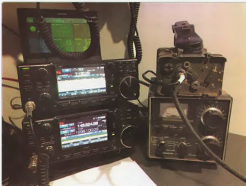
Photo 1. Bob VK2ADF used this WWII CPRC-26 VHF rig. It's crystal controlled, operates over 47 to 55 MHz, and runs 300 mW. Bob used a Buddipole antenna.
