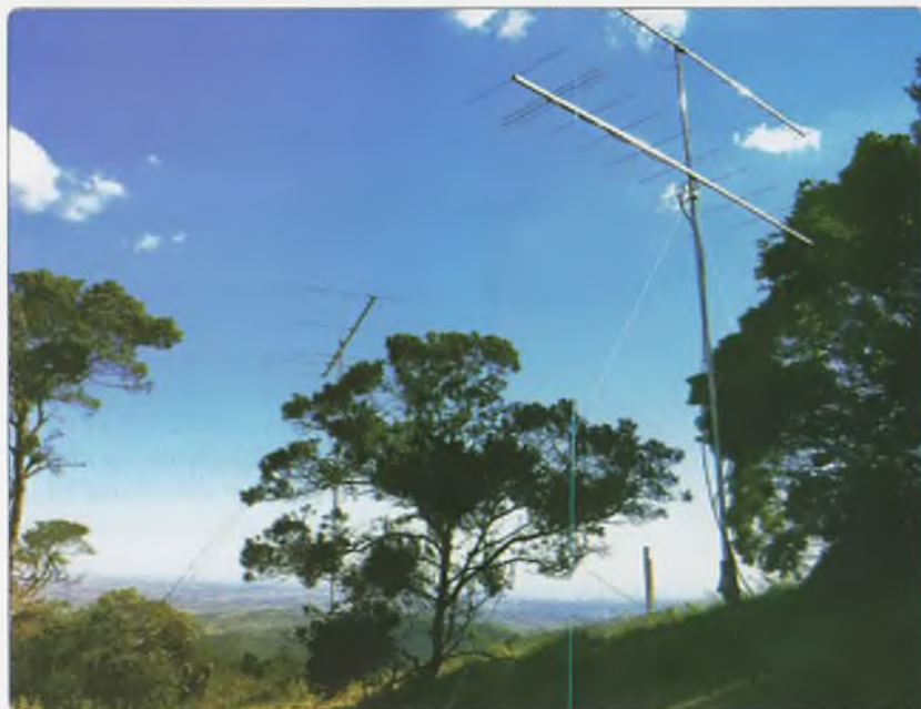
The VK4IF/p Yagi arrays deployed for their winning onslaught on the 2020 Spring VHF-UHF Field Day. On the left is the 6-m Yagi on its own mast, with 2-m and 70-cm Yagis on the other mast at the right.
