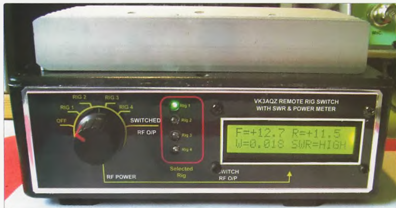
Photo 2A1. A view of the completed Rig Switch.
