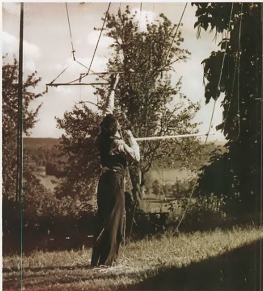
Photo 2: Hull's 56 MHz directional antenna of wire and wood was used in his seminal work on demonstrating tropospheric refraction propagation.
