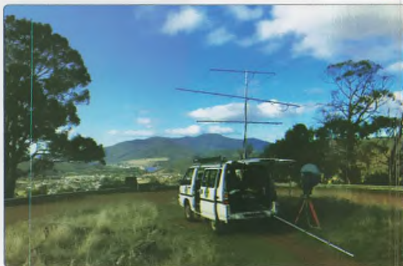
Justin VK7TW deployed his four-band single-operator setup for the 2021 Winter field day, using Yagis for 50 MHz, 144 MHz and 432 MHz, and a dish on 1296 MHz. The site is Peppermint Hill in Hobart, Tasmania.
