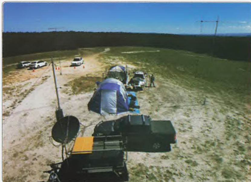
Multi-operator station VL3L (Ralph VK3LL) at Enfield, Victoria, deployed on a site once the location of a VHF Omnidirectional Radio Range (VOR) aircraft navigation system. Note the array of Yagis on masts scattered across the site for bands from 50 MHz through 1296 MHz, and an offset-fed dish in the foreground with a three-band feed for microwave bands.
