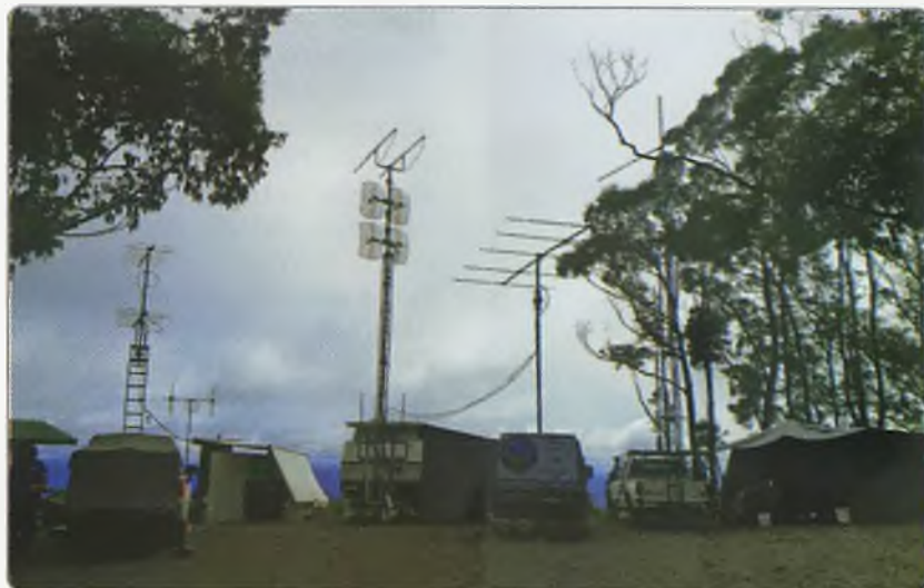
The VK2SRC/p club station deployed at Vista Point in northern NSW for the 2021 Spring VHF-UHF Field Day, operating on all bands from 50 MHz through 3.4 GHz. Note the use of both horizontal and vertically polarised arrays. Horizontal polarisation is the predominant standard for weak-signal working on the lower end of the bands, while vertical polarisation is used on the upper end of the bands for FM/CFM/DMR modes.
